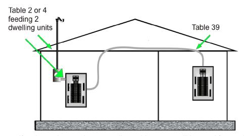
If main service requires upgrading, tables 2 or 4 will be used for service conductors.
