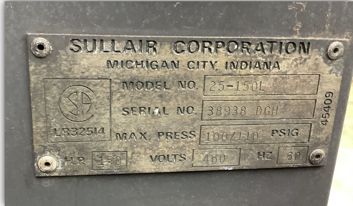
Image 2 - Air compressor manufacturer nameplate and approval certification mark.
