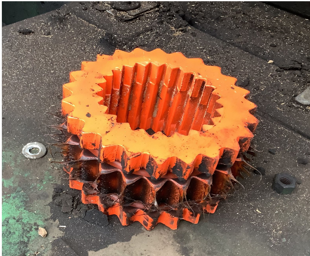
Image 3 - Polymer coupling: couples the prime mover and air compressor.
