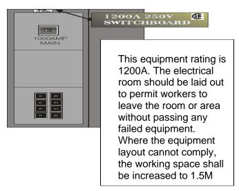
The equipment has a 1000A main breaker, but the 1200A nameplate shall determine the electrical room layout and clearance requirements. An acceptable layout in compliance with sub-rule (2) should be the priority and only when it is not possible should the working space be increased to 1.5M.
