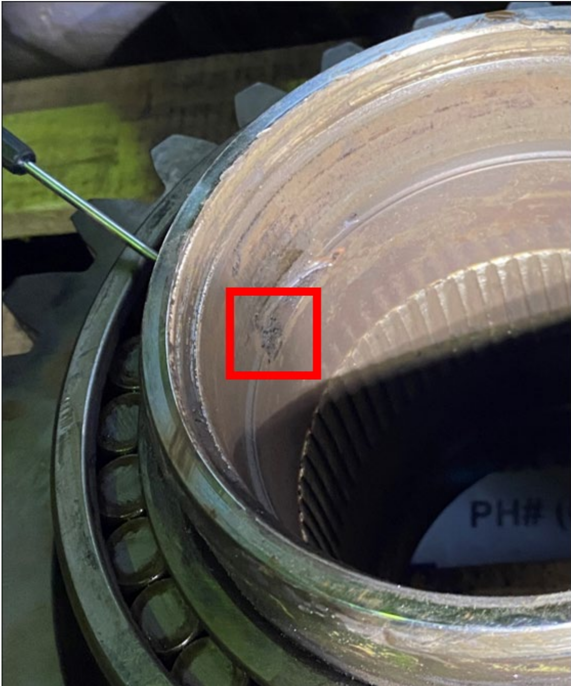
Image 14 – Step-drive main-shaft drive gear, red box showing location of plugged oil passage.
