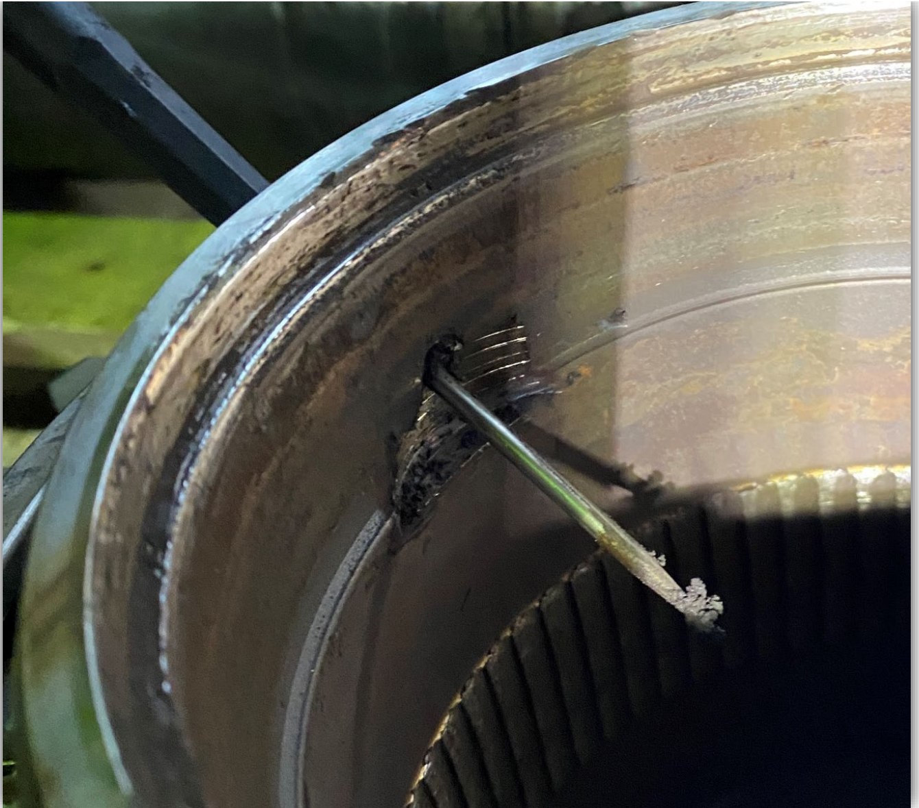
Image 15 - Oil passage unblocked with small screwdriver.
