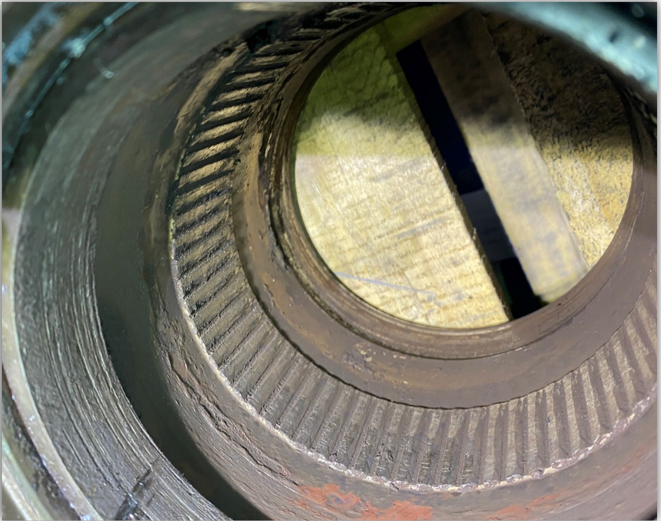
Image 12 – Step-drive main-shaft drive gear showing damaged internal splines.
