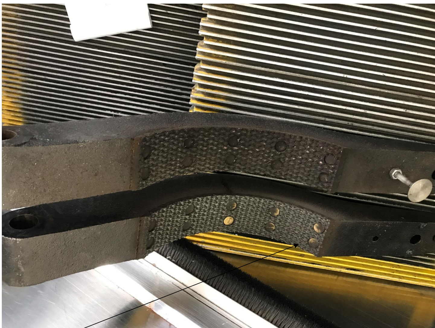
Brake linings unevenly worn. Brake linings worn down to lining retaining rivets.
