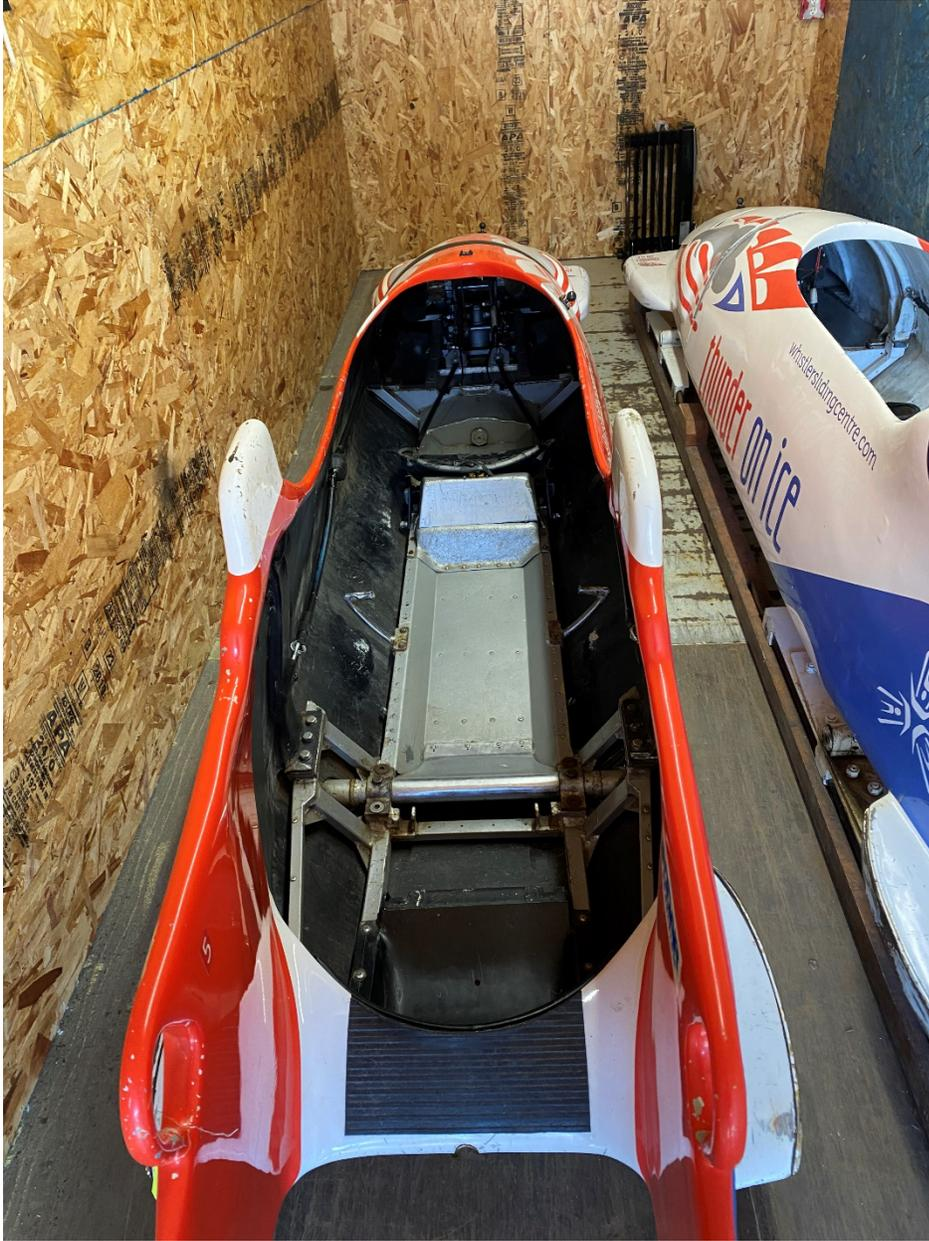
Figure 4 - Internal components including pilot's seat, foot pegs and hand cables for the public passenger bobsleigh.
