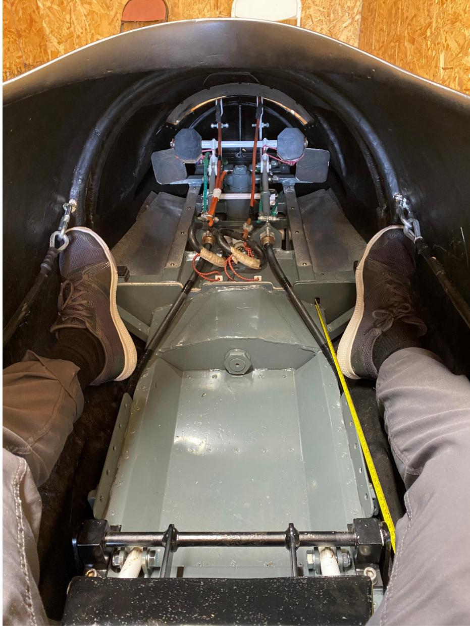
*Figure 9 - View of Pilot's controls from passenger seat 2. Note the foot rest position on the bobsleigh frame.*
