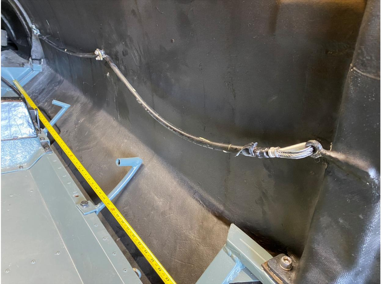
*Figure 6 - Close up view of the cable handholds for the passengers.*
