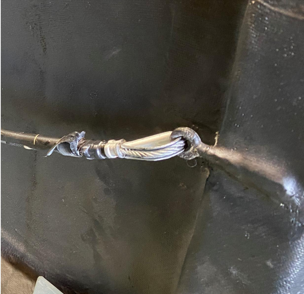
*Figure 7 - Cable thimble at the end of the handhold that requires the passenger in seat 4 to reach further forward for a comfortable grip*
