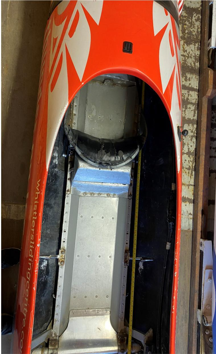
*Figure 5 Overhead view of the pilots seat area and seats 2 and 3 (padding removed). Note the reclined angle of the backrest for the pilot's seat.*
