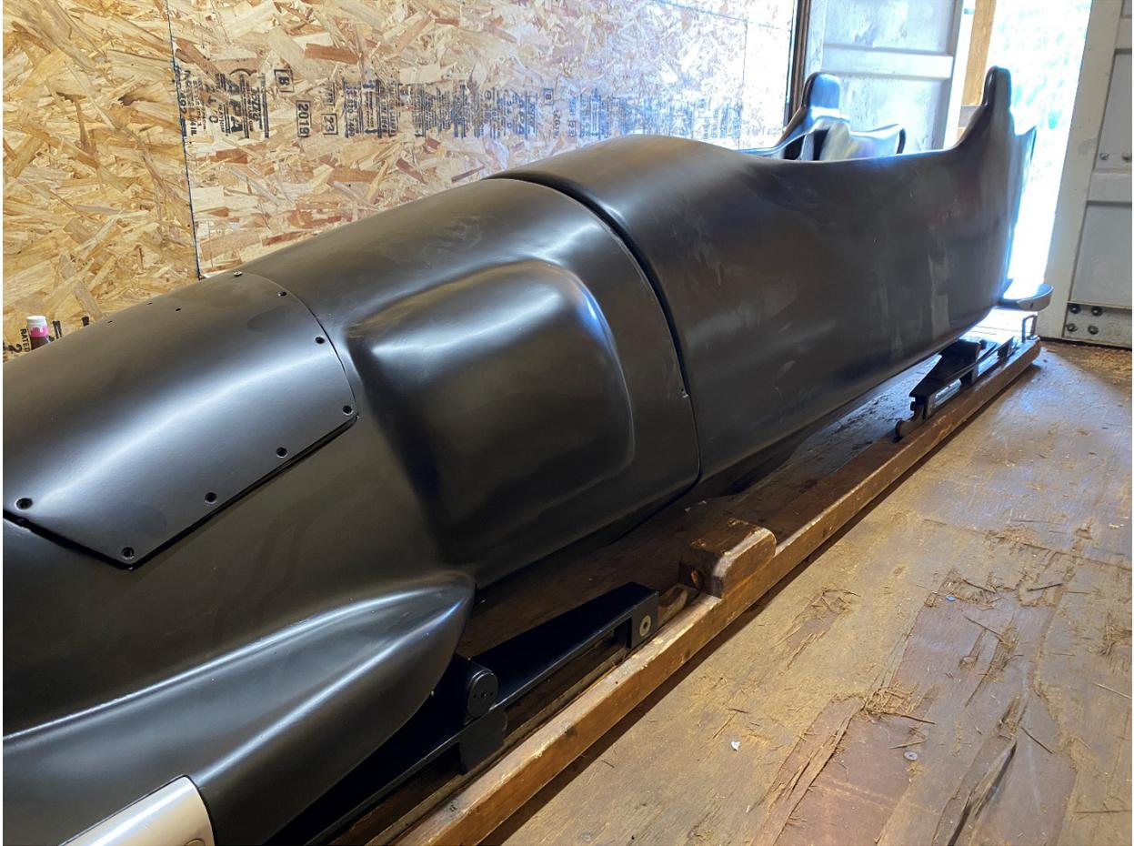
Figure 2 - Front view of the public passenger bobsleigh. Note the higher sides at the rear of the bobsleigh.
