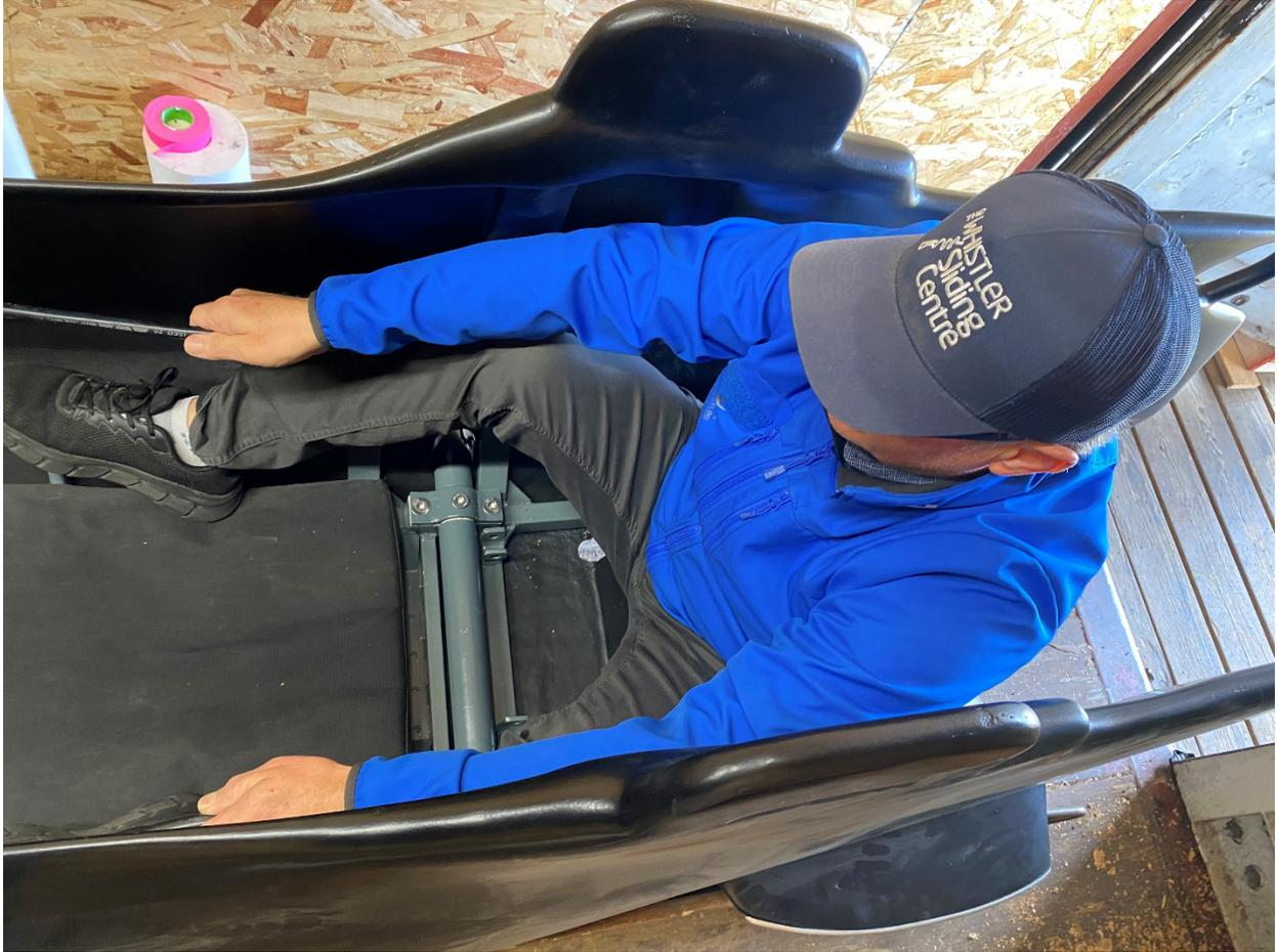
*Figure 16 - Foot position on the foot peg is altered resulting in the knees interfering with the ability to reach the handholds.*
