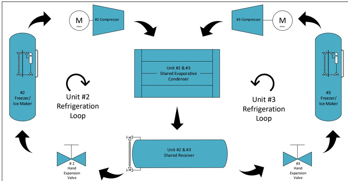
Figure 3: Basic flow diagram of P24 refrigeration cycle
