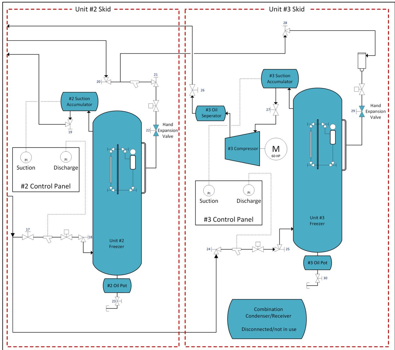
Figure 8: P24 Freezers Piping Configuration Pre- Incident (Unit #2 left and Unit #3 right)
