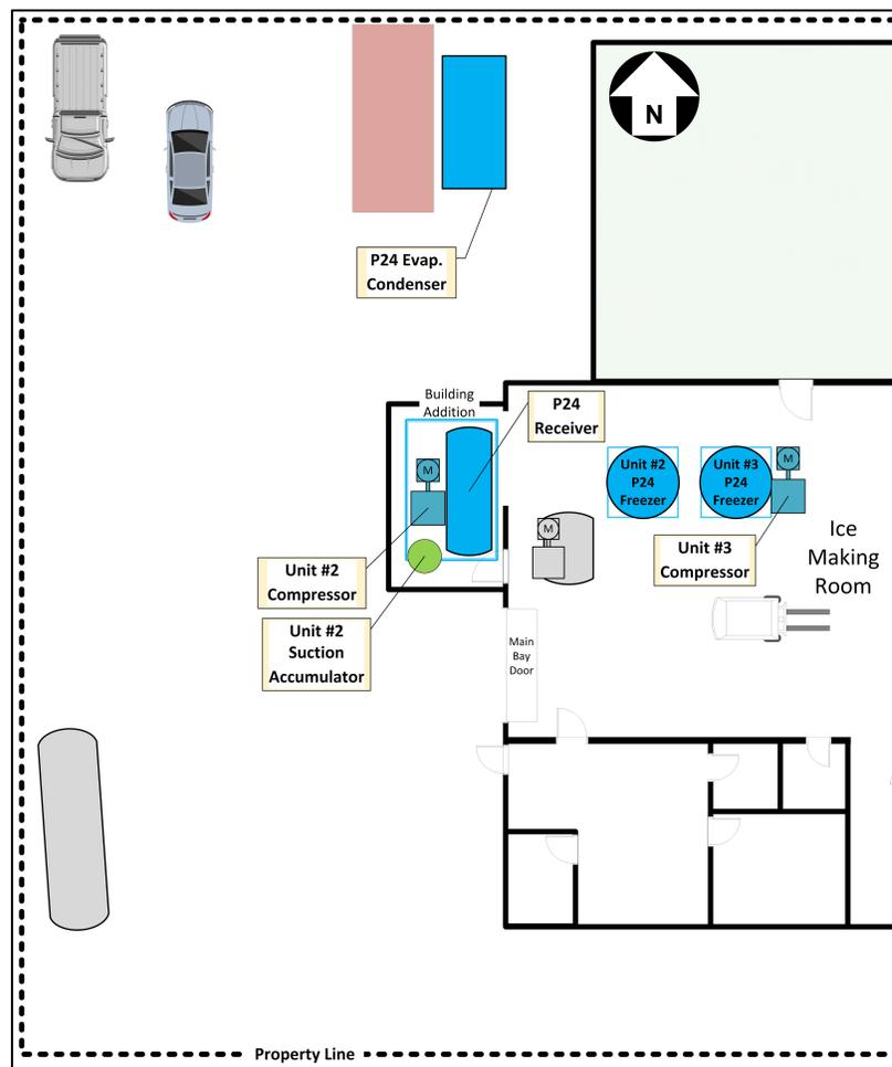
Figure 10: P24 System Components As-Found Post Incident
