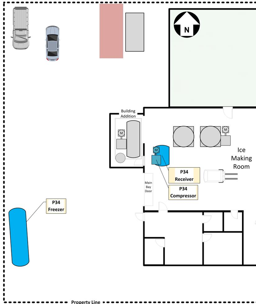
Figure 5: P34 System As-Found Post Incident
