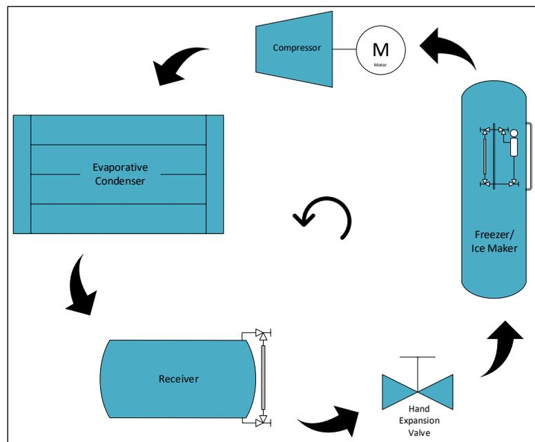
Figure 2: Basic flow diagram of P34 refrigeration cycle
