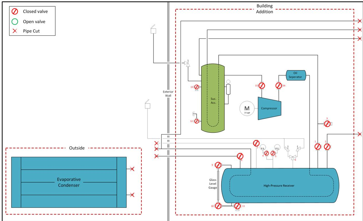
Figure 12: P24 Building Addition As-Found Piping Configuration and Outdoor Evaporative Condenser
