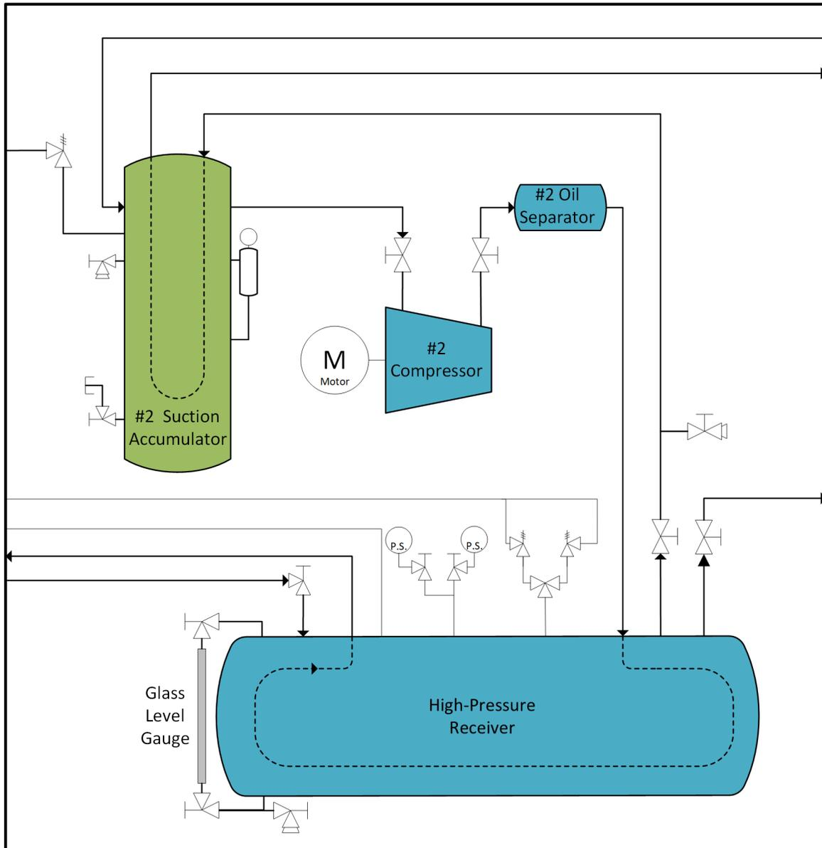
Figure 9: P24 Building Addition Piping Configuration Pre- Incident
