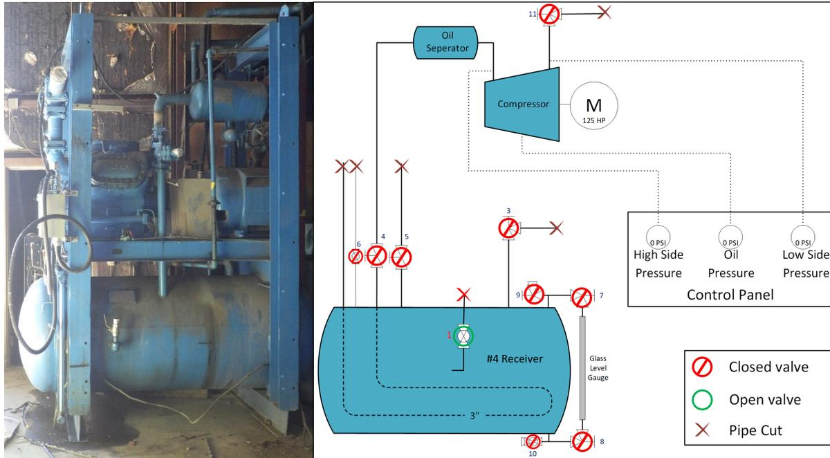
Figure 6: P34 Receiver as Found (Left) and Piping Configuration (Right) Post Incident (See Table 1: P34 Valve Index in Appendix B.1: Process flow diagrams and valve index for valve information)
