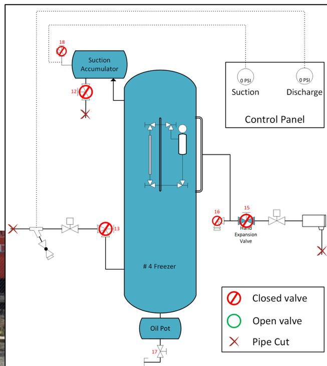
Figure 7: P34 Freezer as Found (Left) and Piping Configuration (Right) Post Incident
