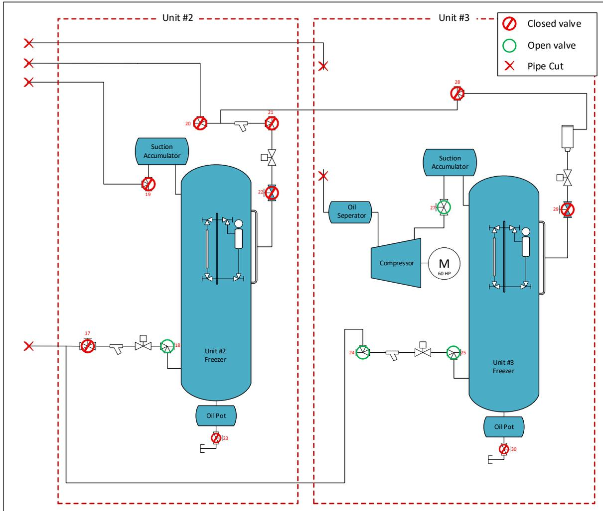
Figure 11: P24 Freezers Piping Configuration As-Found Post Incident (Unit #2 left and Unit #3 right)
