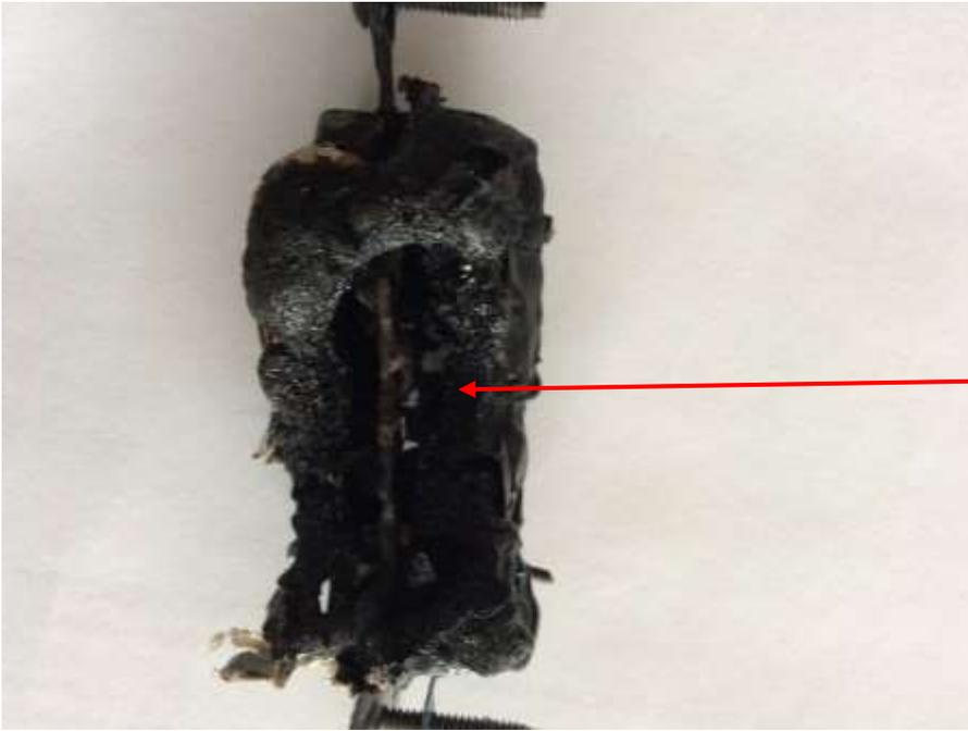
The ungrounded (hot) terminals are missing off the side of the receptacle and the high heat from the arc has disintegrated the side and back of the receptacle body.
