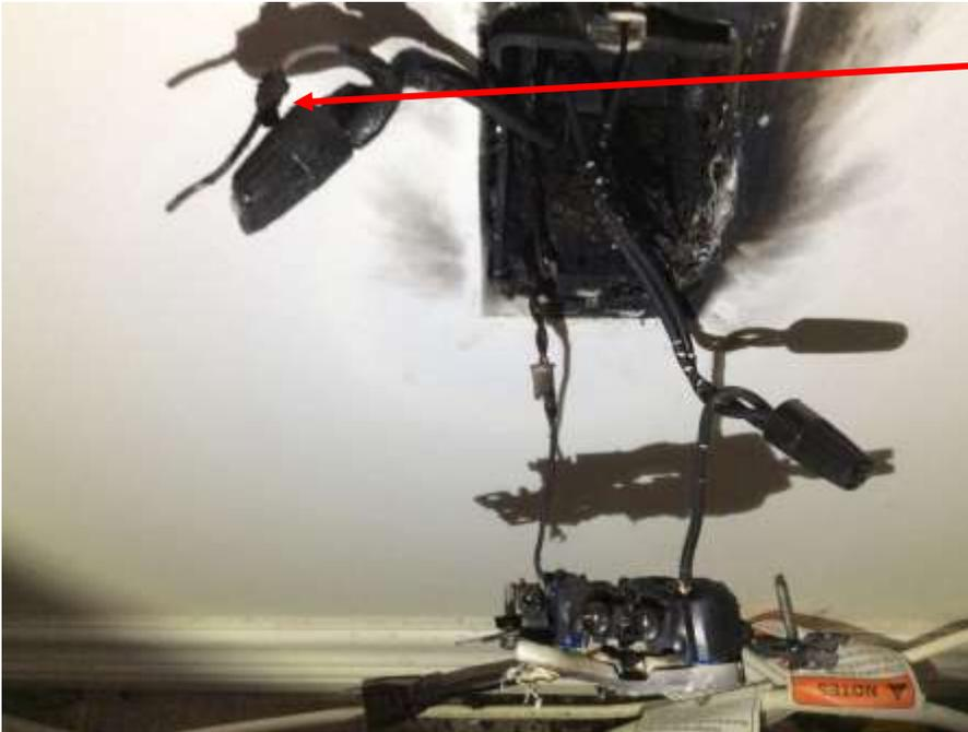
Ungrounded (hot) conductor is burnt off of receptacle. Wire connector is also melted.
