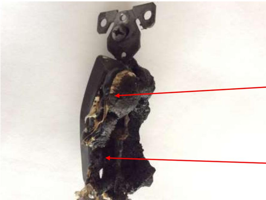
Melted plastic tabs off of the top of the power strip in the receptacle.
