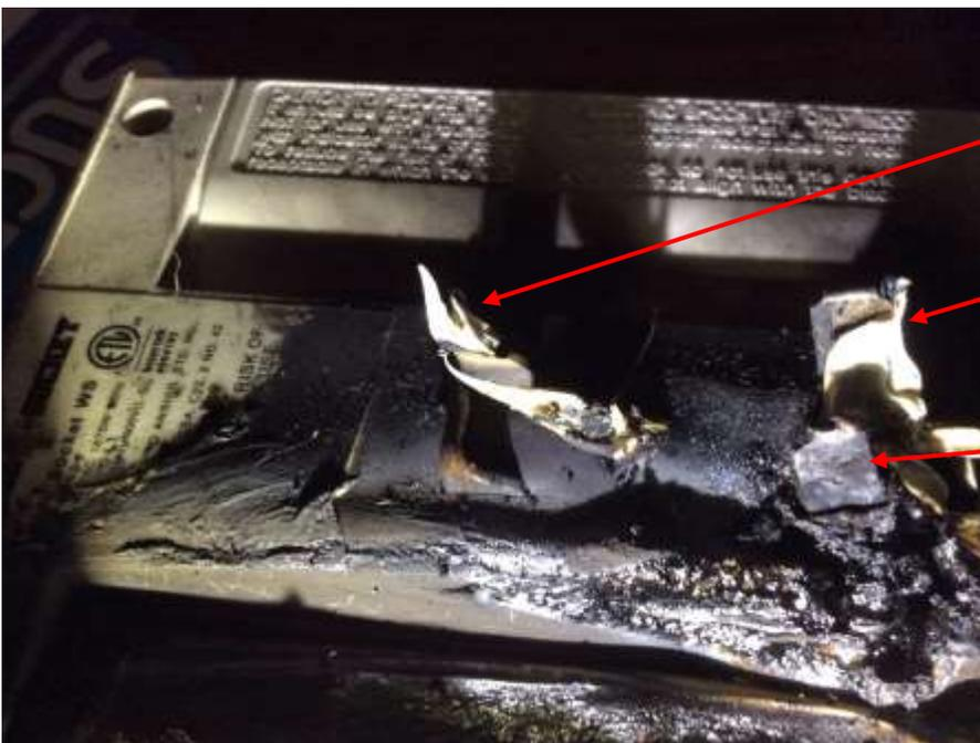
Plastic tabs have melted off of the top of the power strip.
