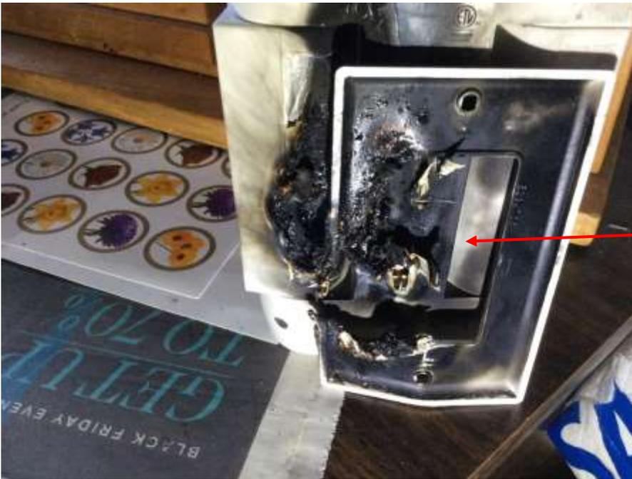
Cover plate and back of surge protected power strip aligned.
