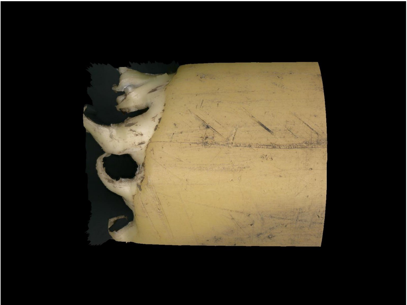
Image 11 – Macro image of gas pipe break from an independent testing laboratory
