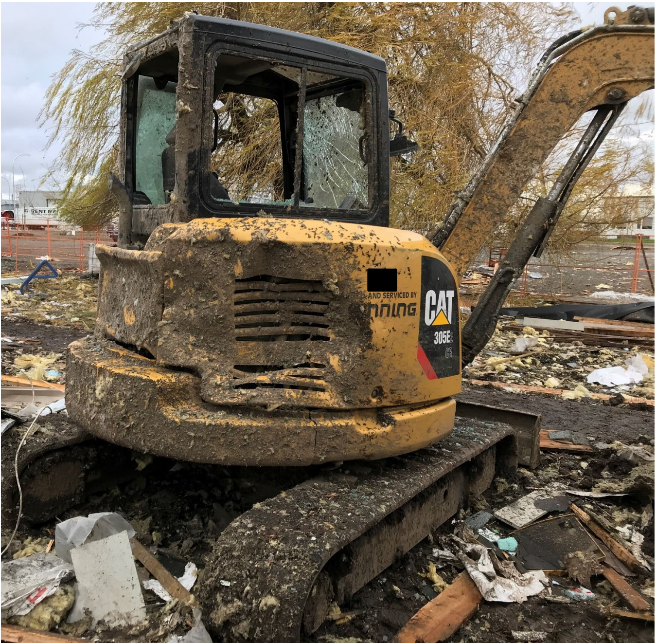
Image 7 – Excavator damage from the blast and flying debris from the explosion.
