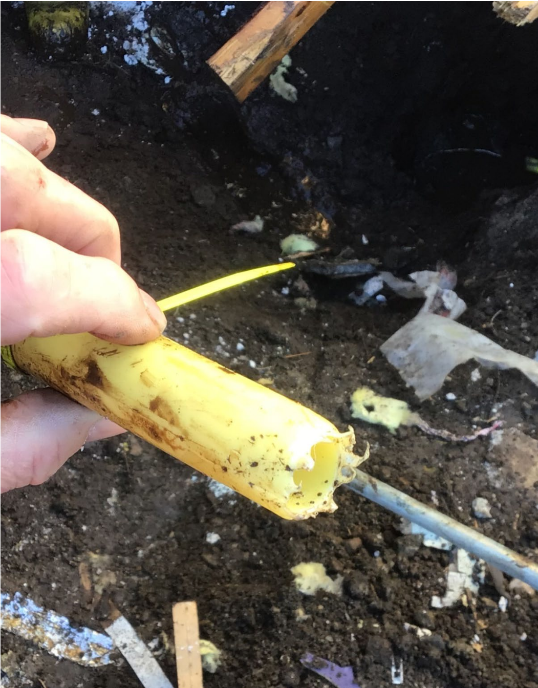
Image 10 – Close image of the severed end of gas pipe.
