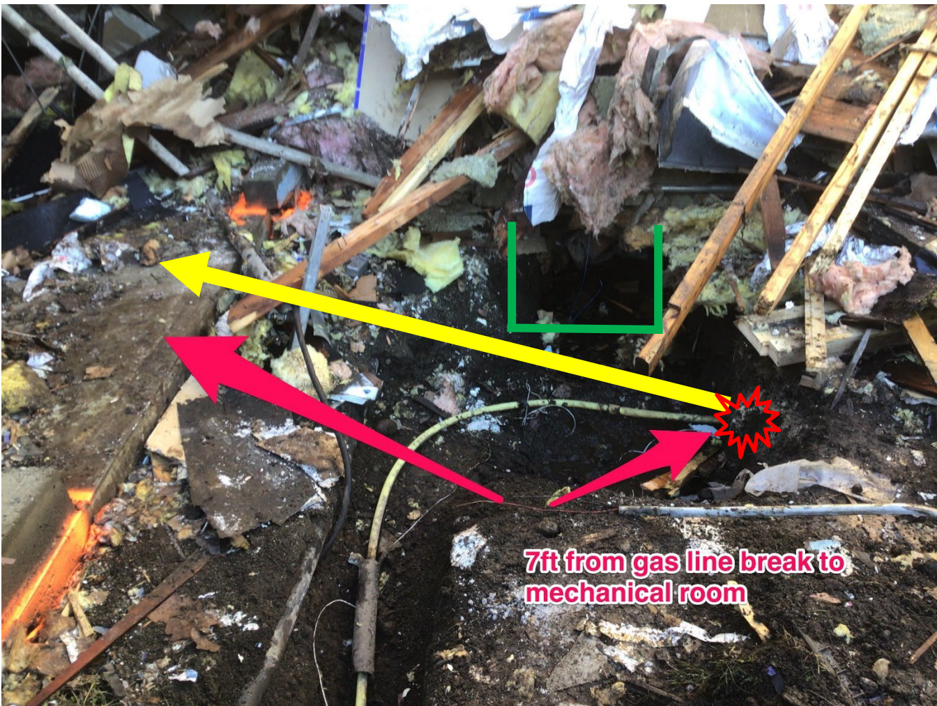
Image 9 – The gas pipe laid back in the hand dug trench after the incident. The red arrows indicate the pipe break 7 feet away and centered to the mechanical room doorway opening. The green lines indicate the location of the mechanically dug trench. The yellow arrow indicates the direction of gas flow from the broken pipe towards the mechanical room door opening. The red symbol indicates the location of the gas pipe strike.
