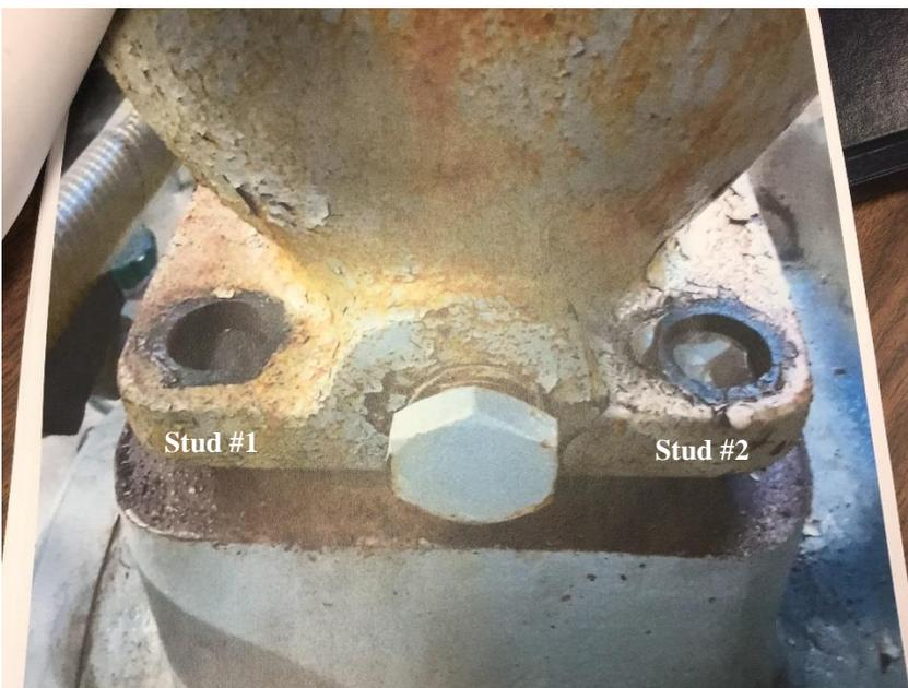
Figure 2: Broken studs. (The nuts and part of the stud is not shown)
