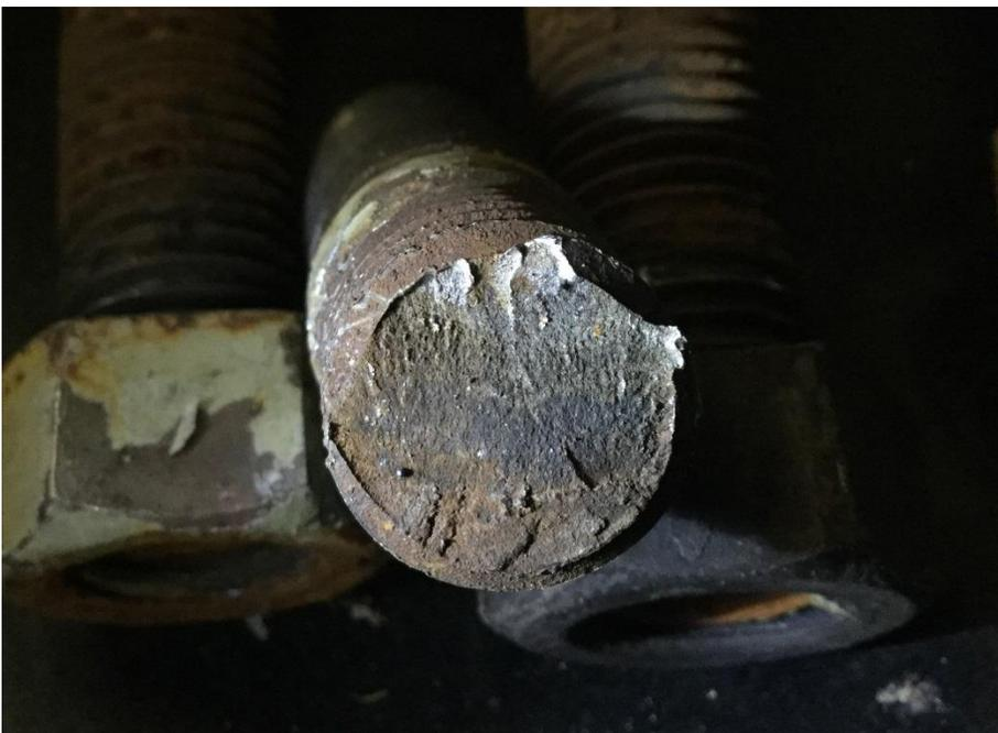
Figure 4: Fracture face of stud #1
