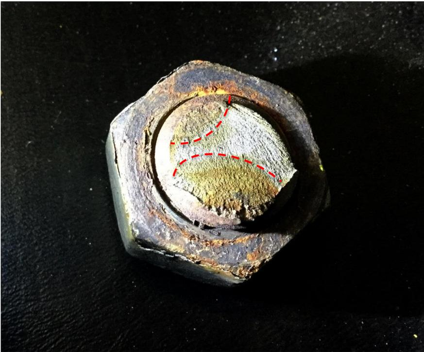
Figure 3: Fracture face of stud #2. The red dashed lines indicate the discoloration at the two separate initiation points.
