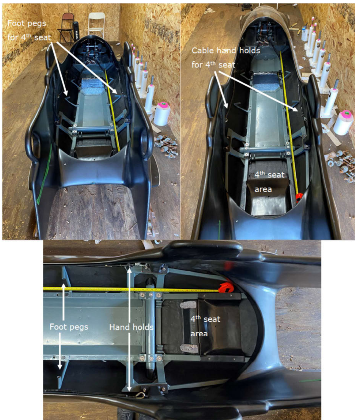
Figure 7. Provided images of a typical Whistler Sliding Centre bobsleigh demonstrating the relative positioning of the foot pegs, hand holds, and seating area for the 4 th rider/occupant of the bobsleigh.
