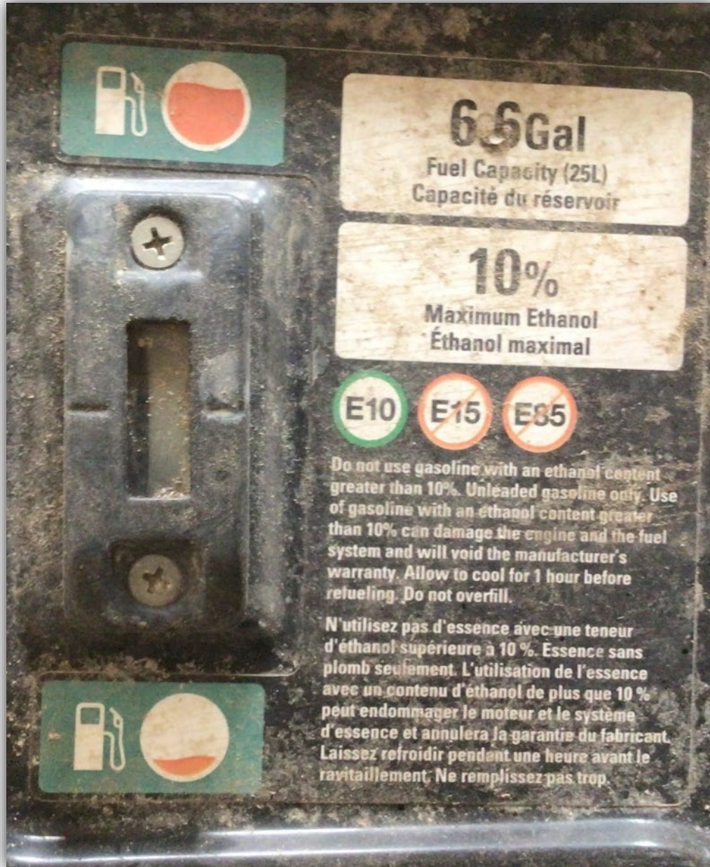
Image 5 – Generator fuel gauge showing empty.
