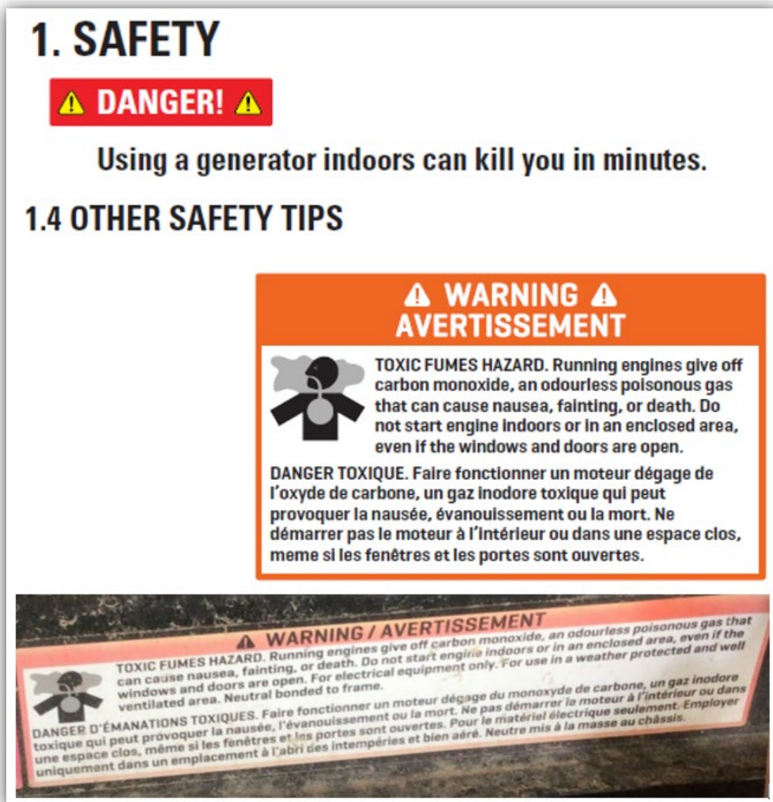
Image 7 – Safety warnings in instruction manual and on generator.
