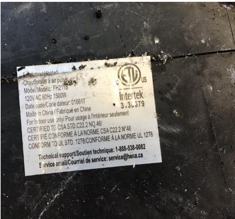
Photo 5: Specification label on electric heater (photo provided by Fire/Rescue)
