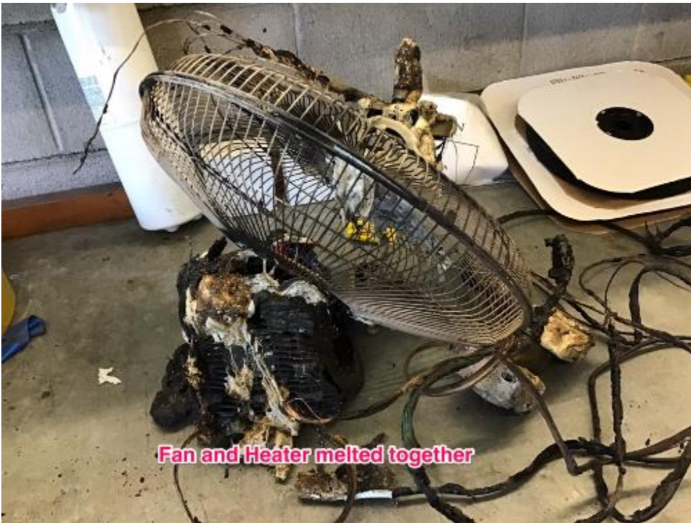
Photo 6: Electric fan and heater partially melted together (photo provided by Fire/Rescue)
