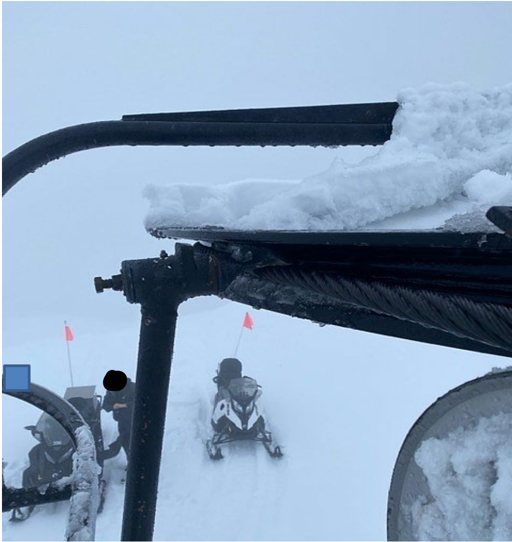
Photo 4 - Grip in correct position as it enters the bullwheel at the return terminal- grip horn and bullwheel flange designed to be in contact when the lift is in motion.
