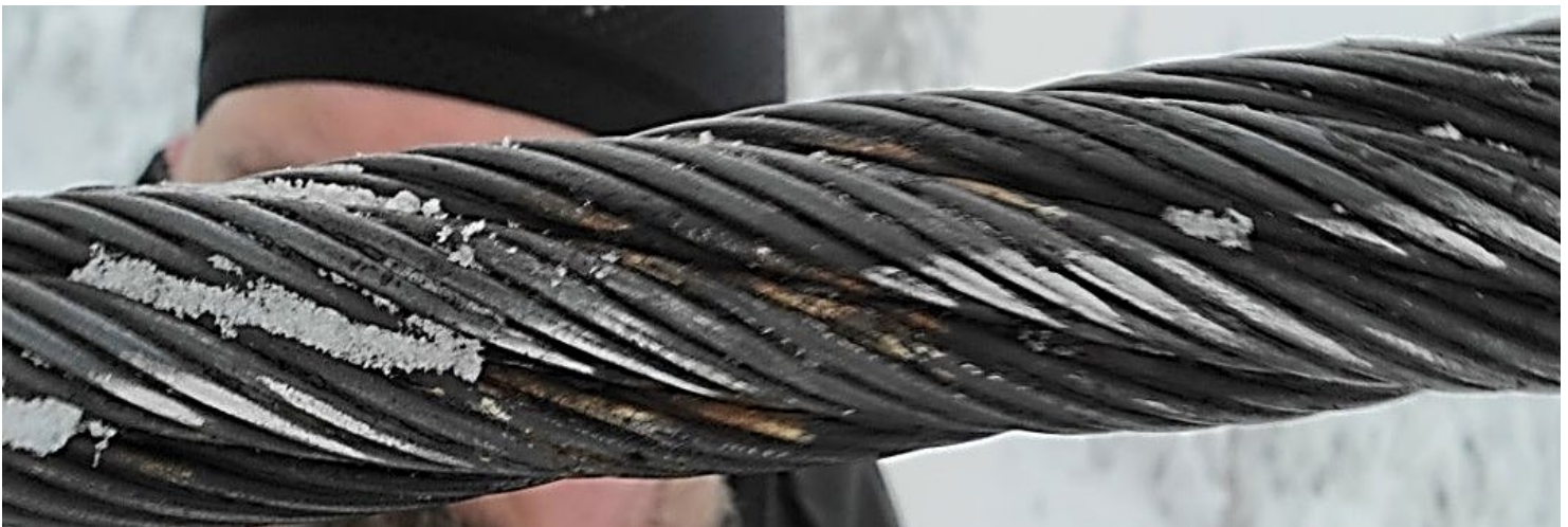
Photo 1 - Indications on haul rope post incident- bright marks where the grip jaw was dragged across the surface of the rope.
