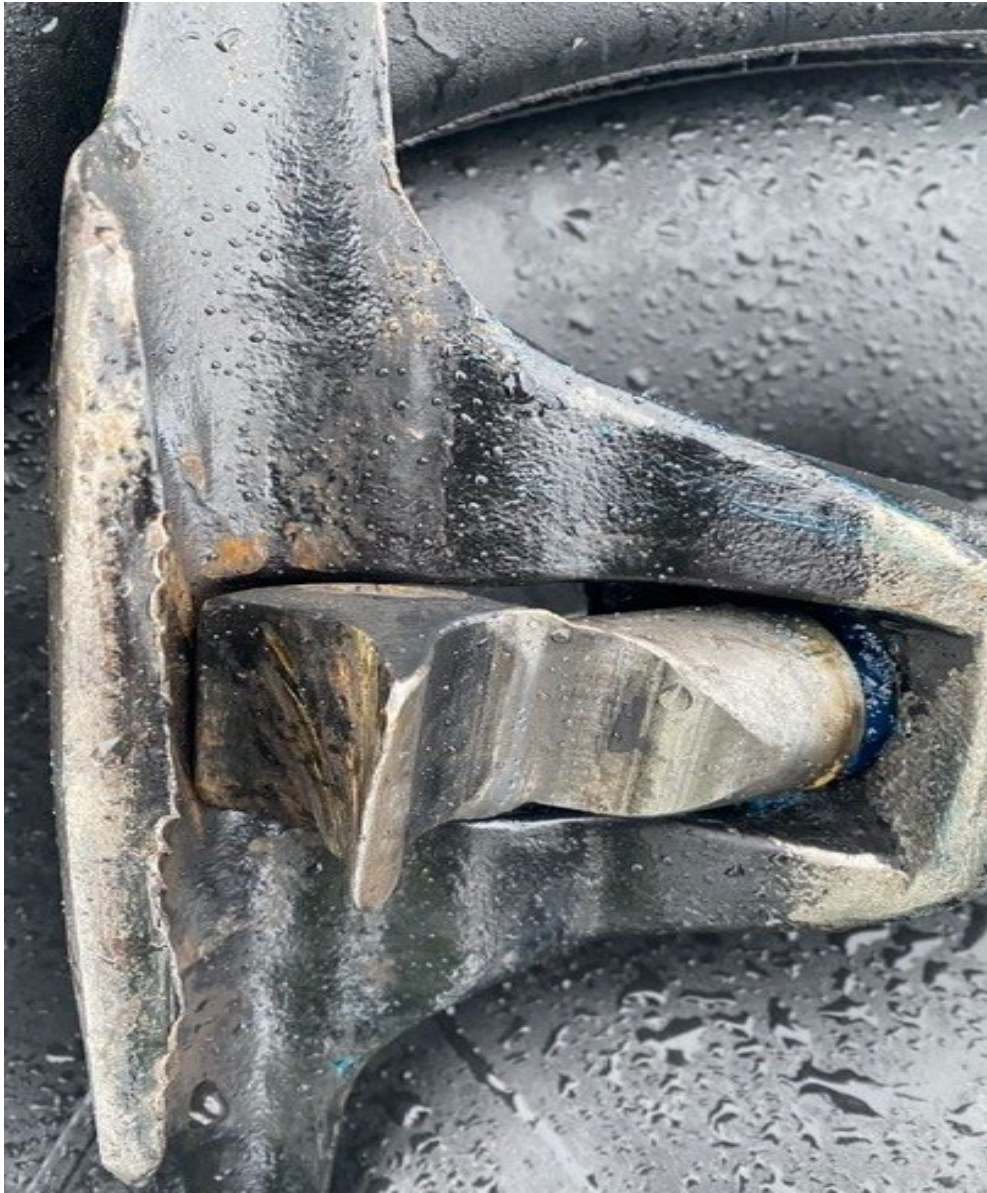
Photo 2 - Damaged grip and grip jaw post incident - rope lay indications found on grip components. The large grooves on grip are to manufacturers design and correspond to the lay of the haul rope.
