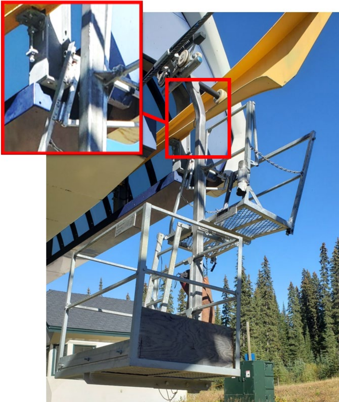
Photo 2 – The work carrier at the lower station. [RED] The area of contact between the upper handrail and the station.
