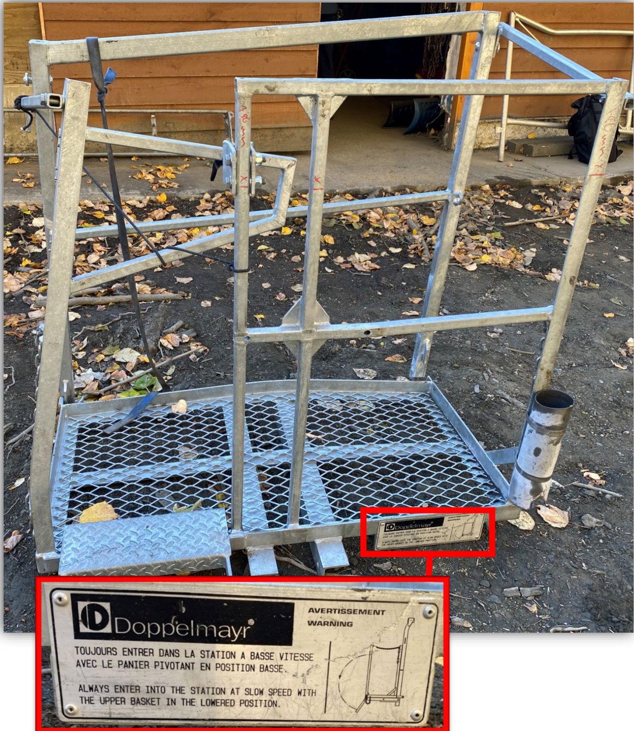
Photo 3 – Upper platform of work carrier removed after the incident showing the damaged handrail. [RED] Warning tag affixed to the work carrier platform.
