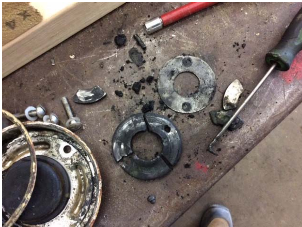
Broken Carbon Thrust Bearing
