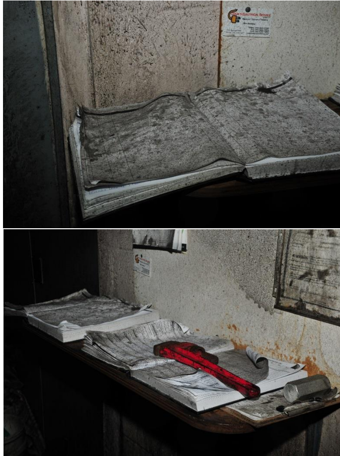
Photos C6-3 and Photo C6-4: View of opened books contaminated with brine spray on a shelf on the mechanical room's south wall. Note the shadowing from spray, suggesting that the spray was directional and projected at and around different components (not evenly misted or distributed throughout the mechanical room).
