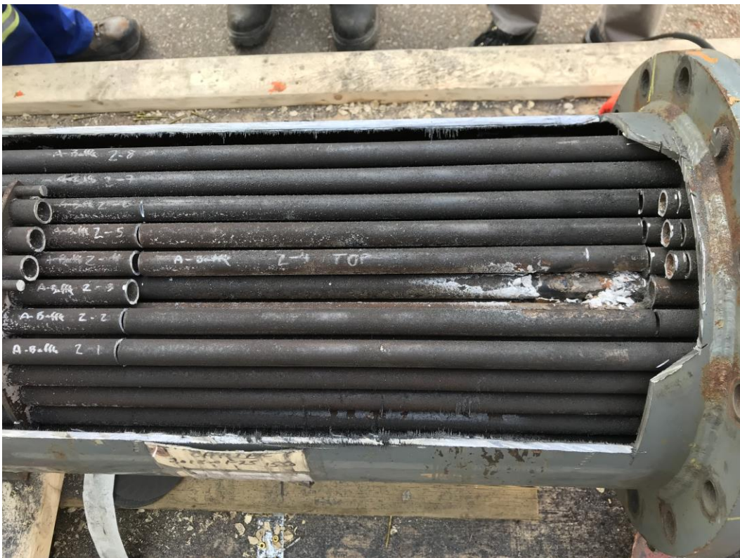
Photo C3-8 and Photo C3-9 (below): Chiller with shell section and top three tubes cut away at return end – white scale indicates brine leak into shell (ammonia) side of heat exchanger. Below shows leaking tube removed with scale deposits and spray patterns on adjacent tubes.
