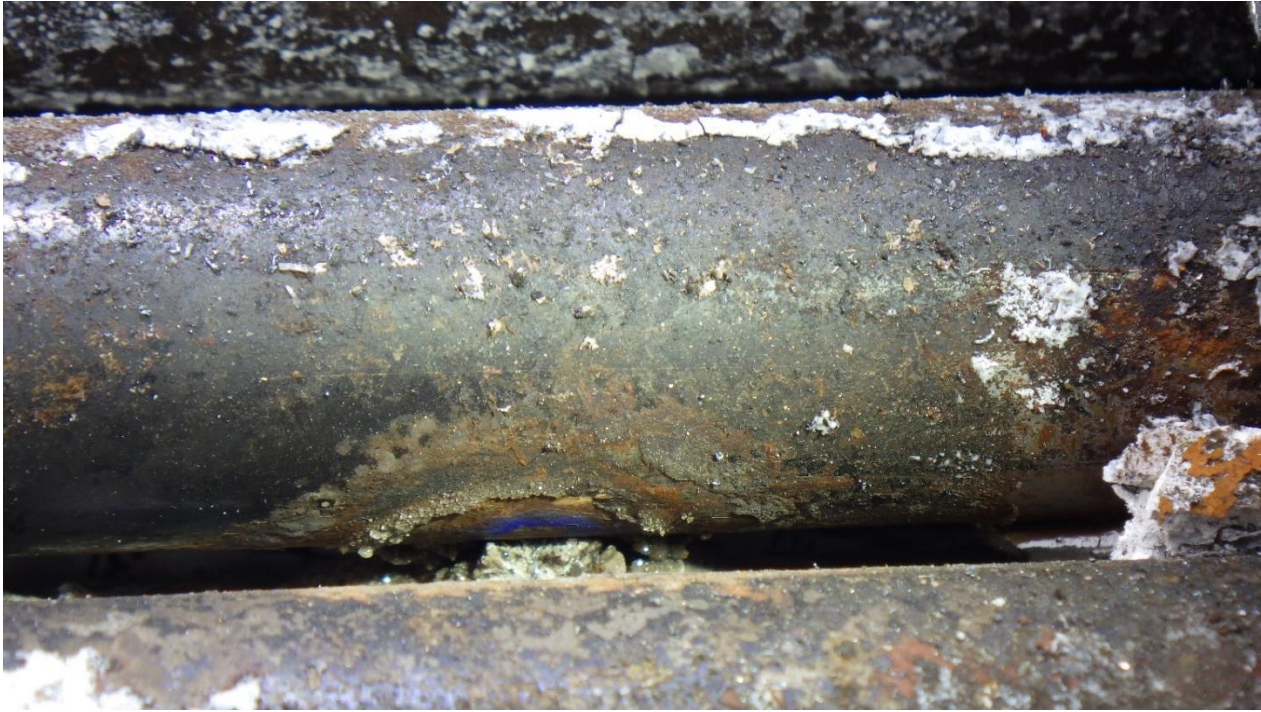
Photo C3-10 (above) and Photo C3-11 (below): Above shows evidence of spray from tube (brine) side into shell (ammonia) side. Photo C3-11 shows close-up of inside surface of the tube and leak location showing erosion of metal from ammonia leak into tube.
