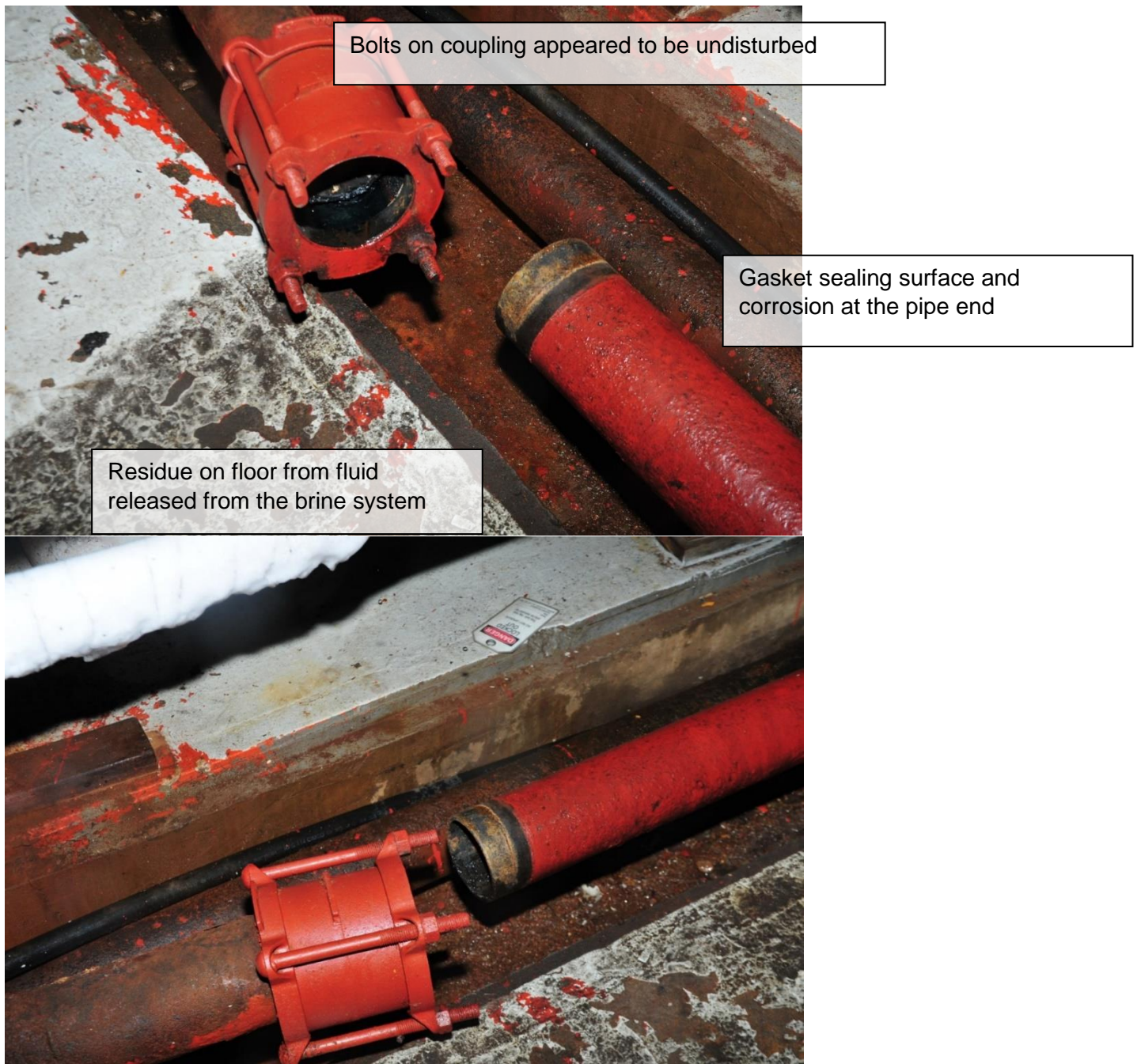
Photo C5-1 and Photo C5-2: Separated brine system coupling.
