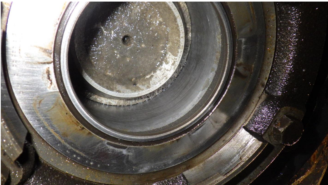
Photo C4-4: Salt deposits/residue from the brine on one of the compressor's upper piston
