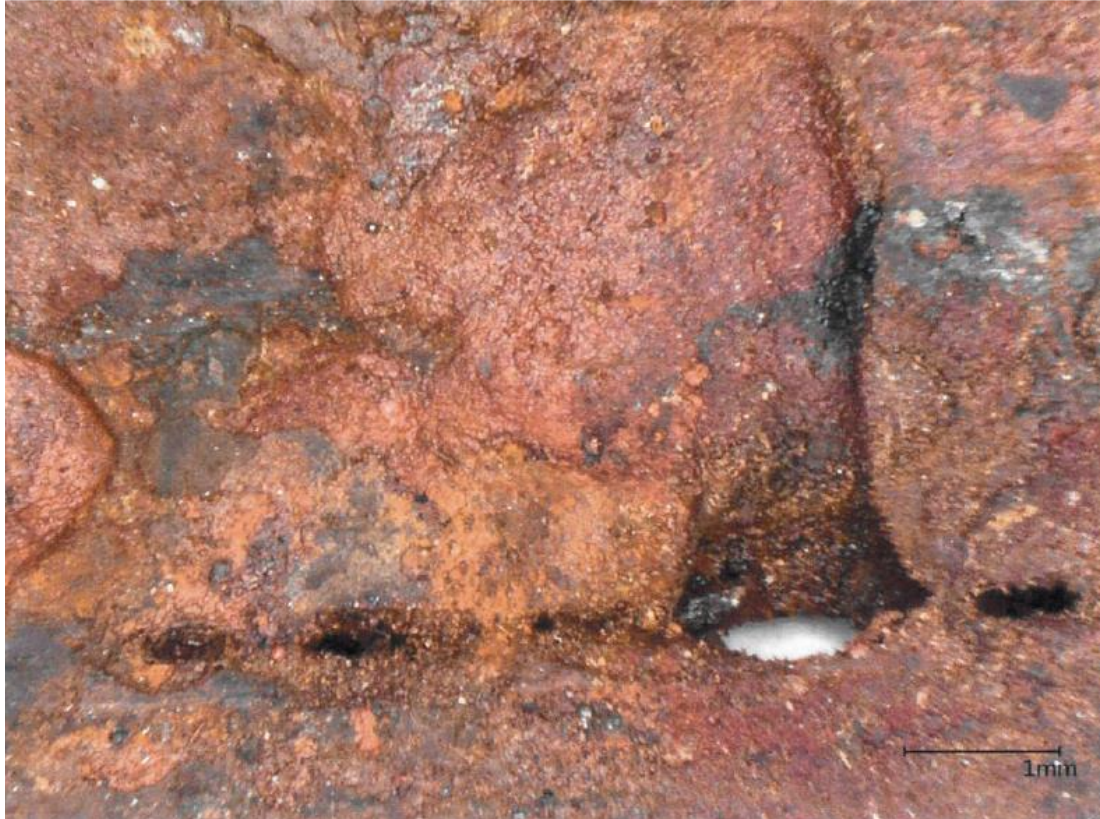
Photo C3-10 (above) and Photo C3-11 (below): Above shows evidence of spray from tube (brine) side into shell (ammonia) side. Photo C3-11 shows close-up of inside surface of the tube and leak location showing erosion of metal from ammonia leak into tube.
