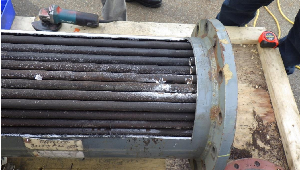
Photo C3-8 and Photo C3-9 (below): Chiller with shell section and top three tubes cut away at return end – white scale indicates brine leak into shell (ammonia) side of heat exchanger. Below shows leaking tube removed with scale deposits and spray patterns on adjacent tubes.
