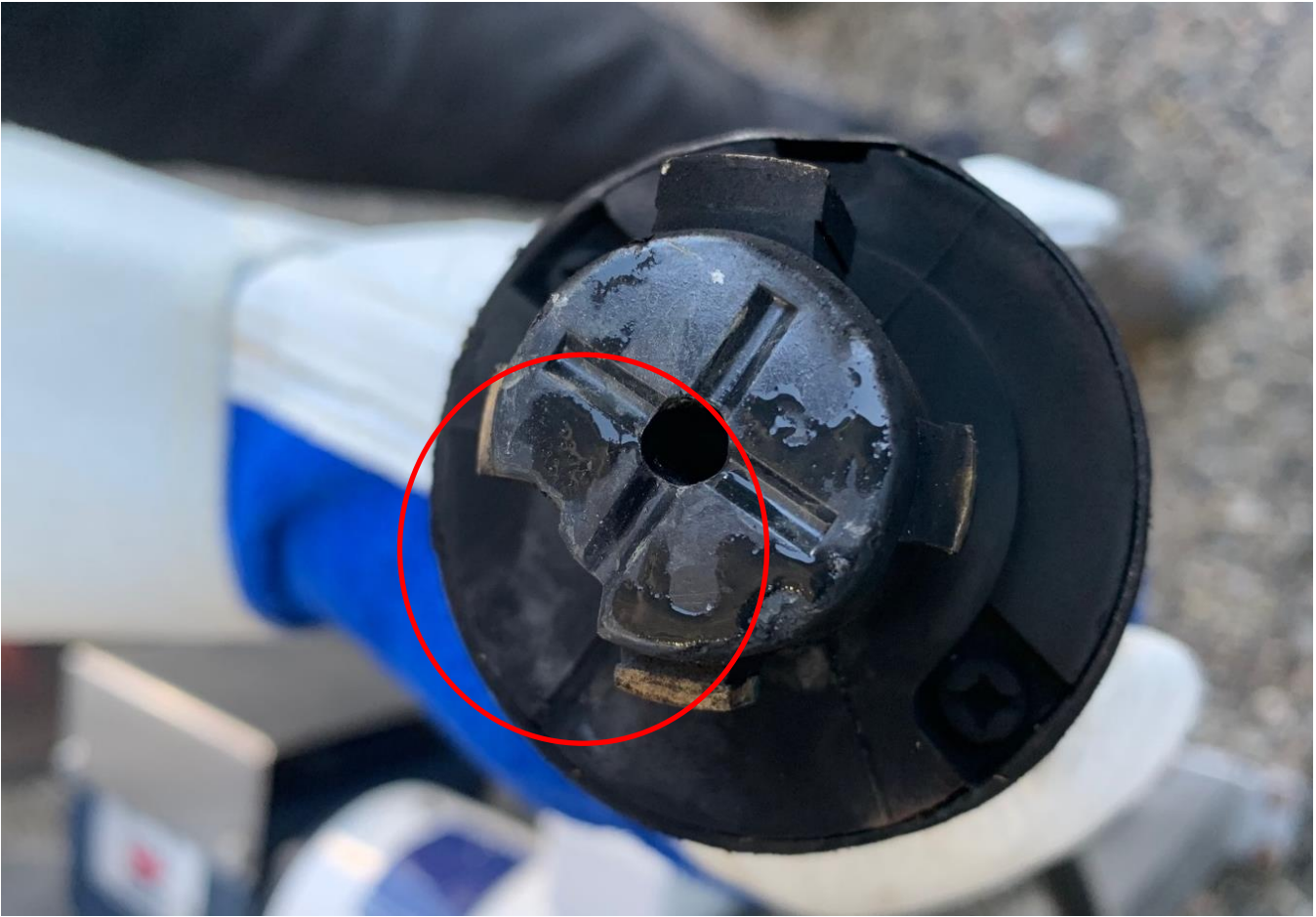
Photo 2: Fail point of receptacle
