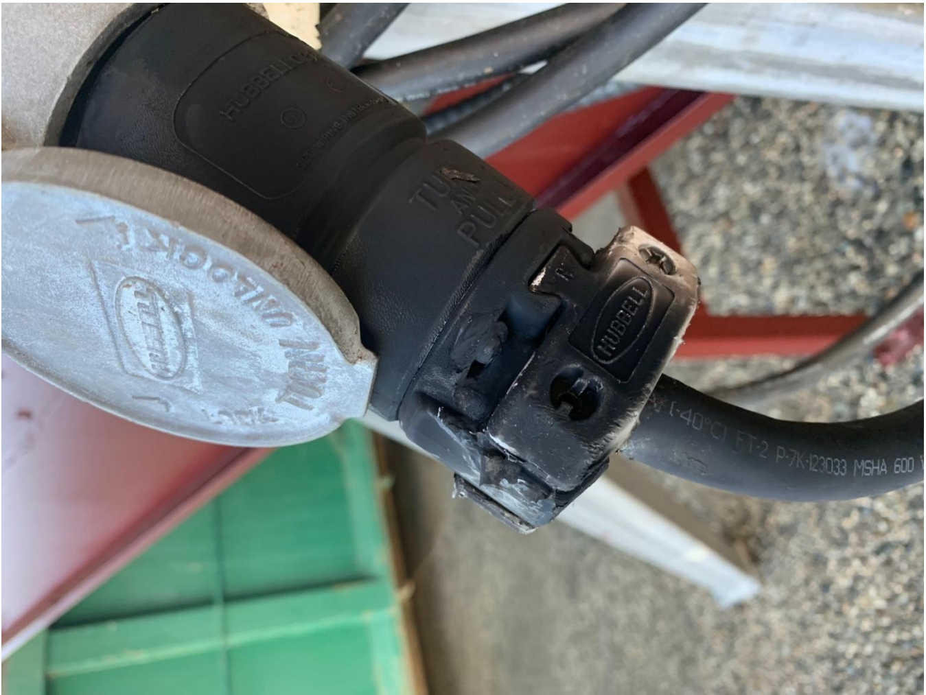
Photo 1: Damaged twist lock receptacle for portable equipment: 30A 480V
