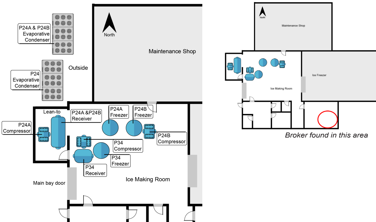
Diagram #2: Plant layout during ice production
