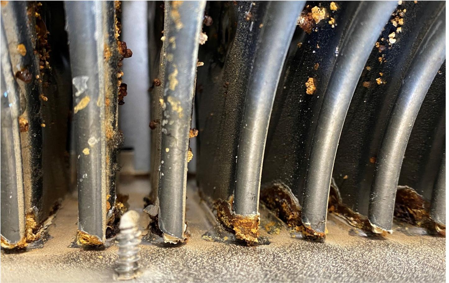
**Photo 4** – Corrosion on the exterior of the secondary heat exchanger tube inlets.
