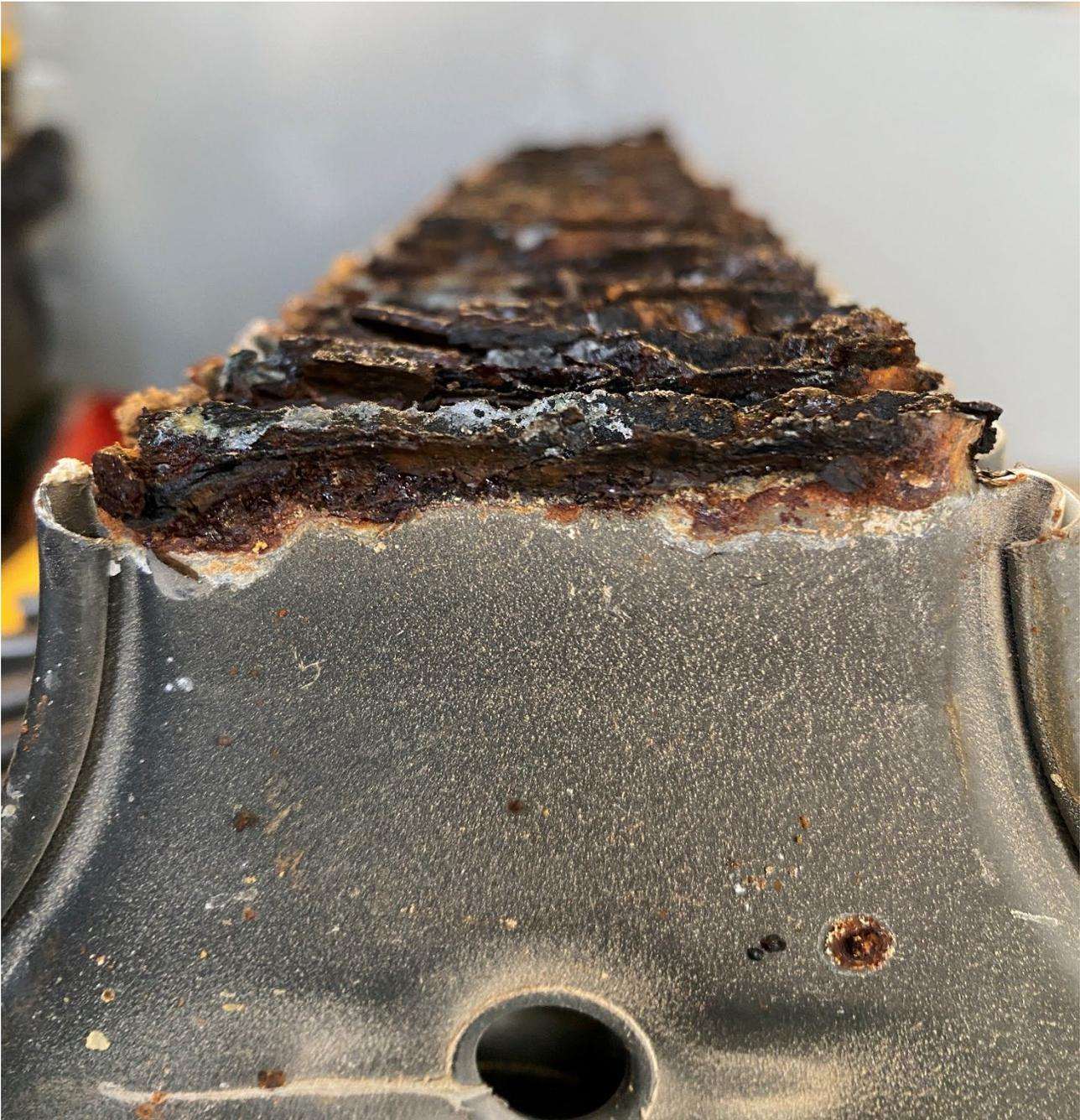
**Photo 8** – Profile showing the corrosion of the heat exchanger inlet tubes.
