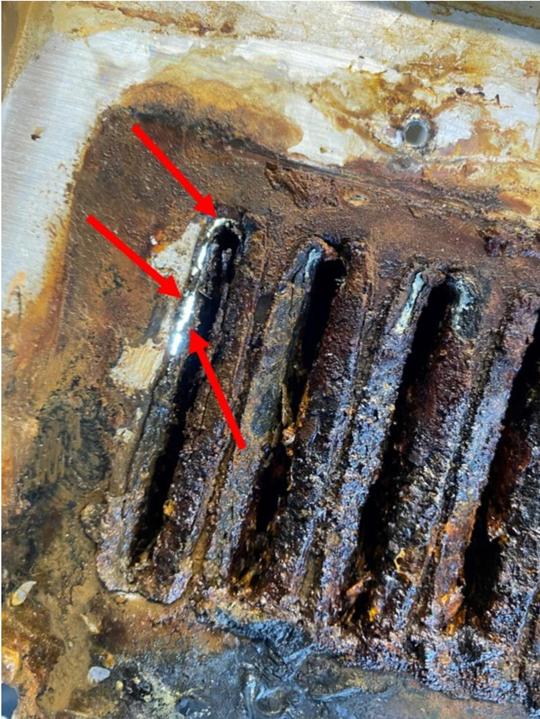
**Photo 6** – Red arrows show light passing through holes from corrosion where the tube connects to the coupling box from the interior.
