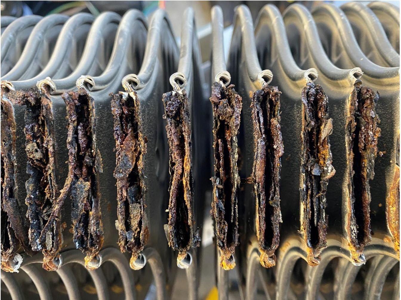
**Photo 7** – Close up photo shows corrosion and delaminated polypropylene liners at the heat exchanger inlet tubes.
