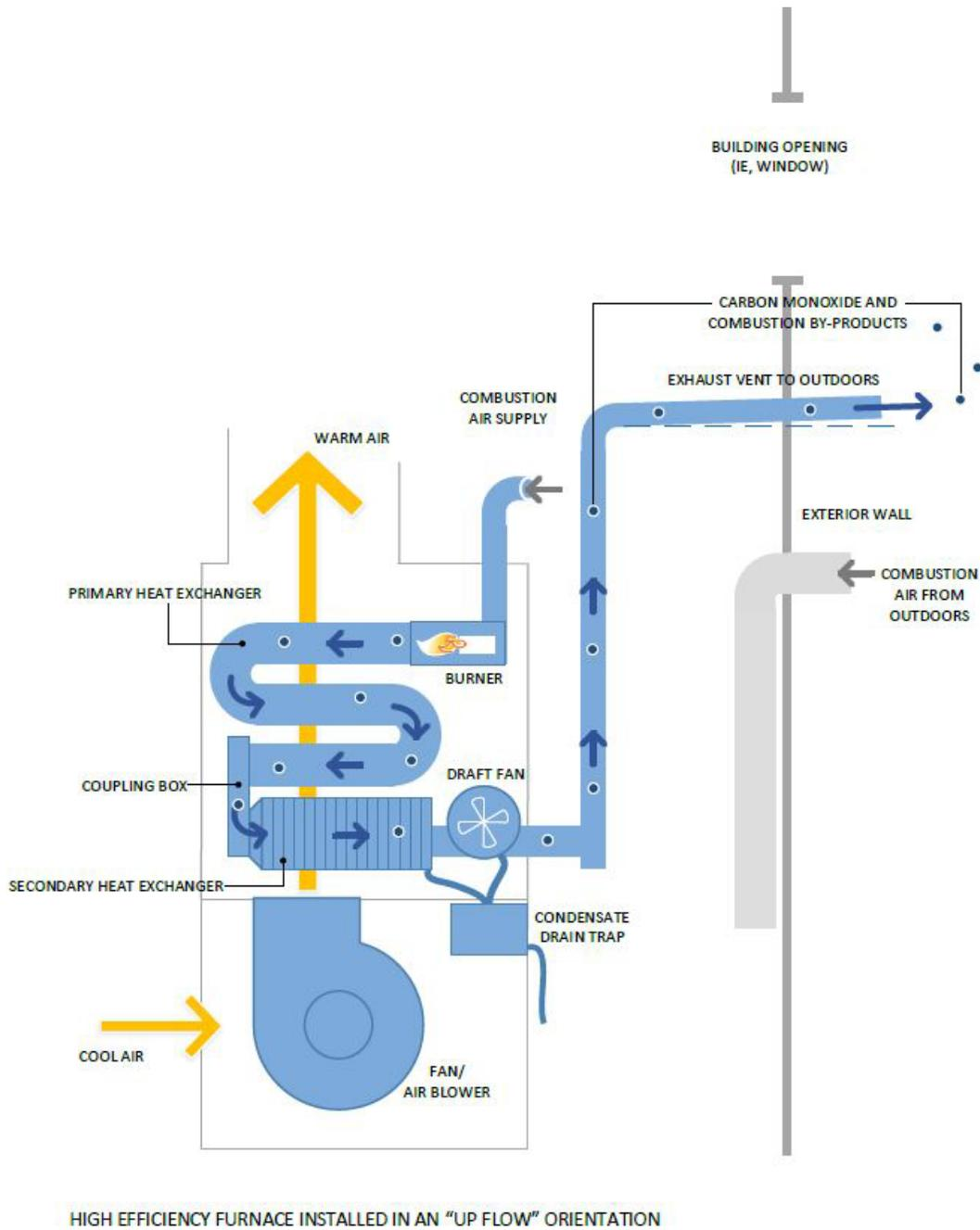
**Diagram 1** – Showing typical furnace operation. Arrows show direction of flue gas flow and dots represent CO.
