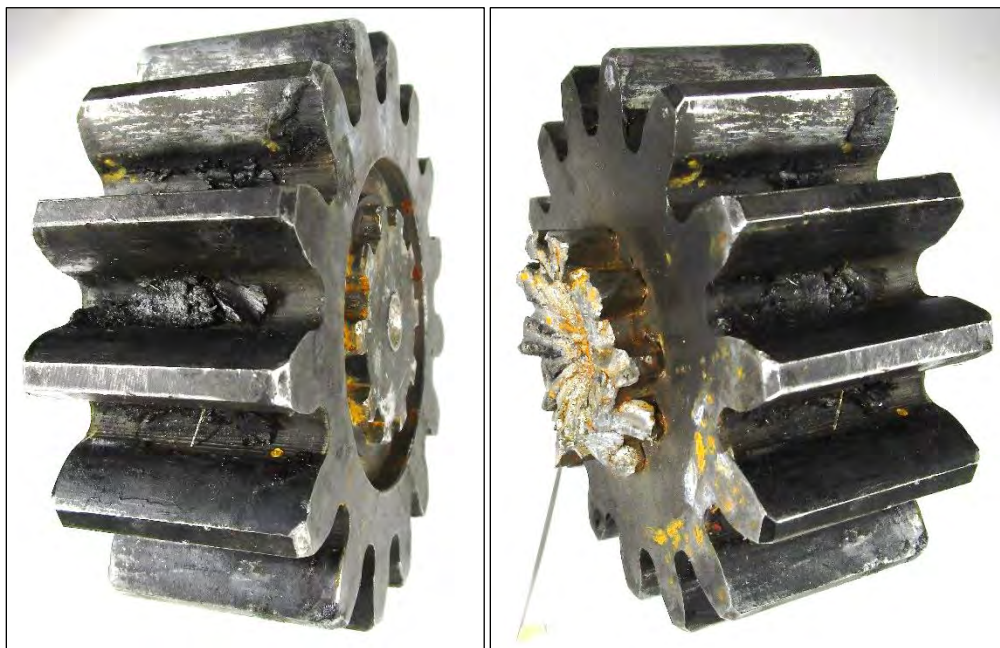
Figure 25 Replacement gear with broken shaft inside.
