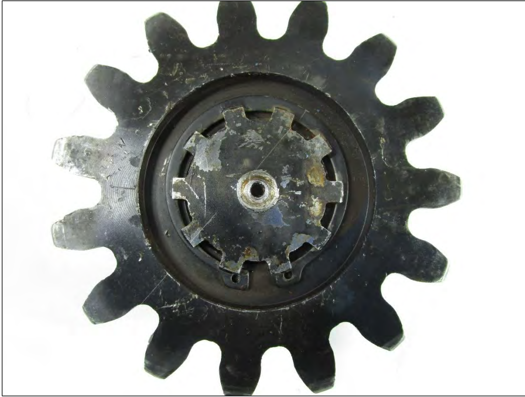
Figure 4 The outboard end of splined shaft inside bottom gear.
