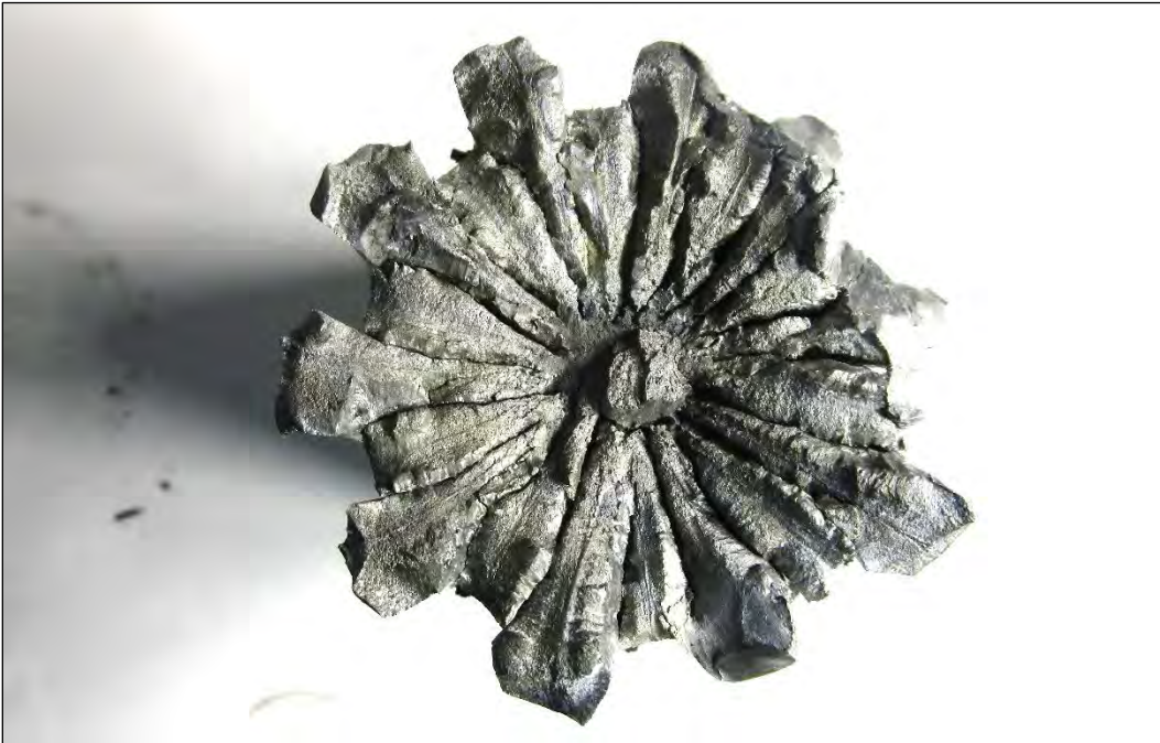
Figure 6 General appearance of shaft fracture after cleaning.
