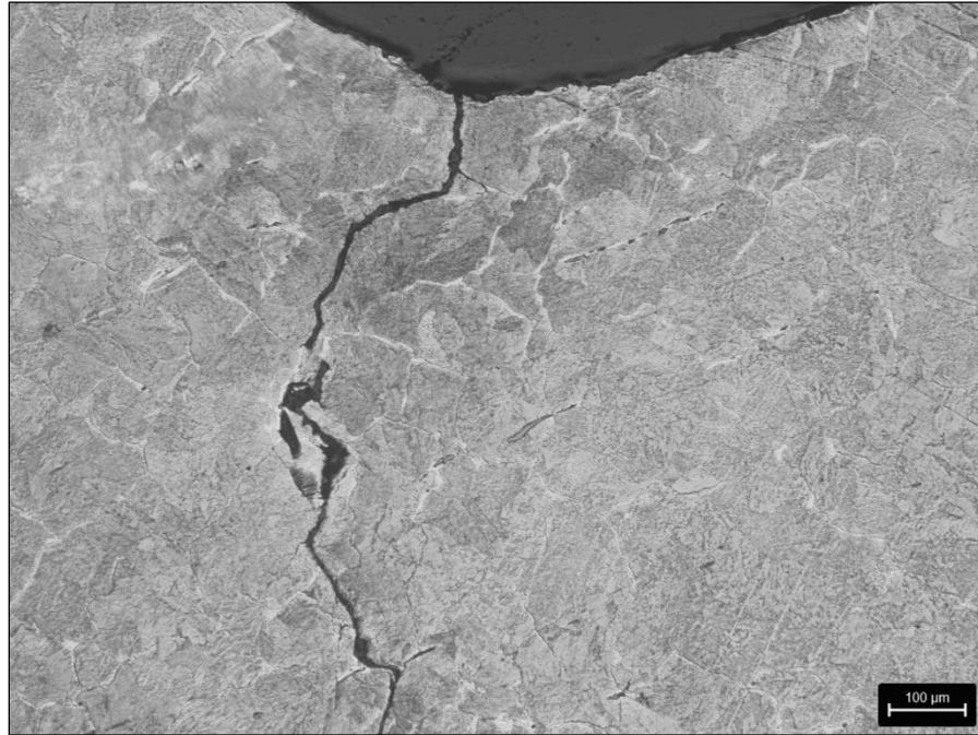
Figure 21 Profile of large tooth root crack and surrounding microstructure.
