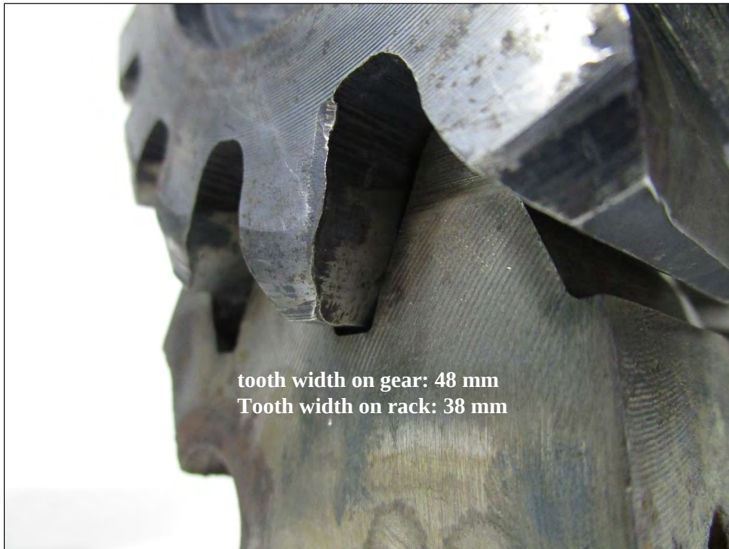
Figure 24 Illustration of meshing teeth of gear and rack.
