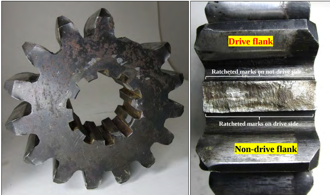
Figure 28 Broken tooth and its fracture.
