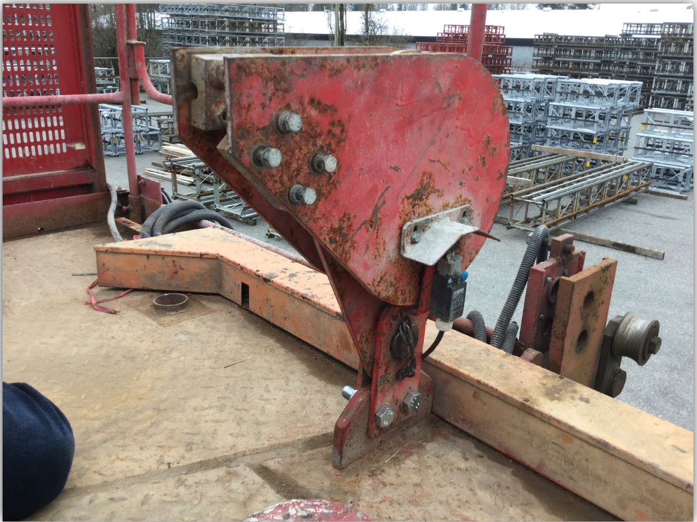
Image 1 - A typical "Leveler" unit that attaches to the top of a construction hoist cab.
