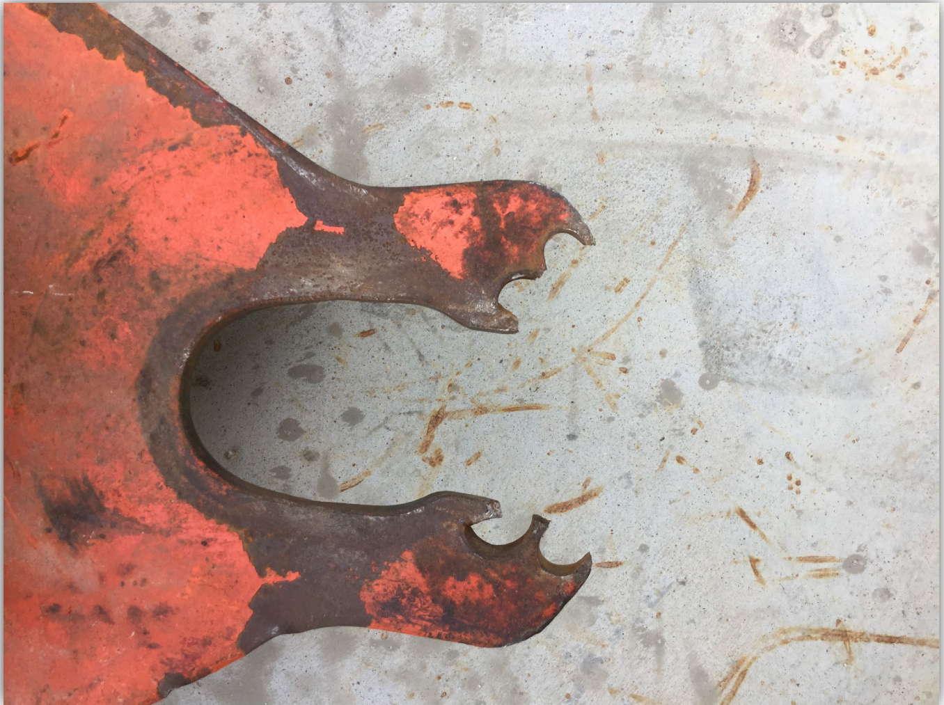
Image 4 - Close-up of "leveler" and failure point.
