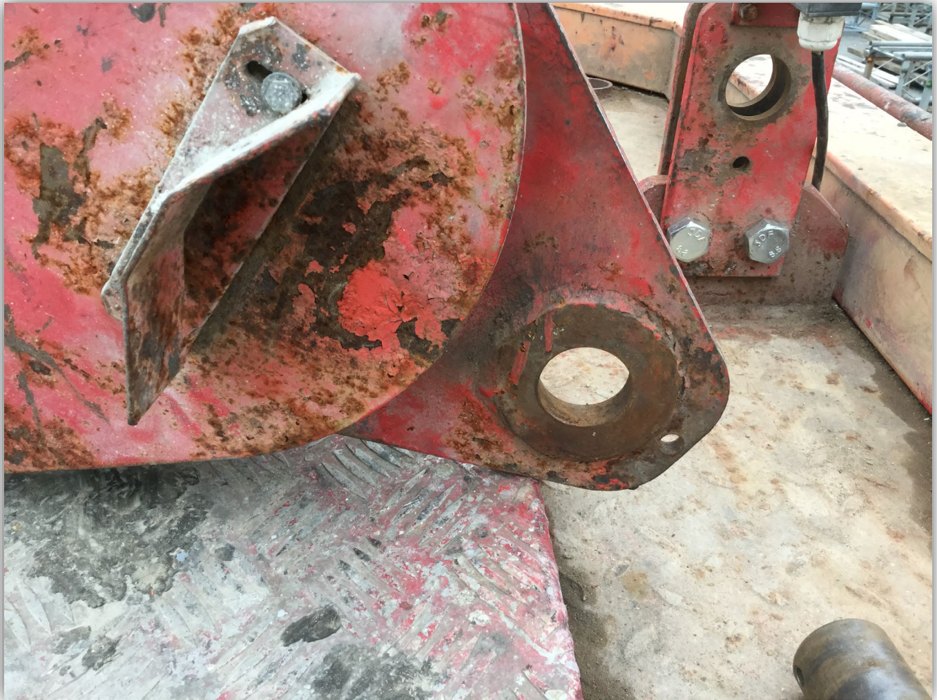
Image 2 - The attach point of a typical “leveler”.
