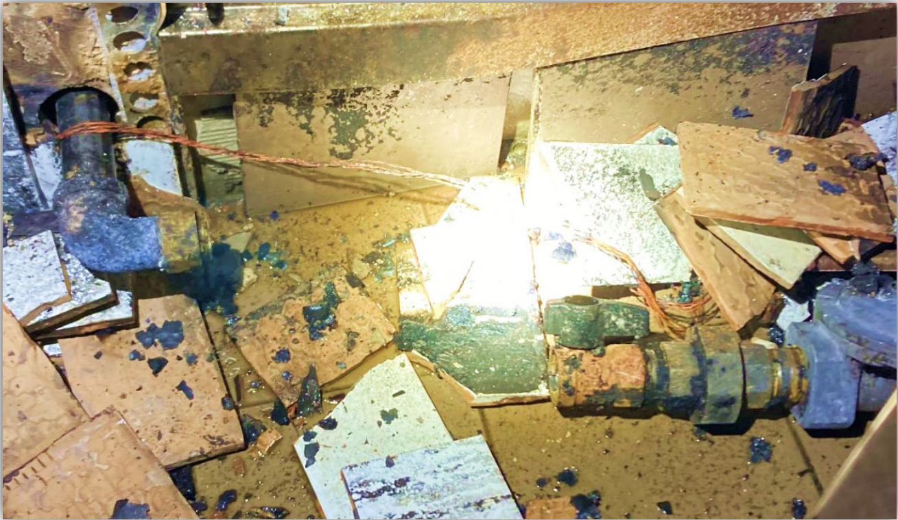
Image 1 - Separation of two-piece ball valve.
