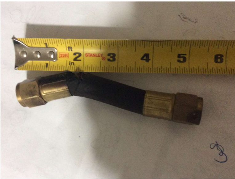
Damaged gas hose
