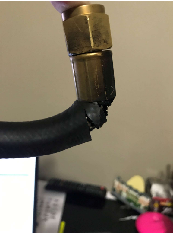
Factory installed hose with sharp bend that caused the damage to the gas hose.
