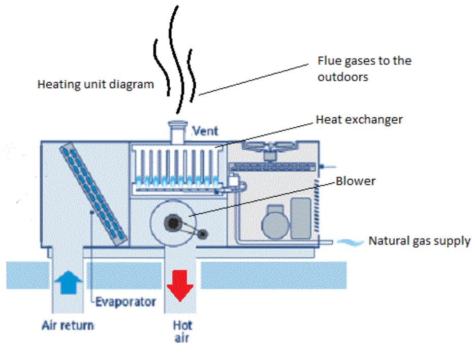
Diagram 1 – Typical rooftop heater. (Benefits of a natural gas roof unit 2021 Energir.com <https://www.energir.com/en/business/equipment/all/roof-unit/>)
