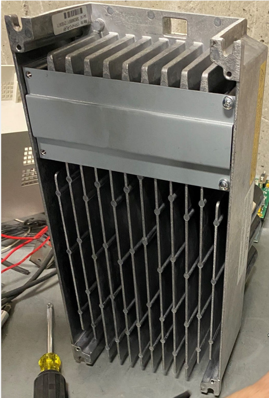
Image 12 – Heat sink with integral fan under cover to cool transistor pack.
