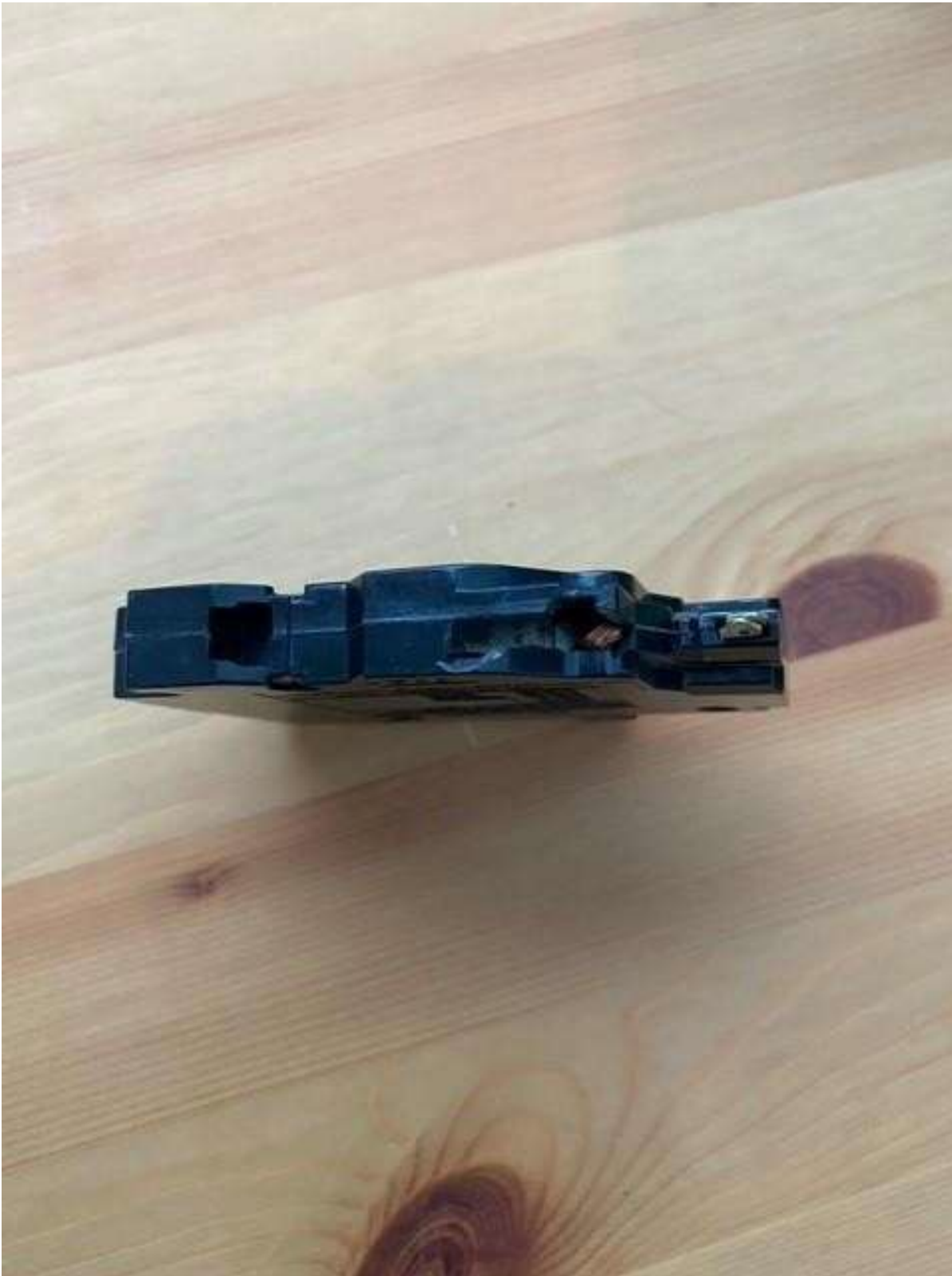
Photo #5 – Underside of damaged circuit breaker
