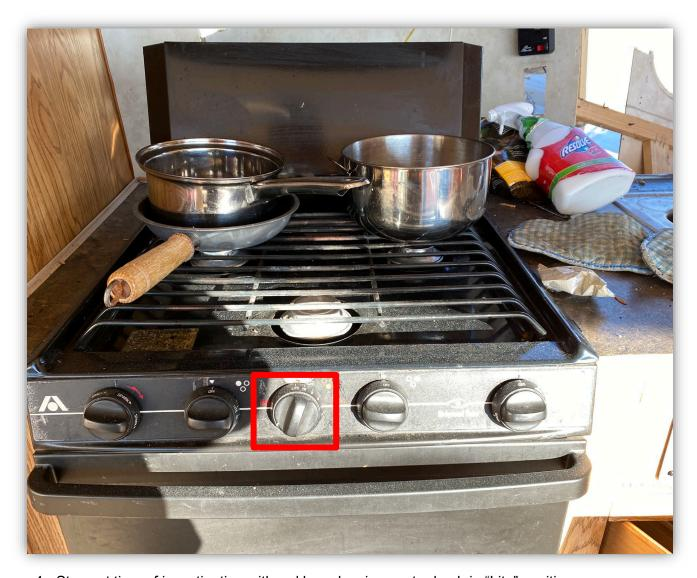
Image 4 - Stove at time of investigation with red box showing center knob in "Lite" position.
