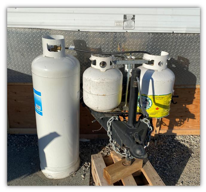
Image 3 - Propane cylinders mounted on front of trailer, including new 100lb propane cylinder and modified supply hose.
