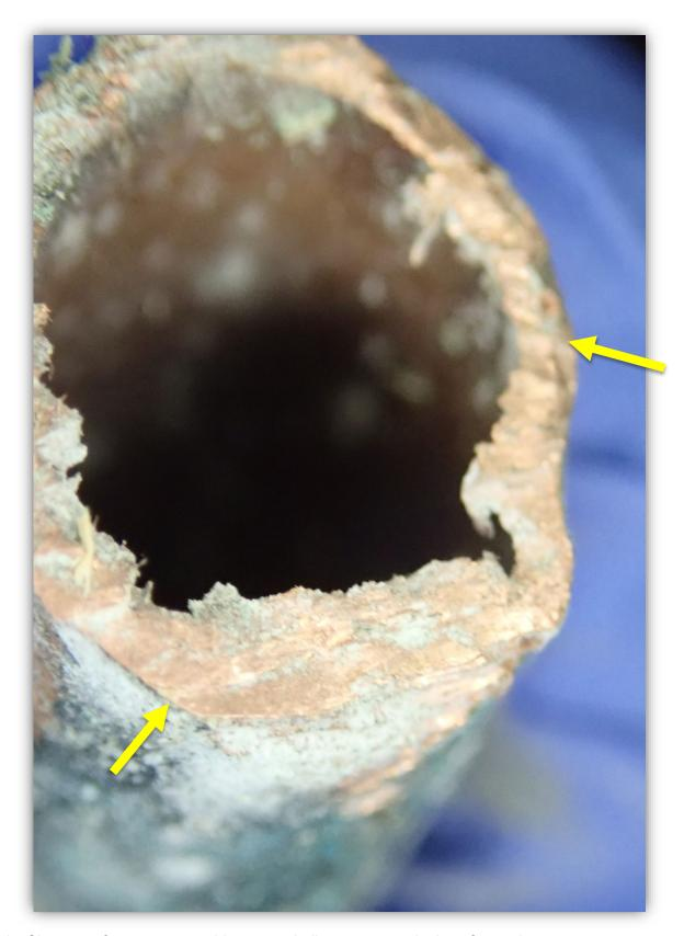
Image 14 - Close up of cut propane tubing arrow indicates cut marks in soft metal.
