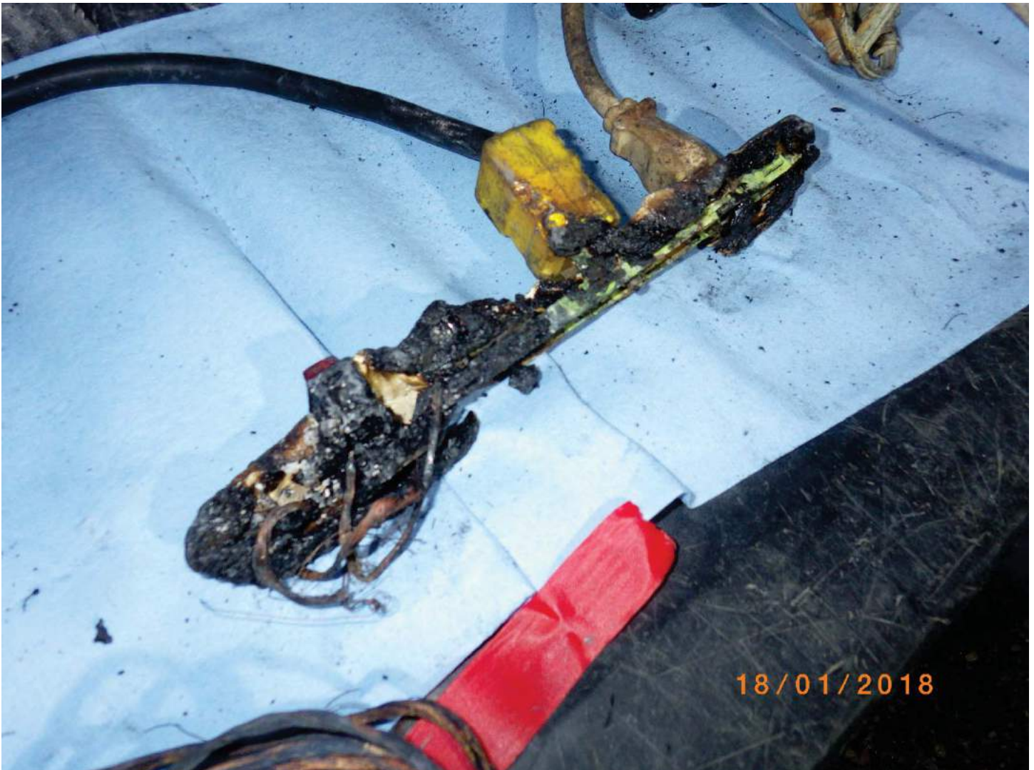
Figure 5 – This photo shows the fire damaged power bar near the end where the flexible cord entered the device and where the switch is located.
