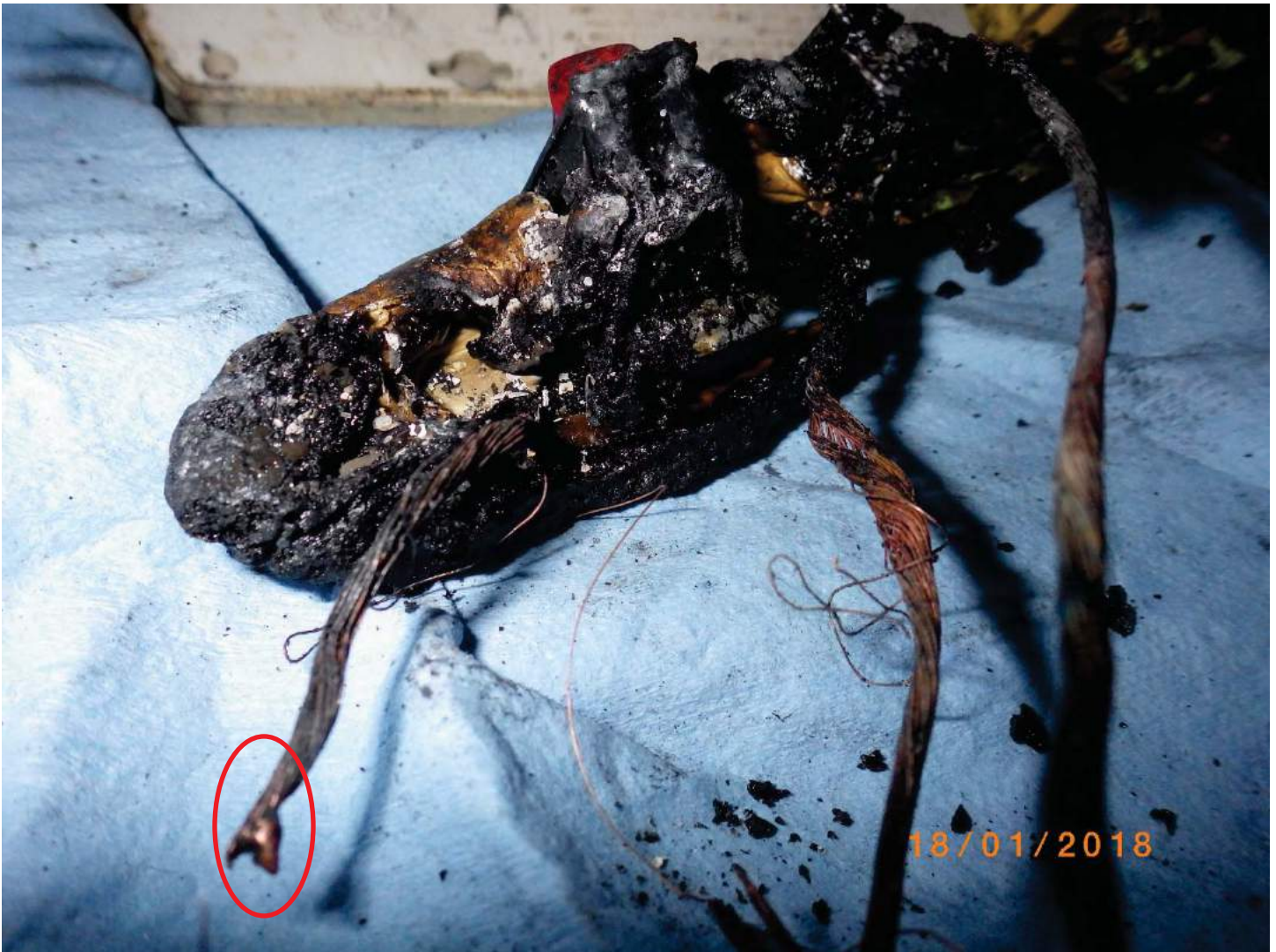
Figure 6 – This photo shows the end of the power bar where the flexible cord enters the device and where the switch is located. It is believed that this area of the power bar is the point of origin based on the damage to the power bar in this location and the corresponding fire damage to the shelving structure. The red oval shows arcing/melting on the flexible cord conductor, indicating that this power bar was energized at the time of the incident.
