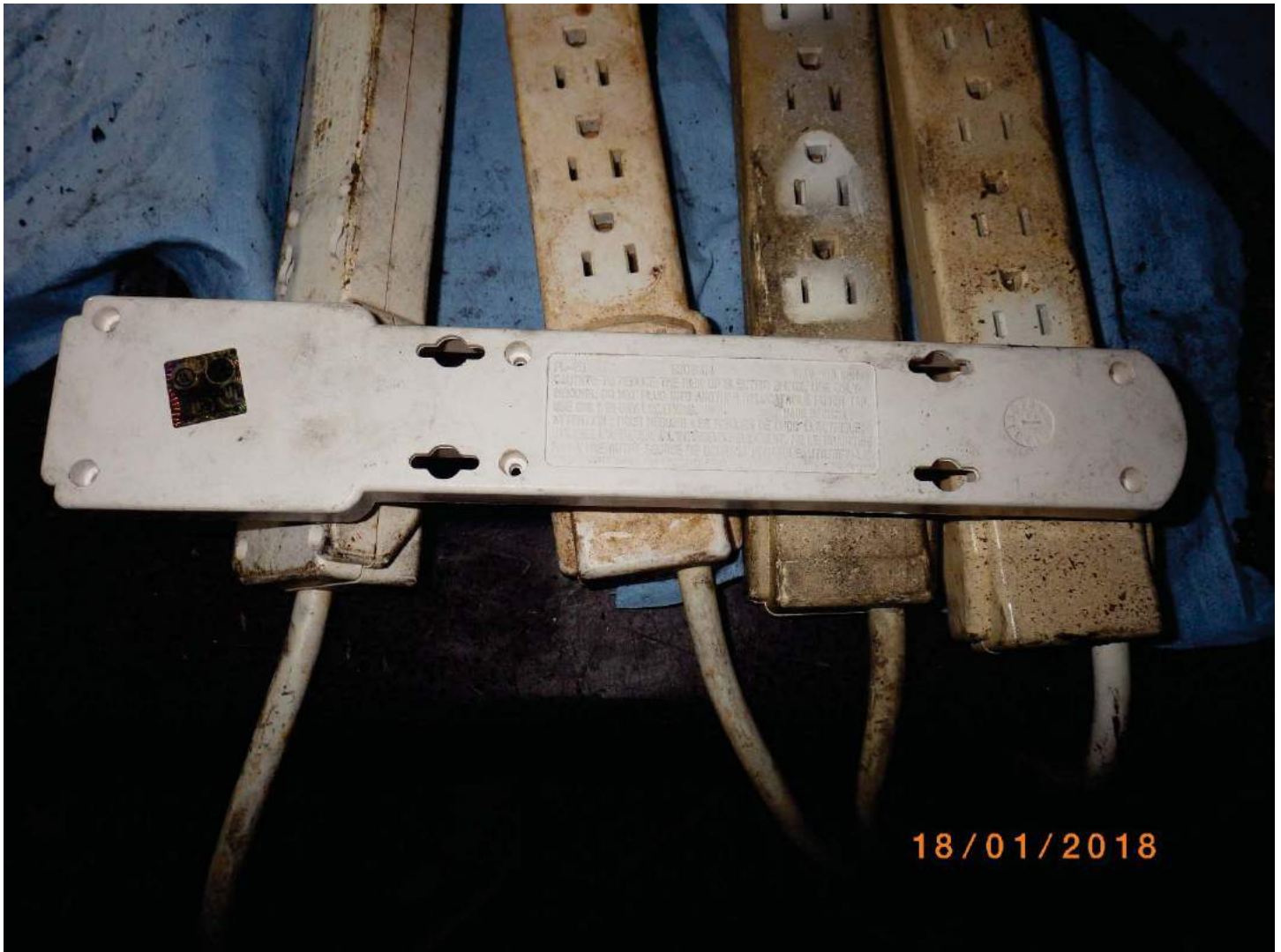
Figure 9 – This photo shows several more exemplar power bars used in the basement growing areas. Note the discolored plastic indicating the wet/humid environment, combined with what appeared to be plant resin or organic matter, and the use of chemical fertilizers and/or pesticides was not ideal for use of this type of equipment that is intended and approved only for use in a dry environment. These conditions will likely cause corrosion and damage to internal electrical components and contacts inside the power bar.
