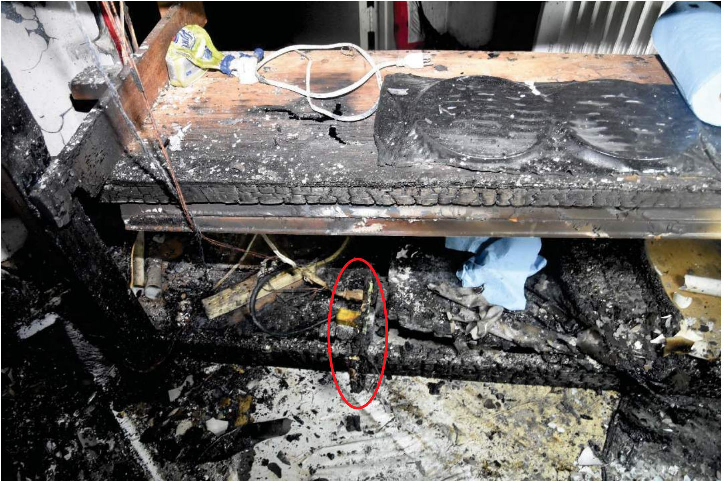
Figure 3 – Photo provided by the private fire investigator. The red outline shows the power bar location viewed from the back of the shelf (shelf pulled away from the wall). This is believed to be the area of origin.
