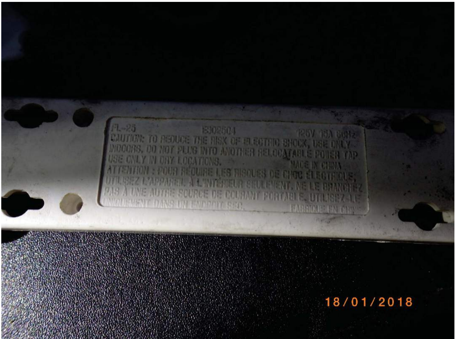
Figure 10 – This photo shows the warning on the back of the power bar indicating “DO NOT PLUG INTO ANOTHER RELOCATABLE POWER TAP. USE ONLY IN DRY LOCATIONS”.
