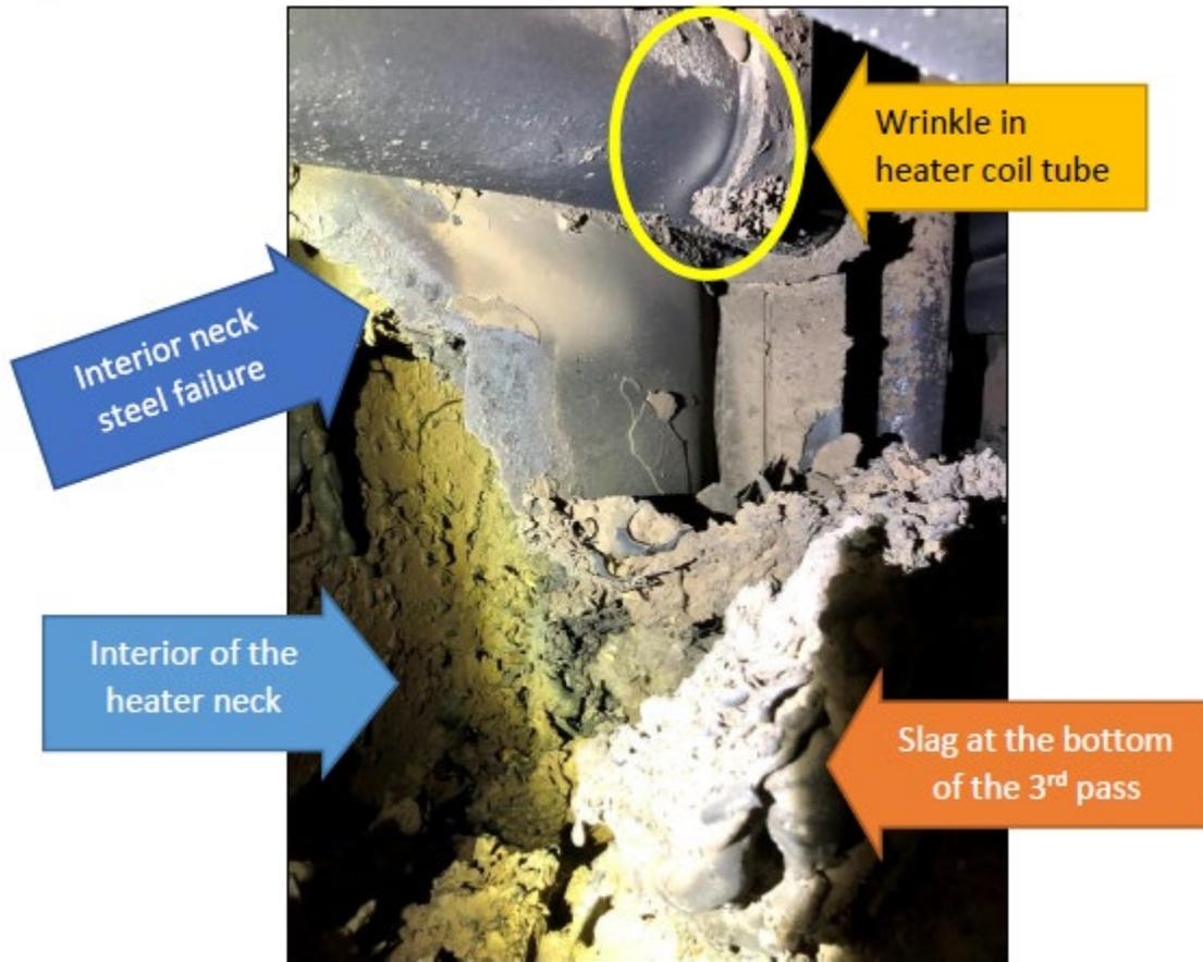
**Heater neck shell failure, slagging, and deformed coil.**
