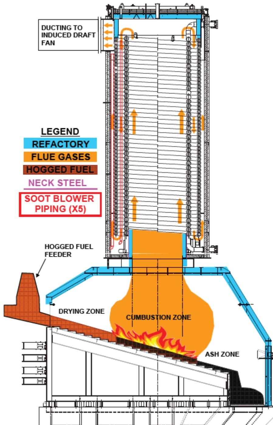
**Normal combustion of hogged fuel reciprocating step-gate furnace and path of flue gases through helical coil heat exchanger.**
