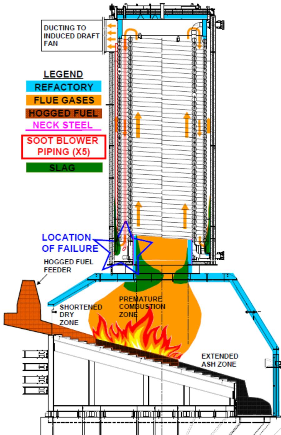
**Premature combustion of hogged fuel, slag accumulations, and location of failure.**
