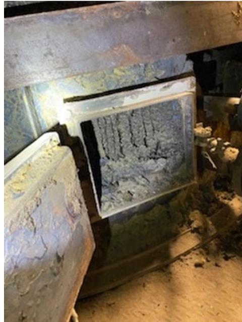
**Slag (clinker) sample and deposit of slag on outer shell.**
