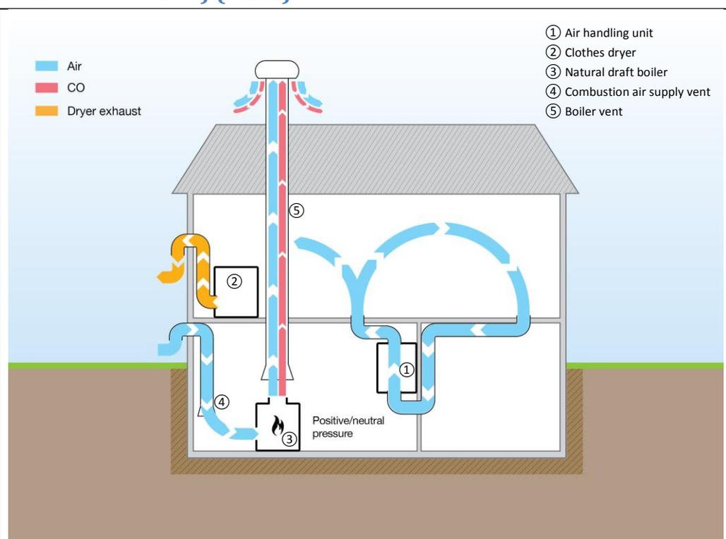
**Figure 1: Intended air flow and combustion air flow**
