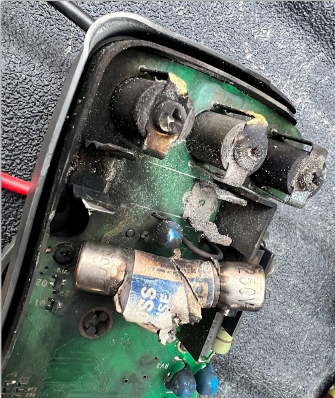
Photo 9 – Damaged multi-meter with undersized (250-volt) fuse.
