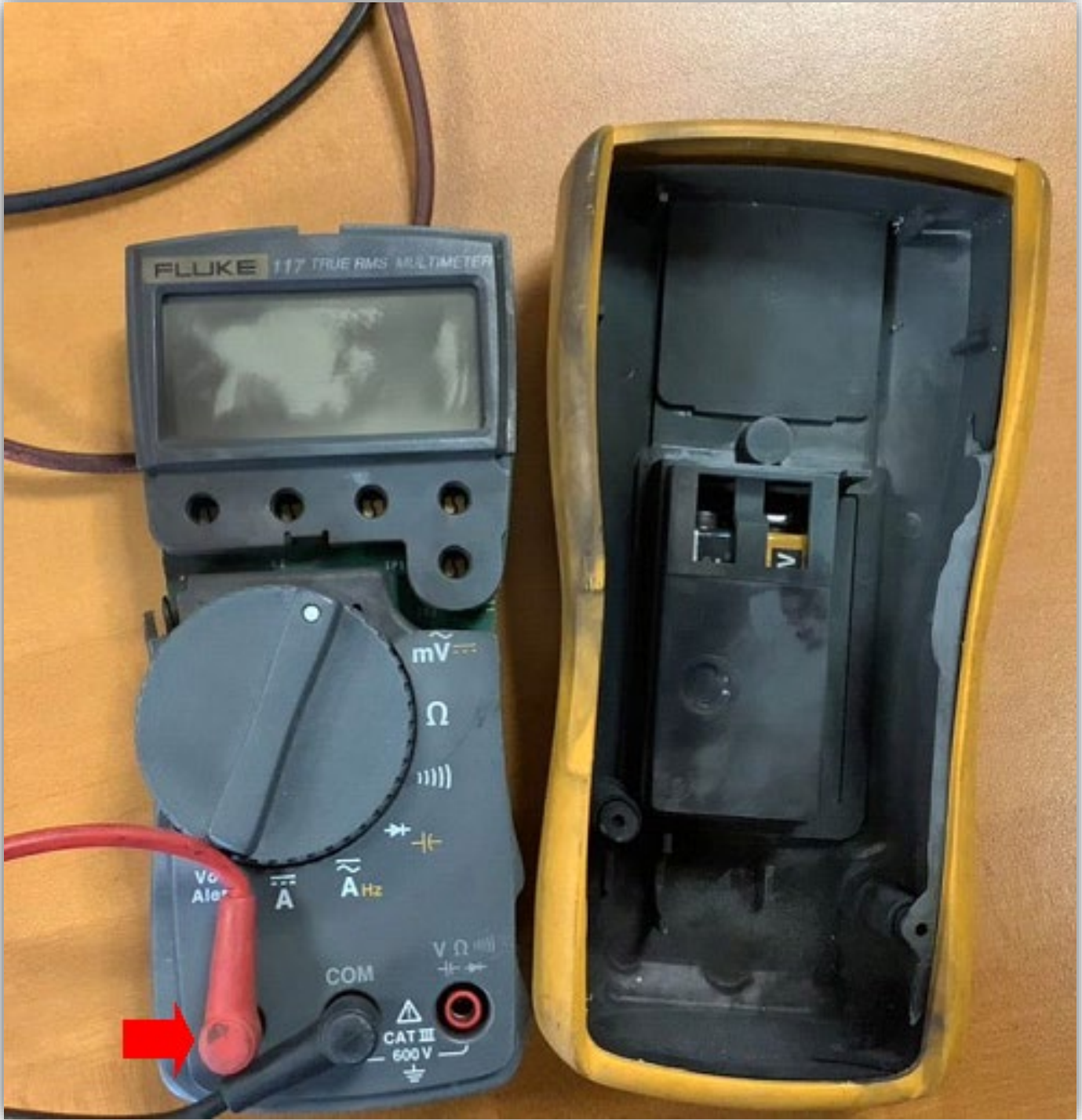
Photo 7 – [ARROW] test lead plugged into the ammeter port.
