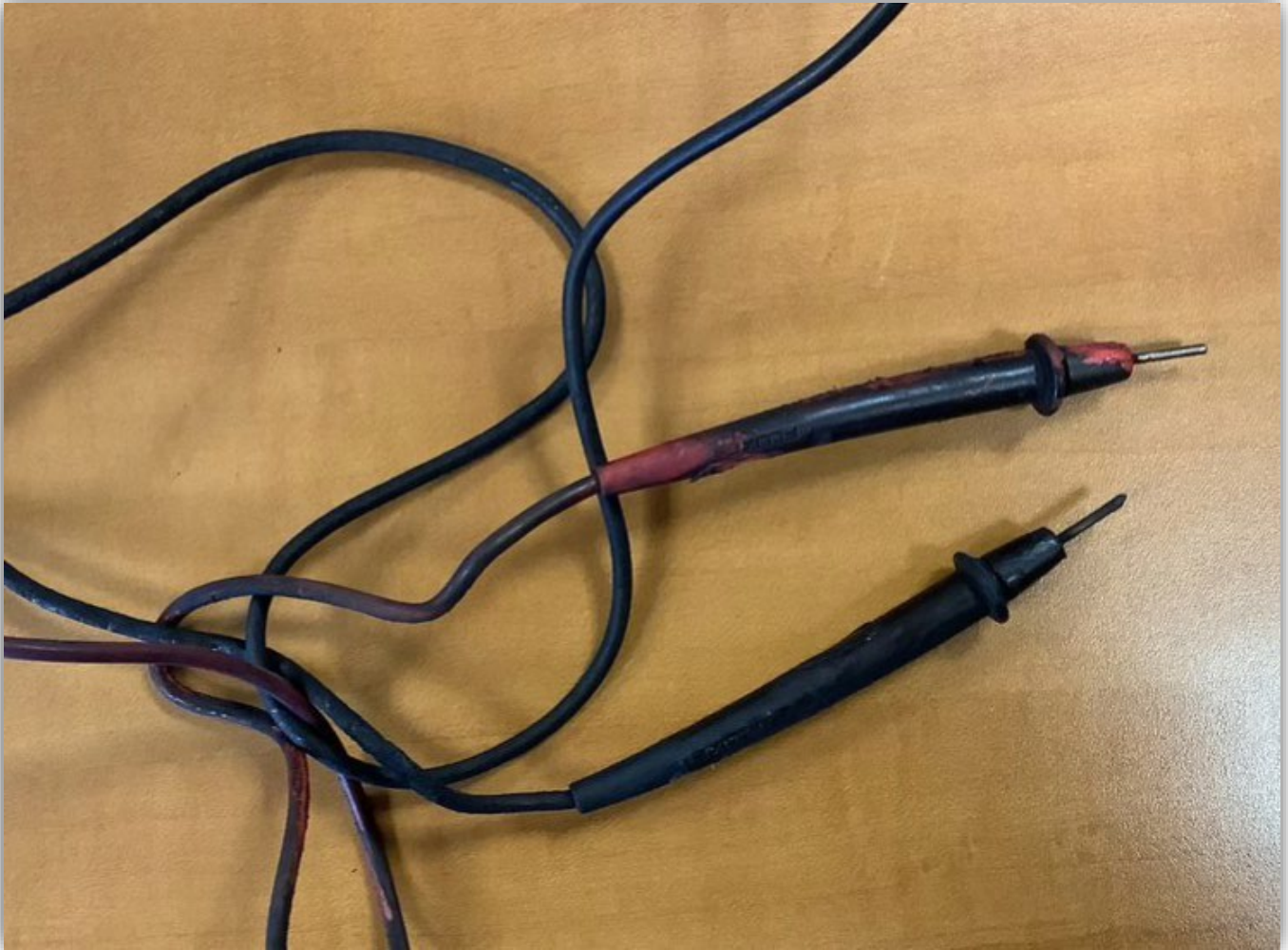
Photo 8 – Multi-meter test leads.
