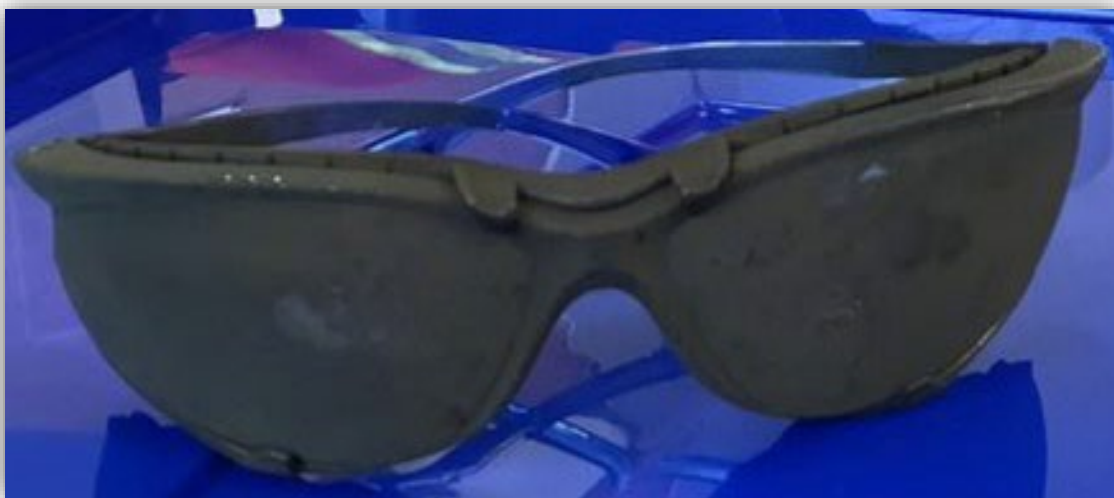
Photos 5 & 6 – Burn damage to hard hat and safety glasses.
