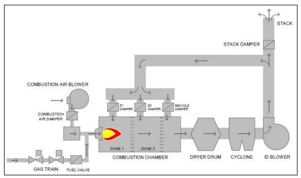
Image 1 – Diagram of the dryer system and component orientation and airflow
