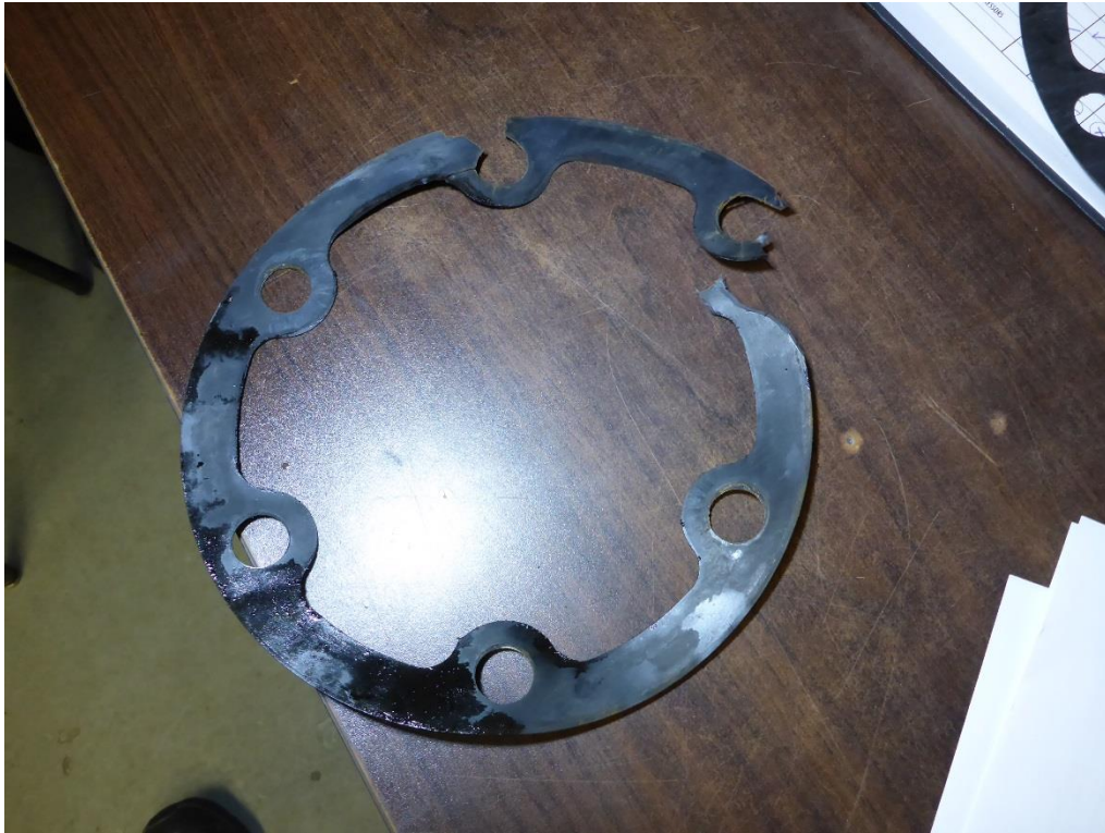
Photo 5: Photo by Boiler Safety Officer-actual gasket.
