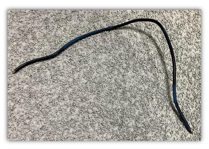
Image 5 – Closeup of the jumper wire used to short across the energized line side terminals.
