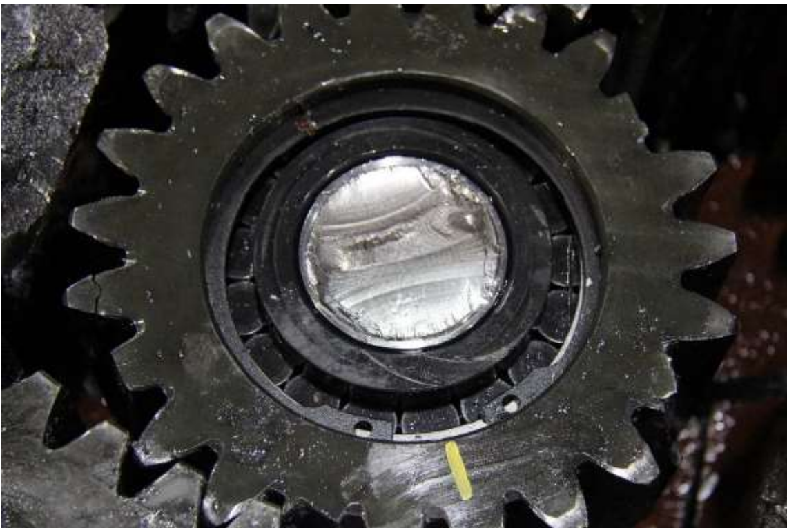
Photo 8: Planetary gear post fracture surface shows reverse bending fatigue cracking, [Lab report].
