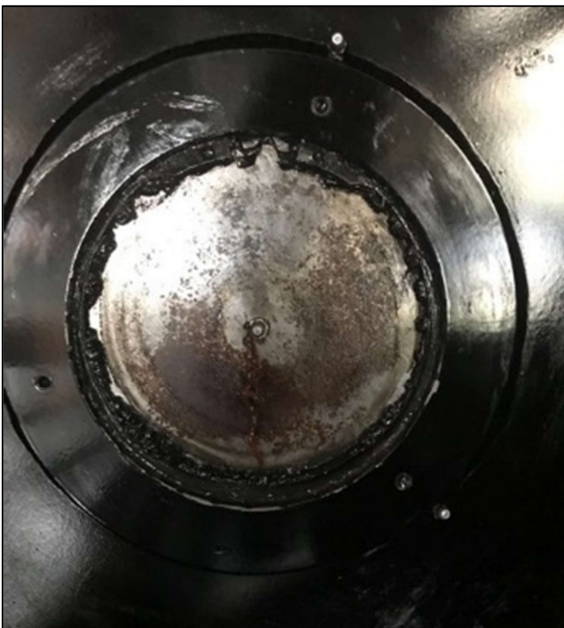
Photo 4: Initial inspection, snap ring pushed out of position by gearbox end plate, due to axial load.
