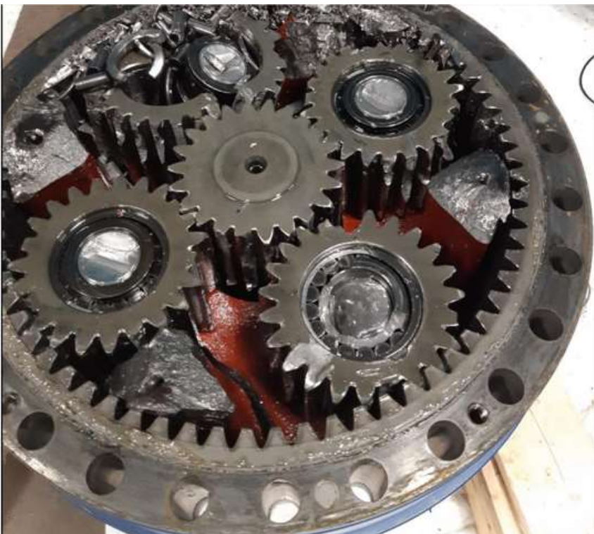
Photo 6: Gearbox Stage 3 Planetary gear set damage, complete fracture of all four posts, [Lab report].
