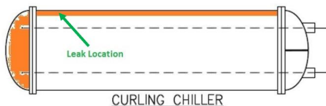
Figure 11: Representation of the areas that were considered near saturation for the release scenario (the drawing is not to scale). The arrow indicates the approximate location of the tube leak.
