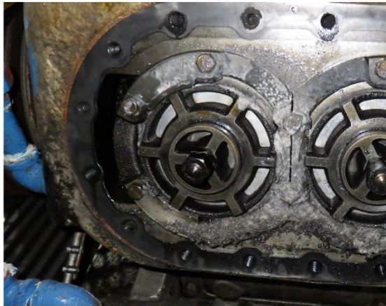
Figure 5: CaCl 2 Evidence in Compressor Cylinder Heads
