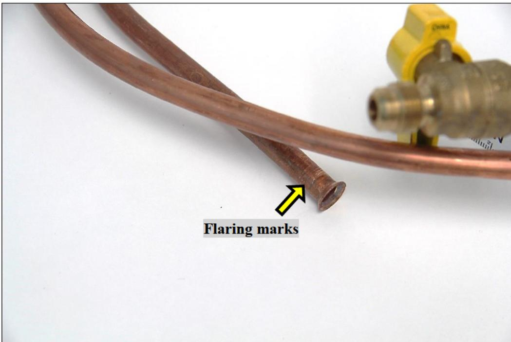
**Figure 10** The riser side of whip #228. The riser side is straight.
