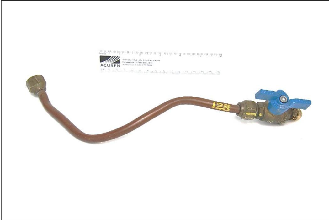
**Figure 1** General condition of whip #128 as received.
