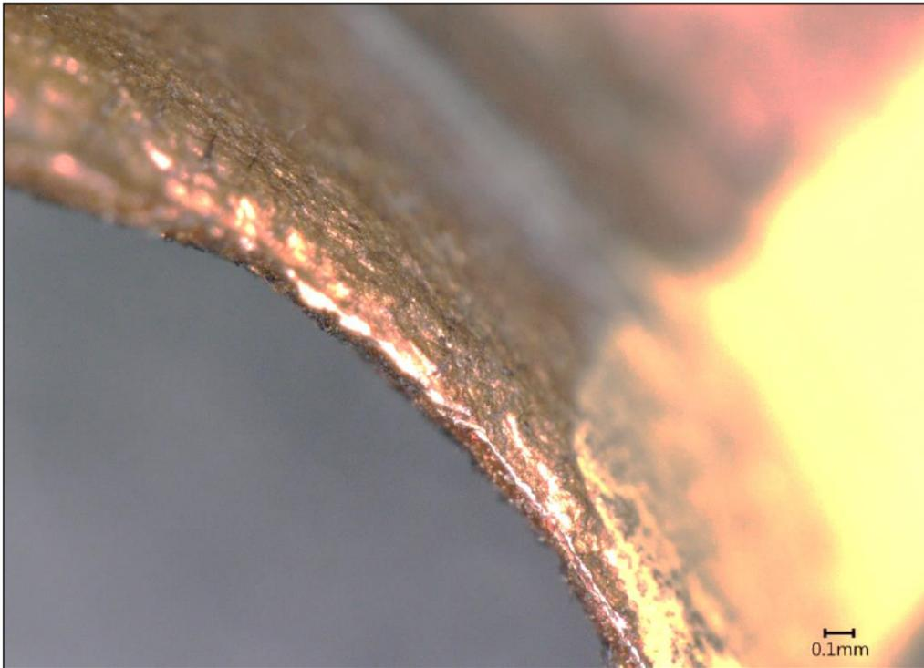
**Figure 24** The fracture origin of the whip #328 fracture surface. The wall of the pipe exhibited necking.
