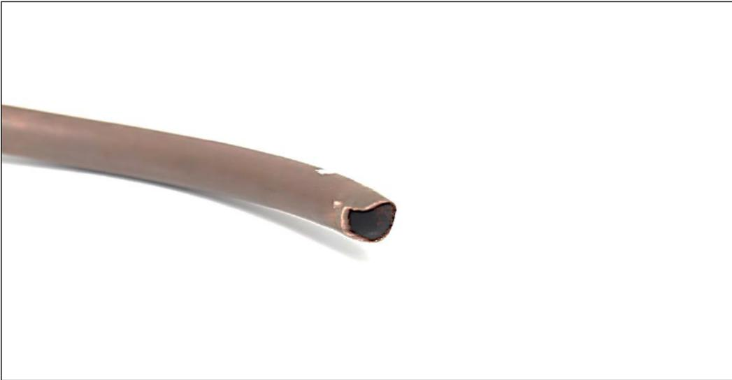
**Figure 15** The fracture surface of the rise side of whip #328.
