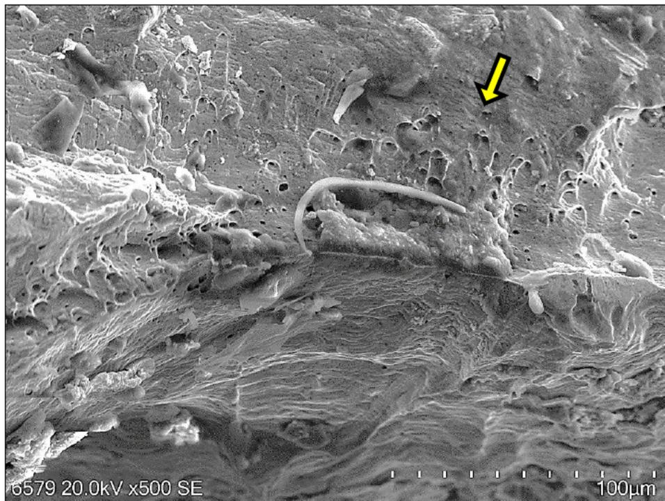
**Figure 29** SEM image of the fracture surface, as indicated in Figure 21. Elongated dimples indicating ductile fracture are notable. The arrow shows the fracture propagation direction.
