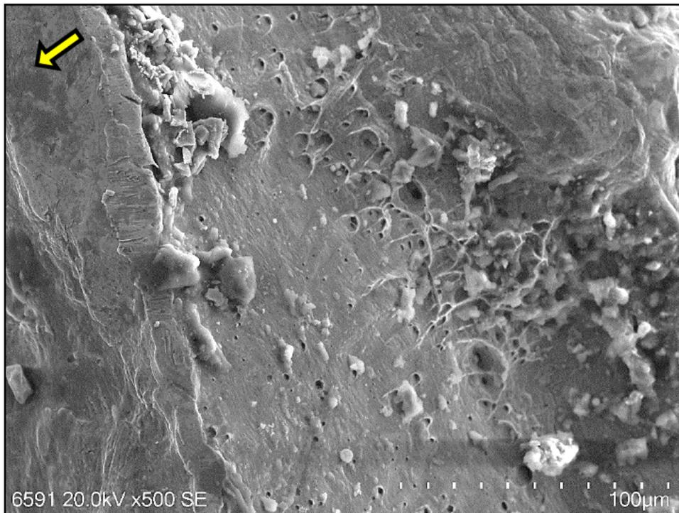
**Figure 32** SEM image of the fracture surface, as indicated in Figure 21. Elongated dimples indicating ductile fracture are notable. The arrow shows the fracture propagation direction.
