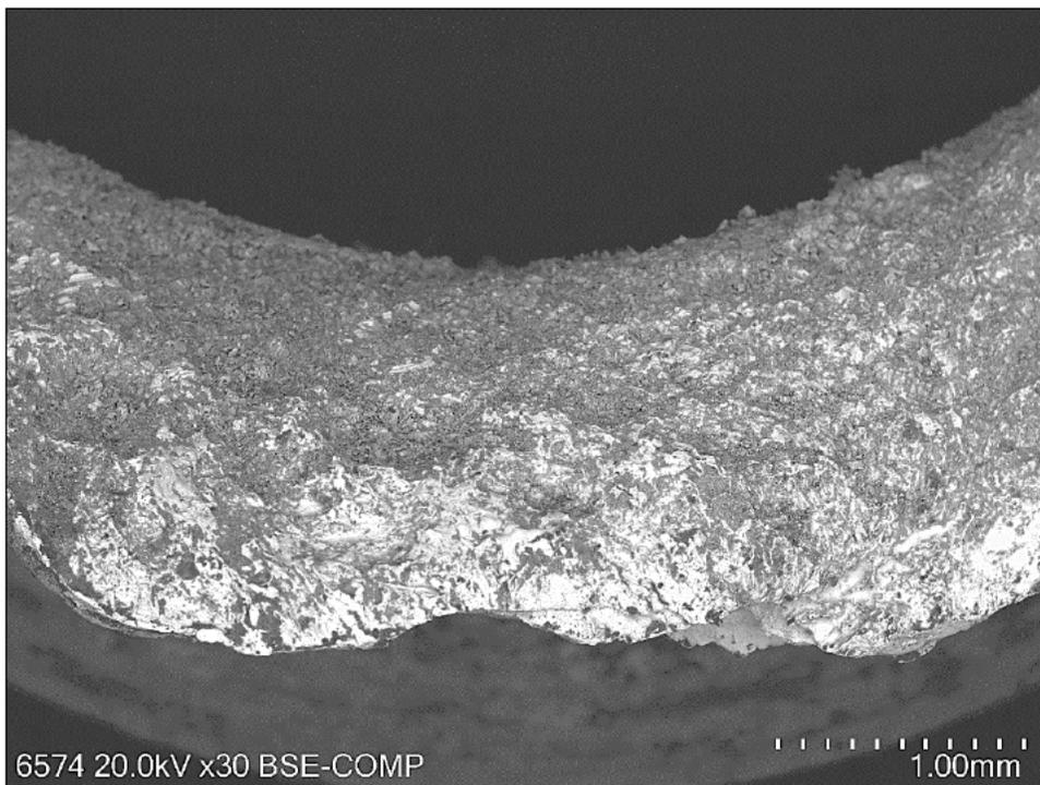
**Figure 27** SEM image of the fracture surface, as indicated in Figure 21.
