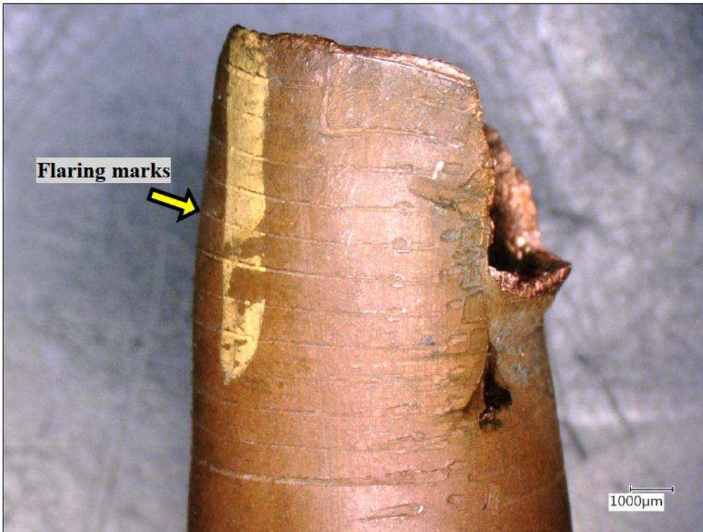
**Figure 26** Matching fracture surface of whip #328 fracture surface. The pipe profile shows that it was under bending stress.
