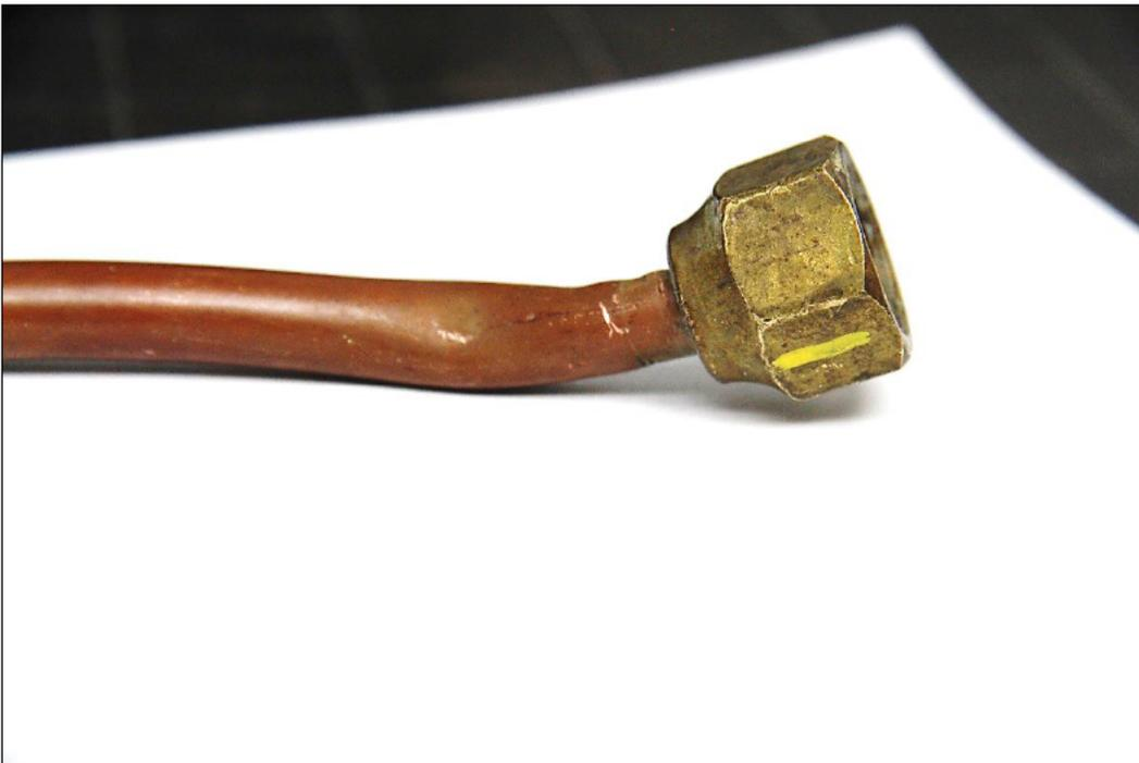
**Figure 6** Whip #128 was bent at the riser side.
