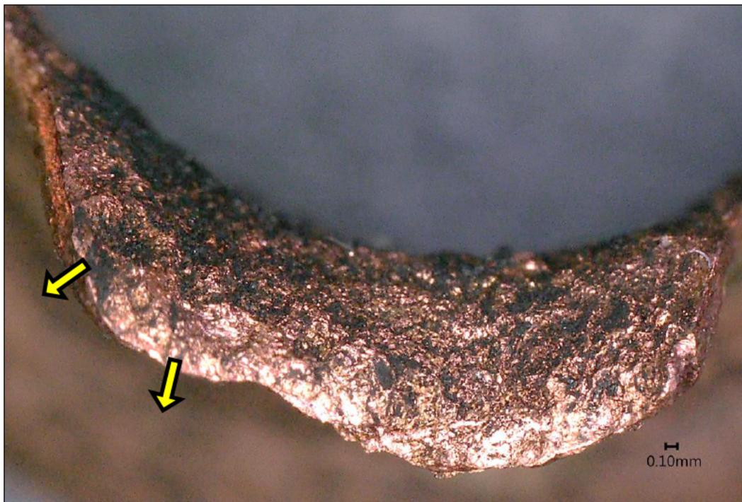
**Figure 22** Final fracture zone of whip #328.
