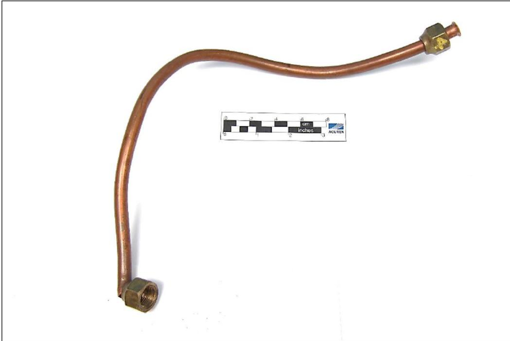
**Figure 17** General view of whip #428 as received. The valve side is intact, and the riser side is fractured.
