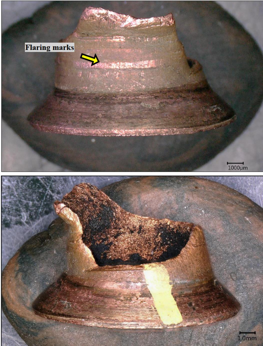
**Figure 23** The fracture profile of the copper pipe indicated that the pipe was bent.
