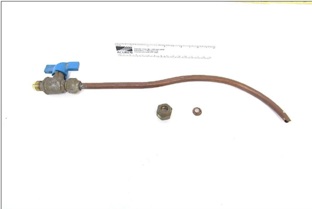
**Figure 11** General condition of whip #328 as received. The riser side was fractured. The fracture fragments are shown.
