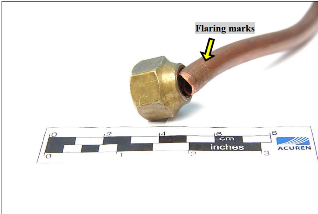
**Figure 19** The position of the fitting indicated that bending forces were applied to the riser side of whip #428.
