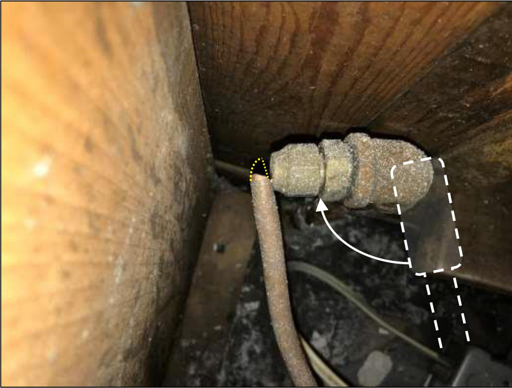
Photo 7: Copper gas whip in suite #4 was bent ~90 degrees and partially fractured (yellow line) then fully fractured due to the explosion, as shown above. The original position of the elbow fitting is estimated by the white dashed line.
