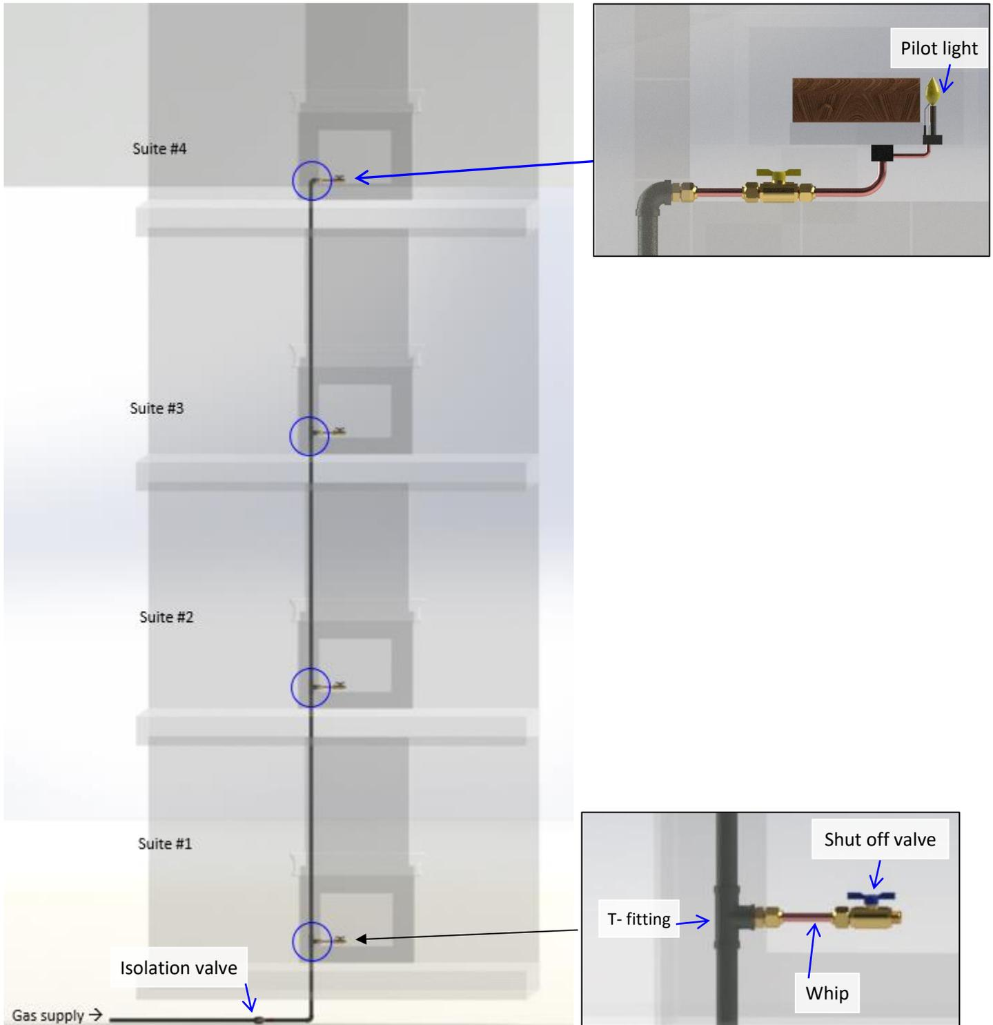
Figure 1: Schematic diagram of the gas piping system. Horizontal gas pipe in parkade connects to vertical gas riser that extends to all four floors. A T-fitting (blue circle) in the riser at each floor connects to a copper whip that supplies gas to the fireplaces.
