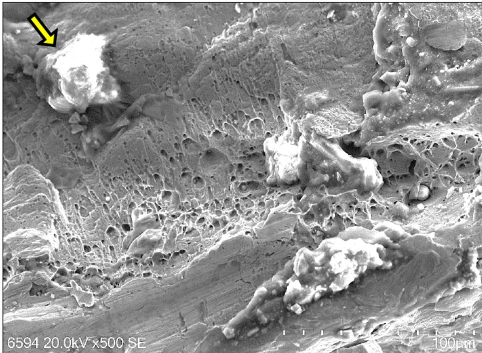
**Figure 30** SEM image of the fracture surface, as indicated in Figure 21. Elongated dimples indicating ductile fracture are notable. The arrow shows the fracture propagation direction.
