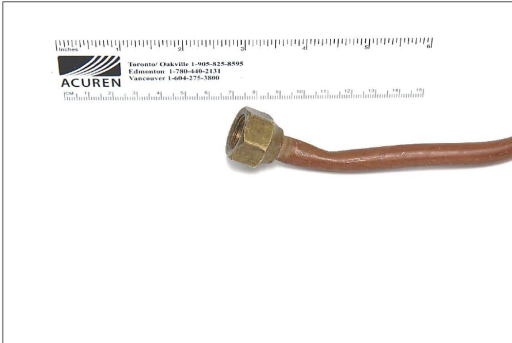
**Figure 7** Whip #128 was bent at the riser side.
