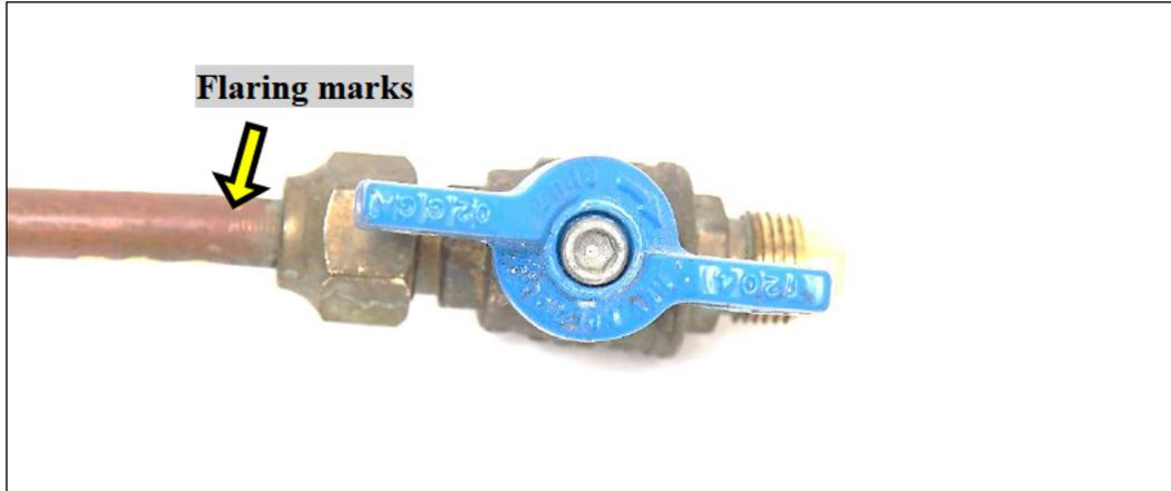
**Figure 13** The valve side of whip #328.
