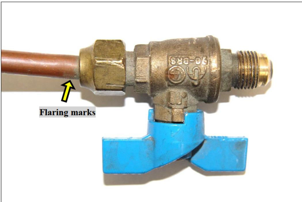
**Figure 4** The valve side of whip #128.
