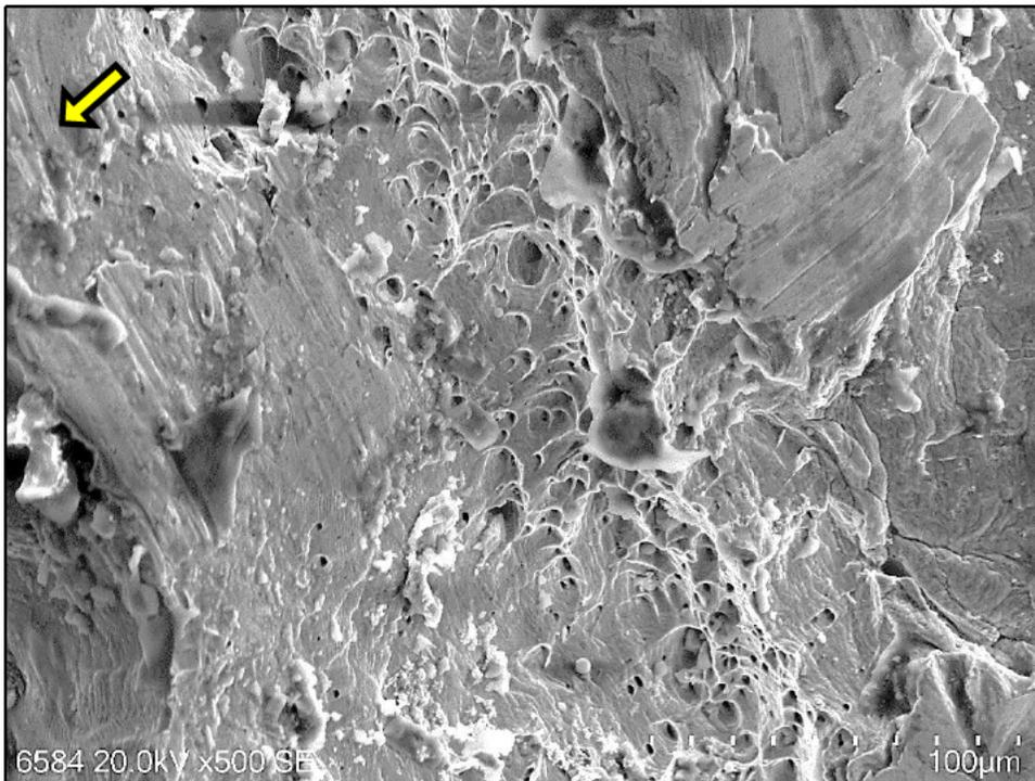
**Figure 31** SEM image of the fracture surface, as indicated in Figure 21. Elongated dimples indicating ductile fracture are notable. The arrow shows the fracture propagation direction.
