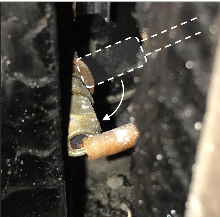
Photo 6: Copper gas whip in suite #3 was bent ~90 degrees and completely fractured. The leaking gas ignited, burning the wood structure. The original position of the T-fitting is estimated by the white dashed line in the photo.
