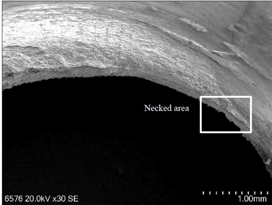
**Figure 28** SEM image of the fracture surface, as indicated in Figure 21. Pipe wall experienced necking.
