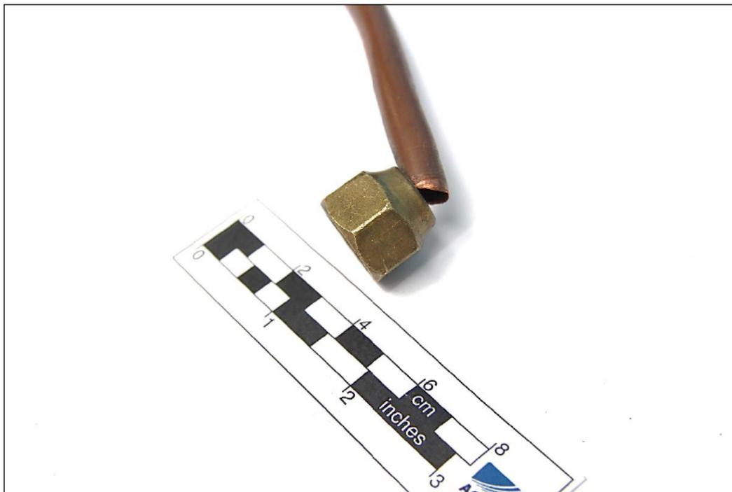
**Figure 20** The position of the fitting indicated that bending loads were applied to the riser side of whip #428.
