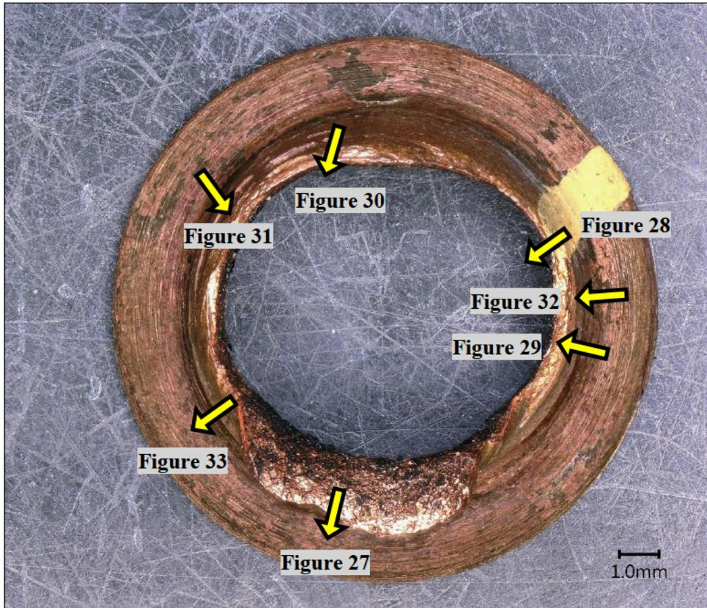
**Figure 21** Fracture surface of the riser side of whip #328. Arrows show the fracture propagation direction.
