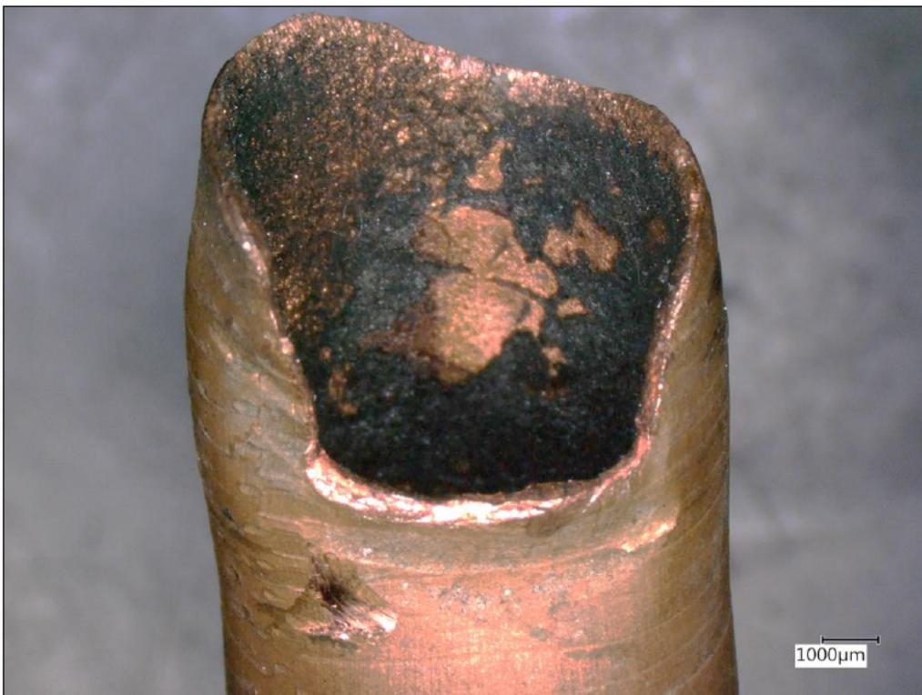
**Figure 25** Matching fracture surface of whip #328 fracture surface. Black deposits were noted on the pipe ID. The copper pipe was bent toward the final fracture zone.
