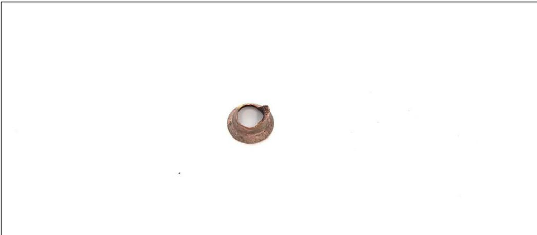
**Figure 16** The fracture surface of the rise side of whip #328.
