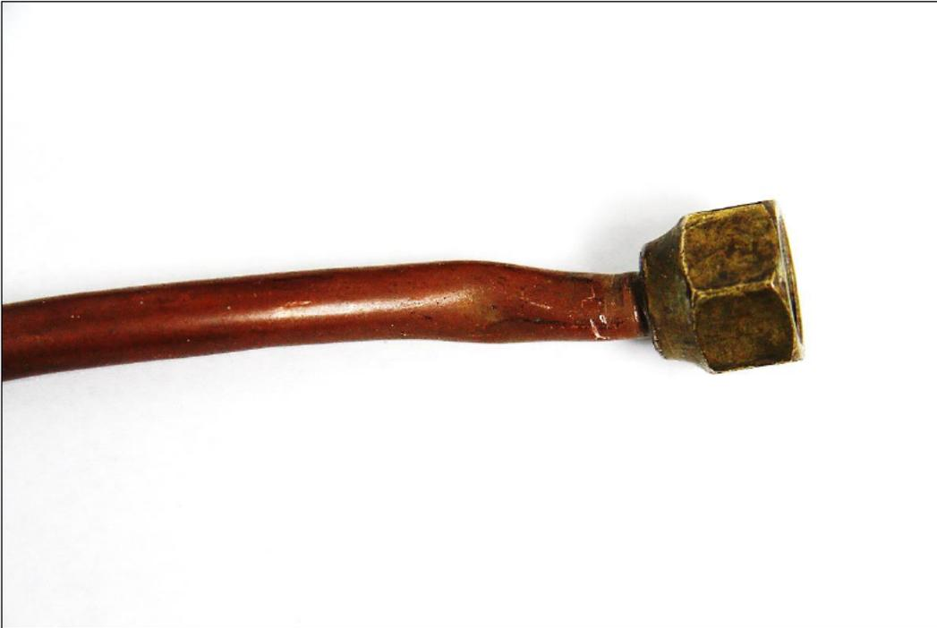
**Figure 5** The riser side of whip #128 was bent.
