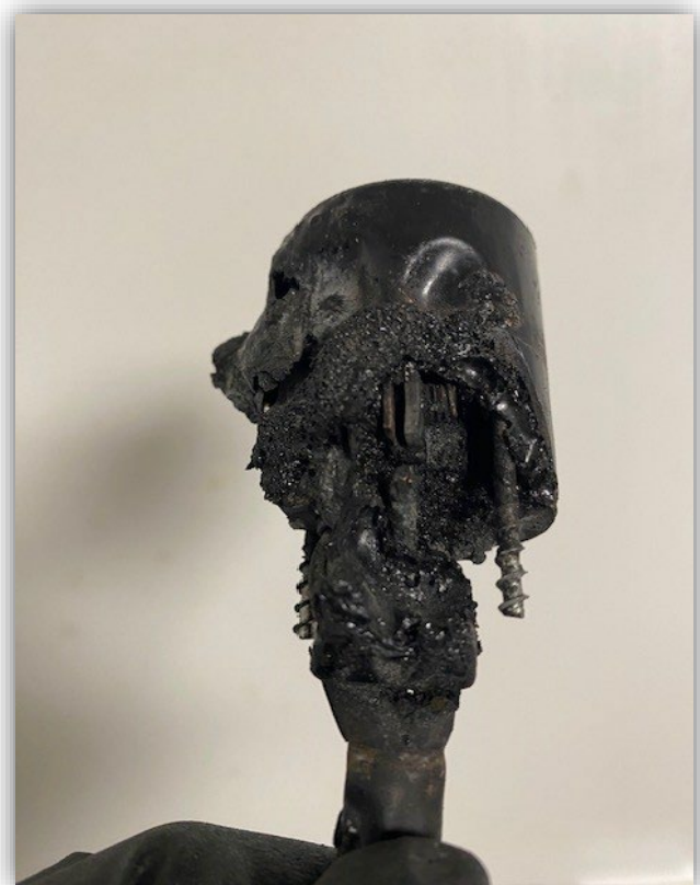
Image 7 - Localized melting inside the receptacle-end.
