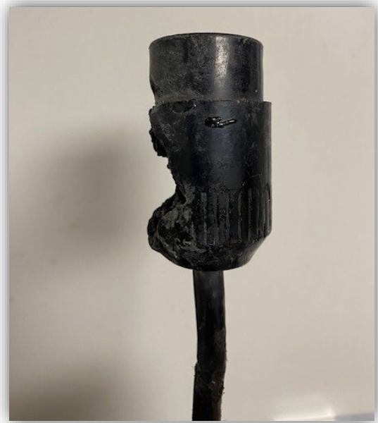
Image 5 - Localized melting of receptacle-end.
