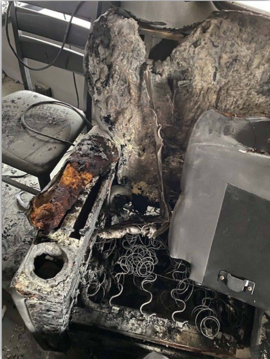
Image 2 - Upholstered couch, which appears to have been the point of origine for the fire.
