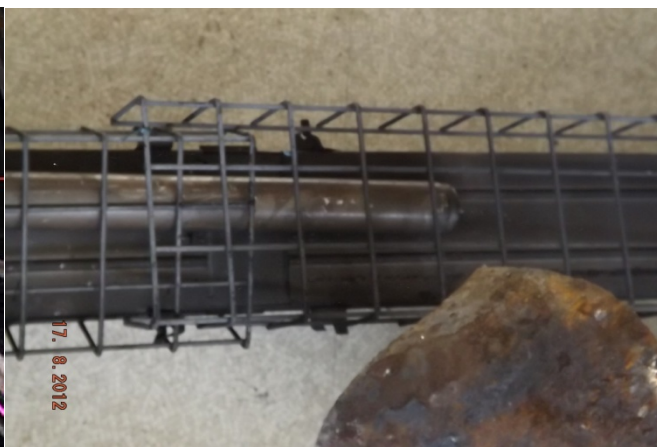
Photograph 15: Fluorescent light assembly found within the area of origin.
