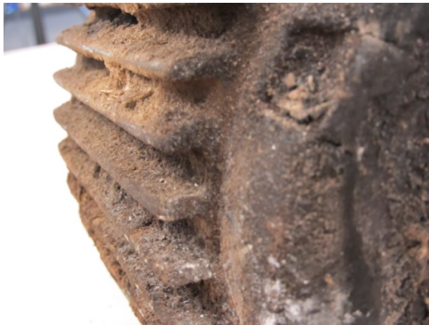
Photograph 10: P6 motor – view of side cooling fins -wood dust contamination.
