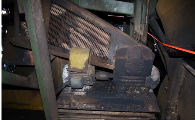
Photograph 6: P6 motor assembly, shaft and guard, gear reducer and chain guard as found. Note that the yellow shaft guard was installed over the shaft connecting the motor and reducer.
