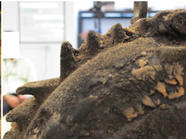
Photograph 9: P6 motor – end view top quarter – wood dust found contaminating cooling fins.
