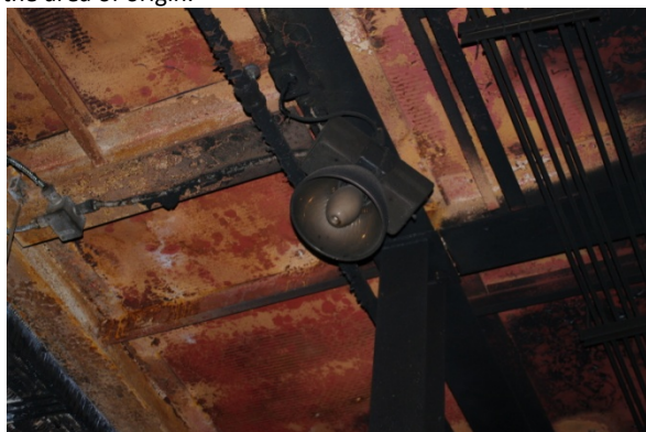
Photograph 14: Fluorescent light assembly found within the area of origin.
