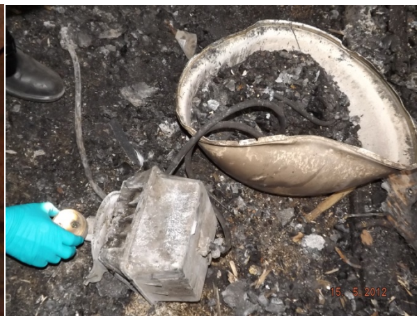
Photograph 13: High bay light assembly found within the area of origin with metal halide bulb.
