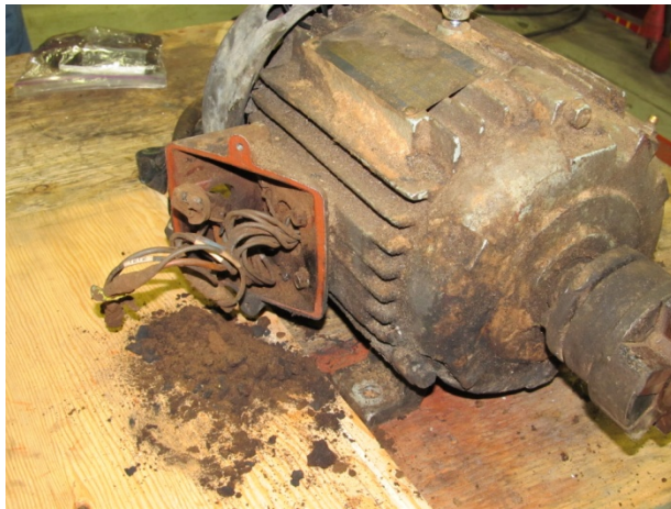
Photograph 8: P6 motor – wood dust found within junction box.
