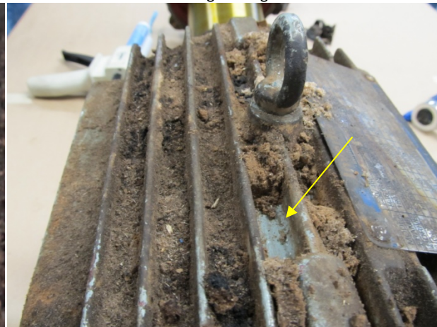
Photograph 11: P6 motor – top view showing depth of cooling fin contamination on scraped portion.
