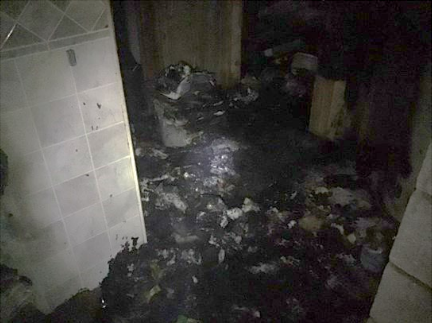
Area around base of domestic hot water tank – burnt toilet paper, tissue, paper towels.
