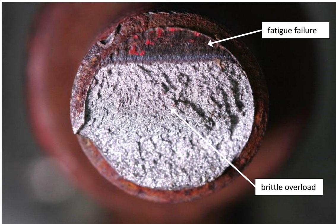
**Figure 6:** Fractured Surface of Eyebolt Threaded Shaft.
