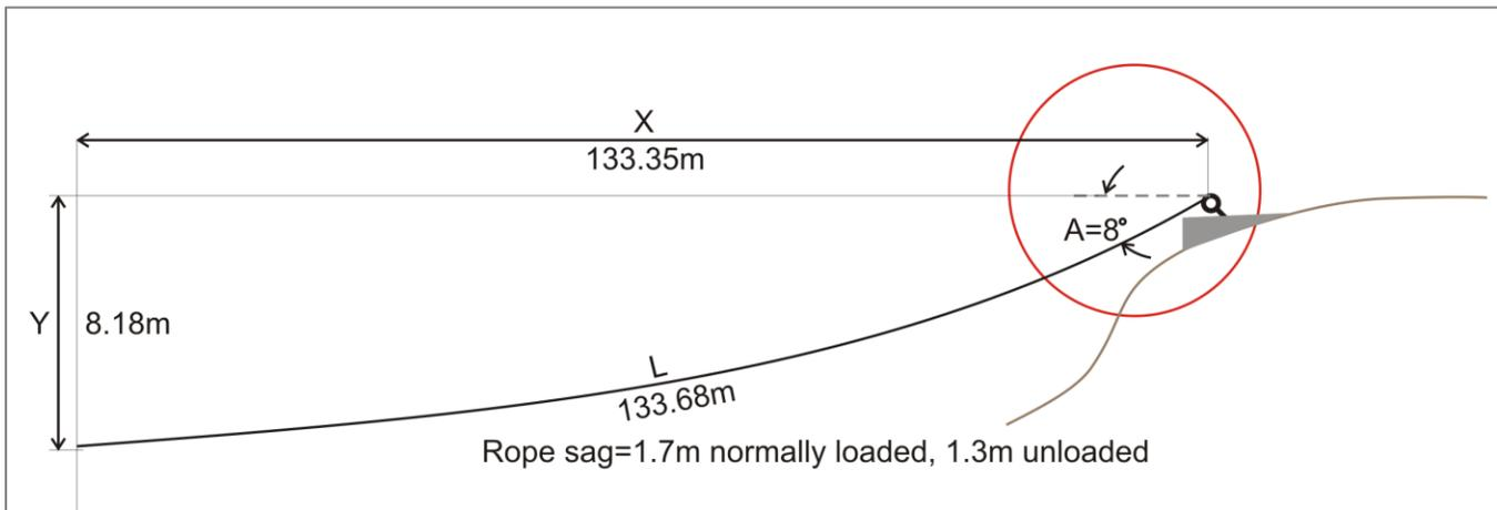
**Figure 3:** Profile of Zipline as Measured Following Incident
