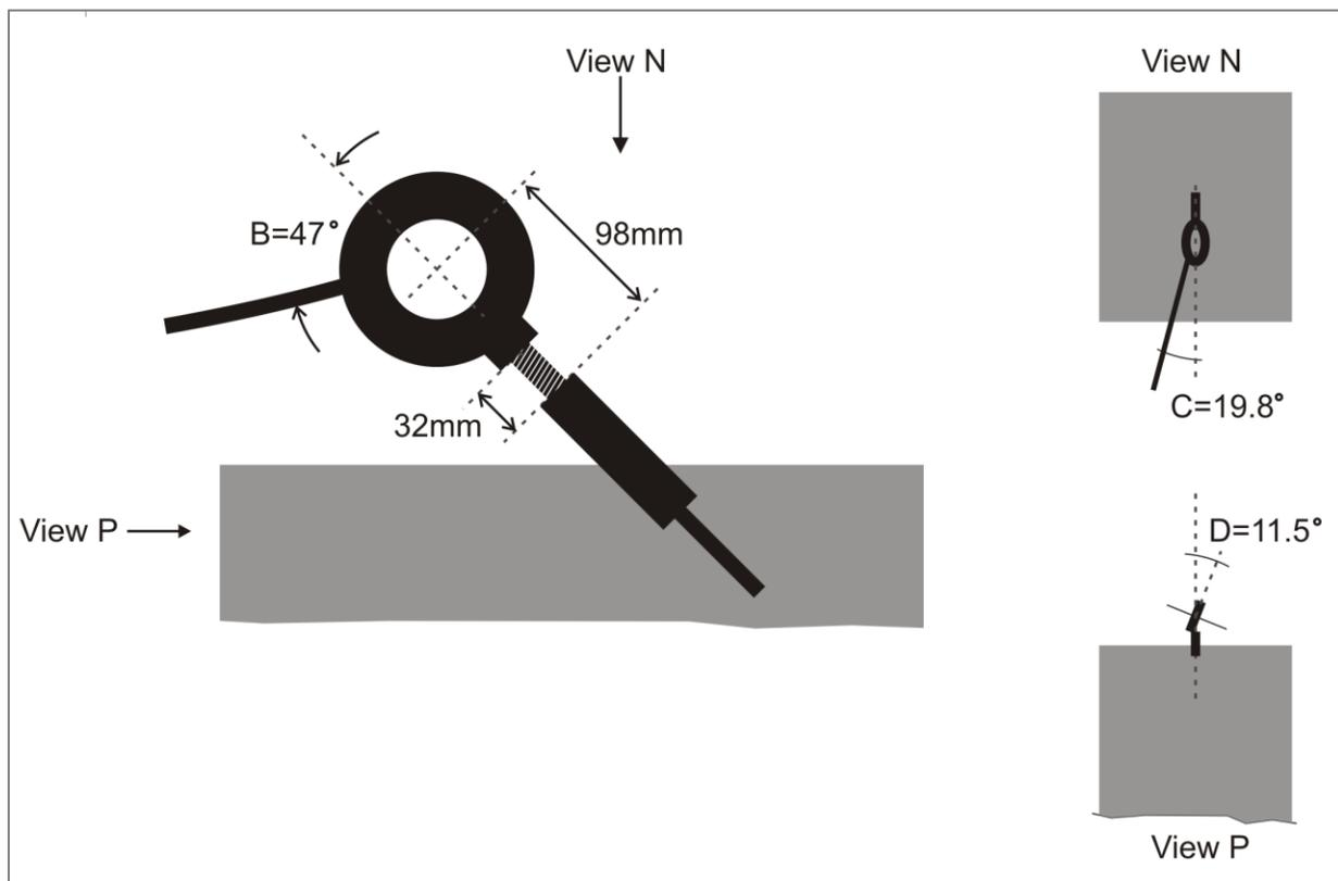
**Figure 4:** Orientation of the Eyebolt and Anchor relative to Zipline Cable
