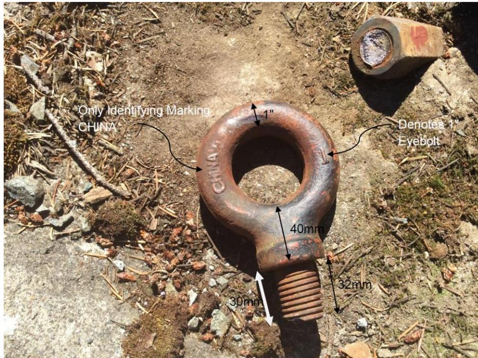
**Figure 5:** Fractured Eyebolt. Image shows approximately 30mm of threads were protruding from the anchor.
