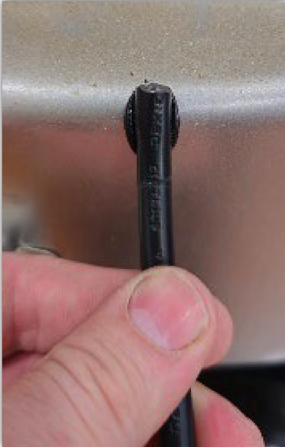
Image 2 - Burnt end of the adjacent kitchen counter appliance.
