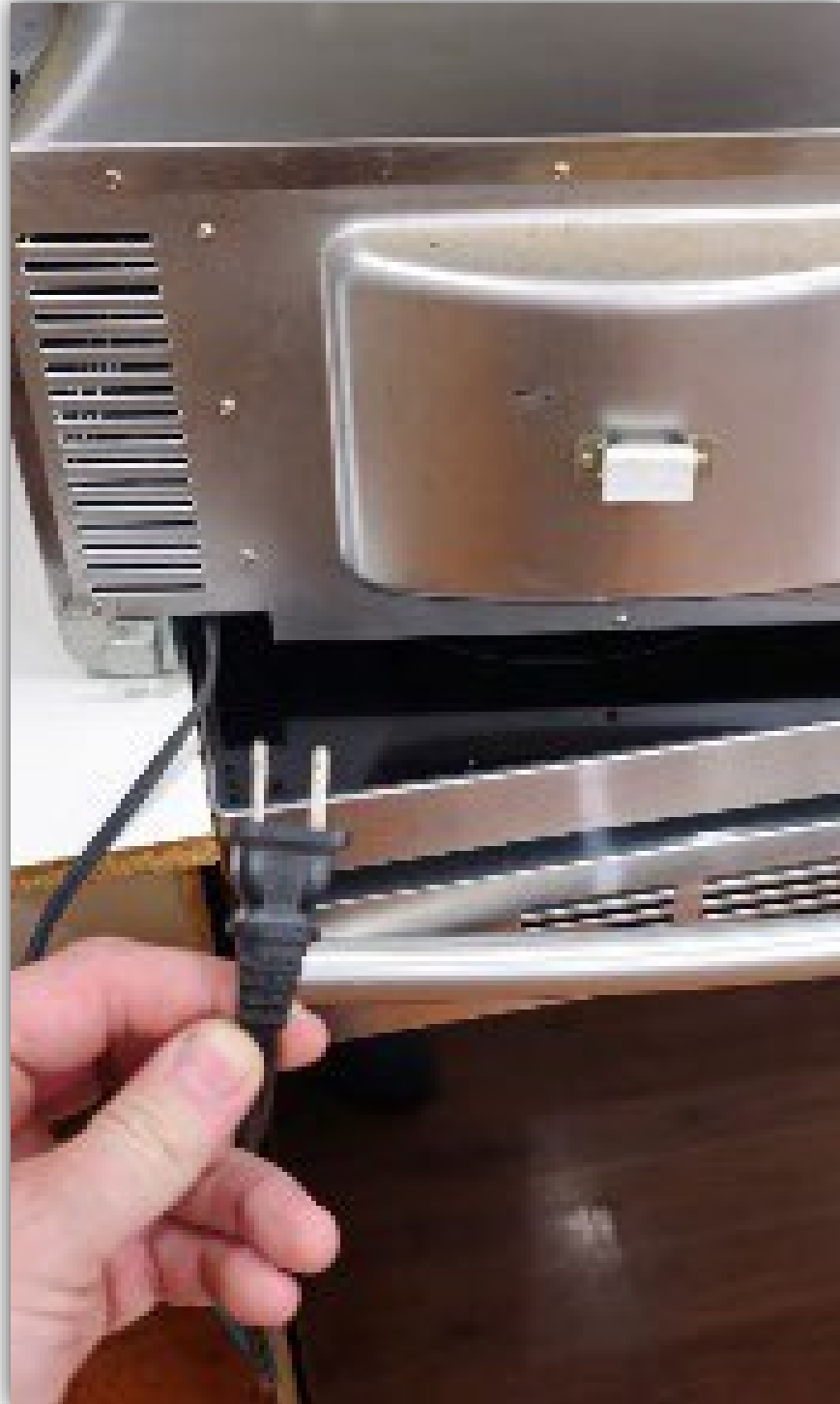
Image 3 - Metal enclosed toaster oven with only a two-prong attachment cord.
