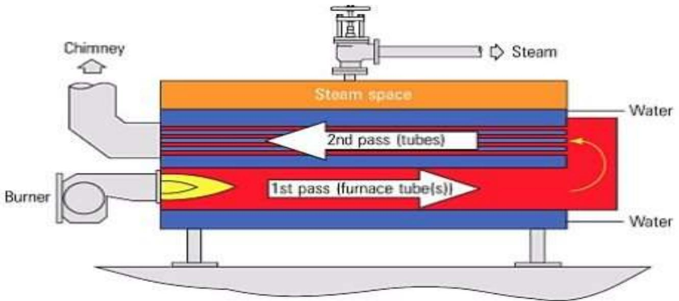
Diagram 1: A fire tube boiler
