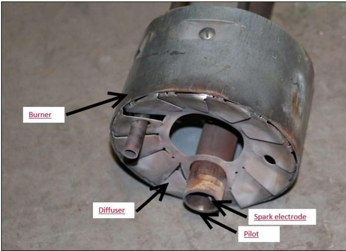
Photo 3: Power burner and its components.
