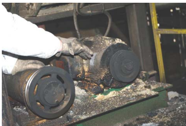
Photograph 9: Wood dust accumulation around conveyor motor labeled 8R-26.
