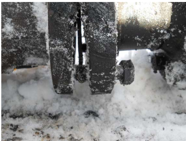
Photograph C1: Broken bolt at valve flange to heat exchanger
