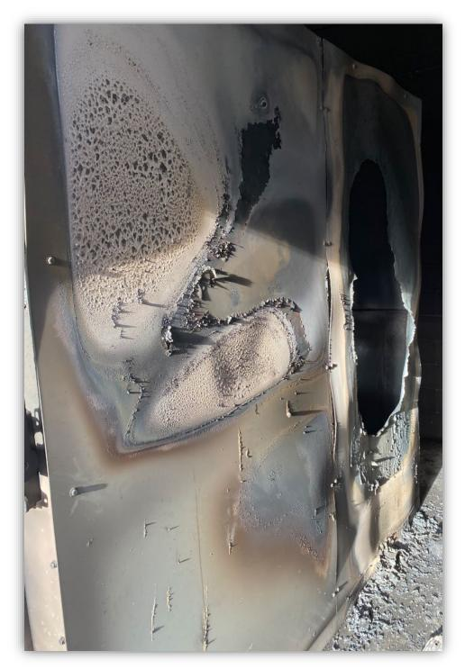
Photo 10 - End section of Unit #6 chip mill where majority of damage occurred, back side of unit has large hole approx. 2'w x6' high blown through it.
