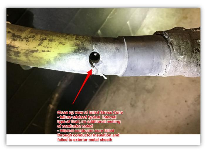
Photo 15 - Close-up photo of failure point of cable within stress cone. Interior conductor is noted to be blown out from the interior outwards.
