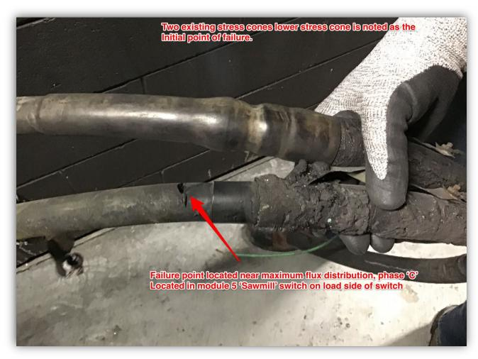
Photo 14 - Two of the stress cones cut out from Modules #5 with failed cable noting location of fault within the stress cone.
