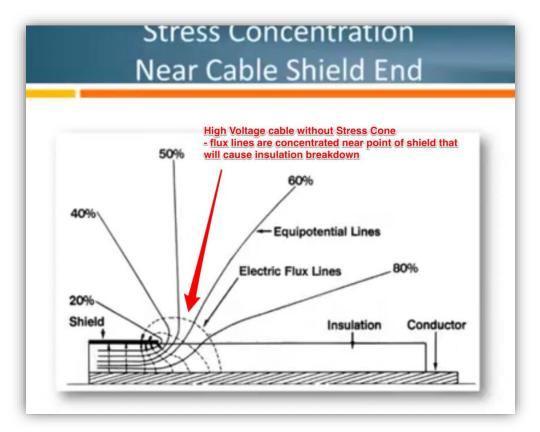
Photo 16 - Shows stress cones are installed and what they do to providing a long-lasting operation of cable terminations. Upper shows how the lines of flux are spread out to dissipate and minimize the degradation of the cable insulation. The lower diagram provides 'how' the lines of flux are contained within a short space that will cause a quick failure of the cable insulation due to heating.
