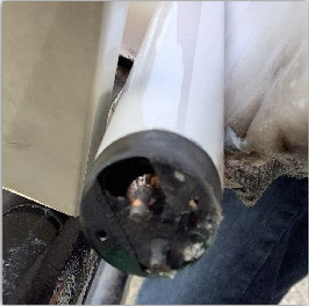
Image 2 - Burnt end of the fluorescent tube.
