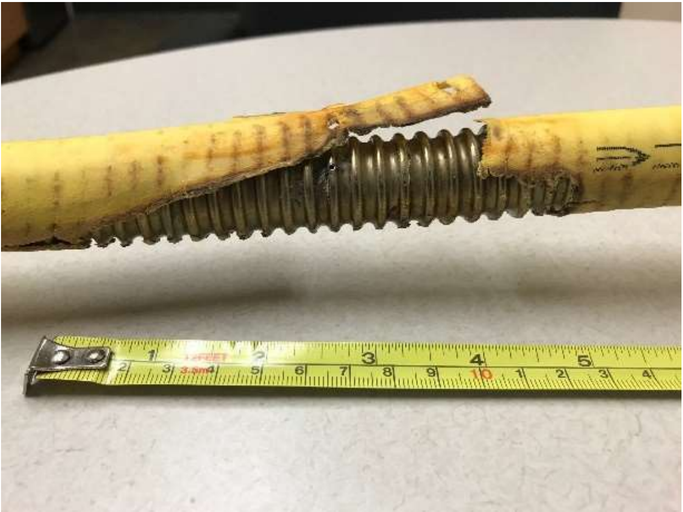
Image 2 - Damaged section of CSST
