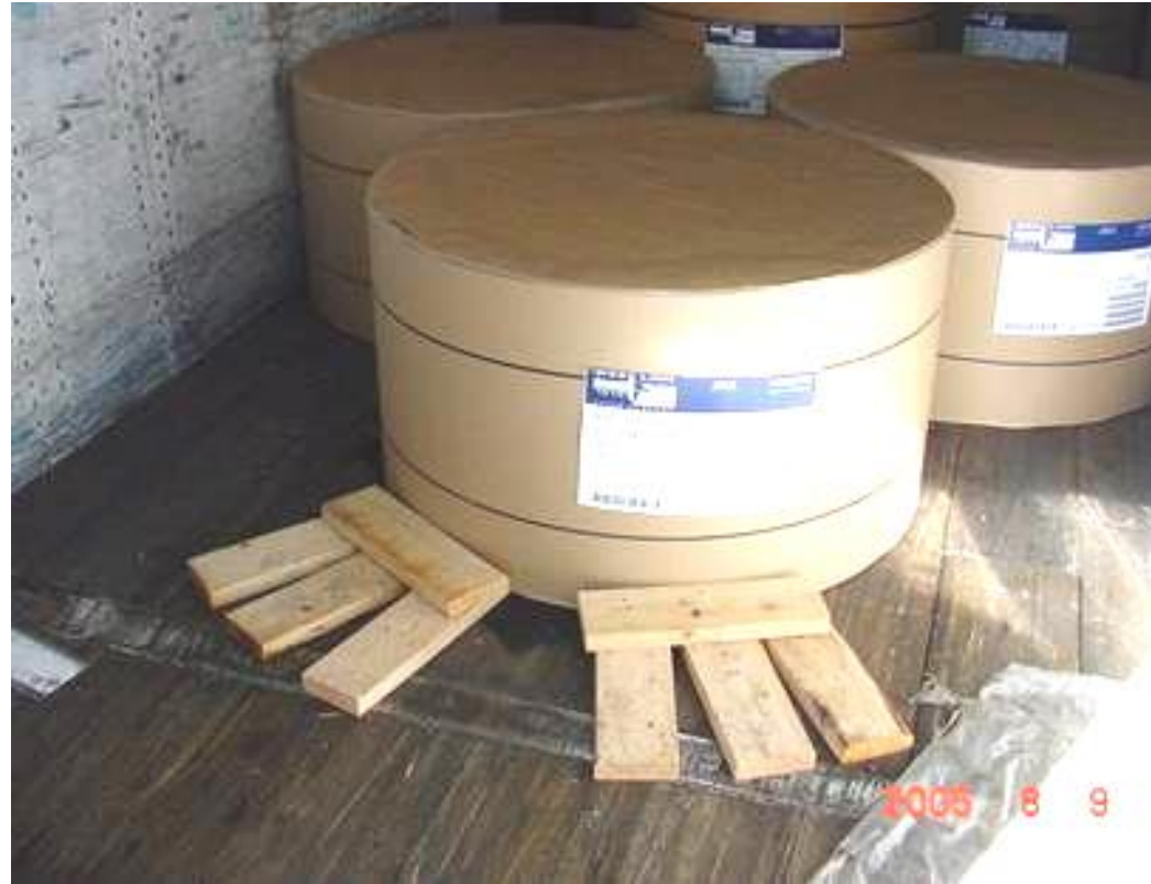
LAMINATED 2\"X6\"X24\" E-BRACES: 2 PER REAR POINT ROLL
